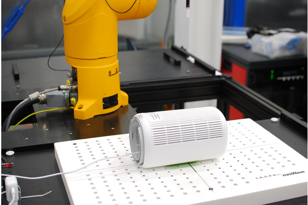
Figure C-3 Near Field Power Density Test Setup Photo – Back Side at 200mm
