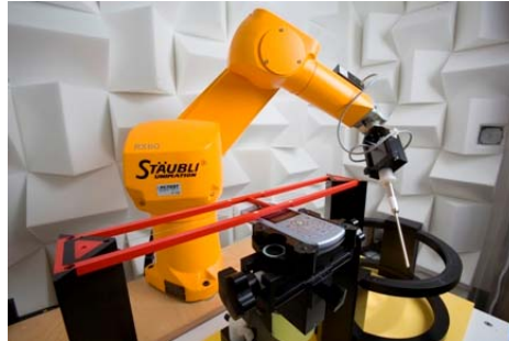
Figure 4-3 SPEAG Robotic System
