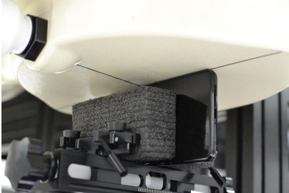
SAR Test Setup Photo 9 – Right Side at 0 mm
