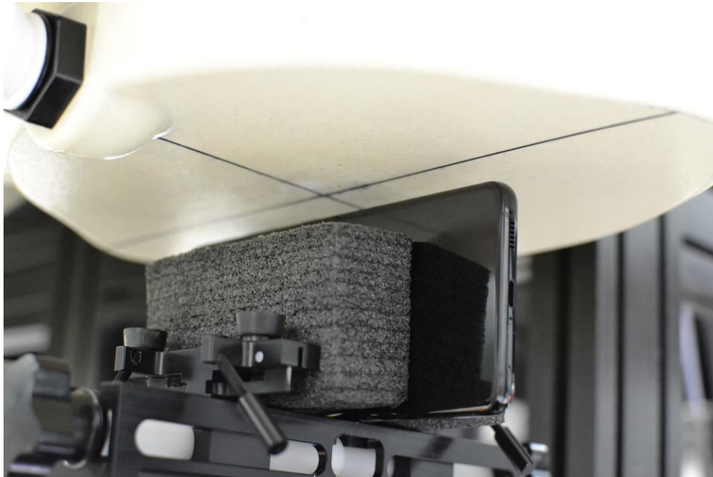
SAR Test Setup Photo 8 – Right Side at 10 mm
