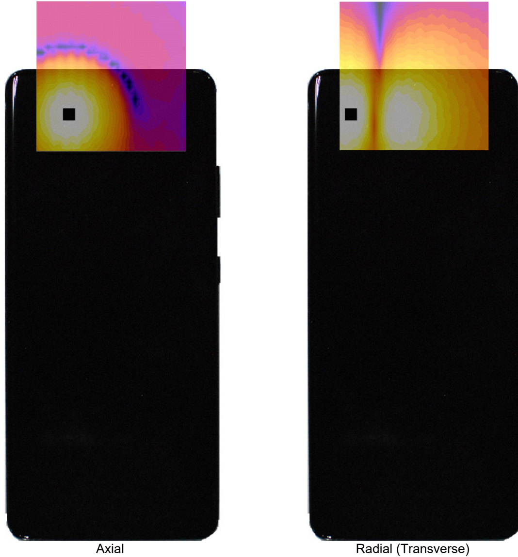
Figure 13-3 T-Coil Scan Overlay Magnetic Field Distributions
