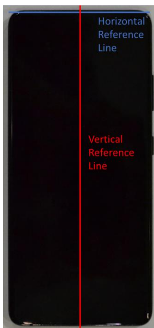
SAR Test Setup Photo 12 – Vertical and Horizontal Reference Lines
