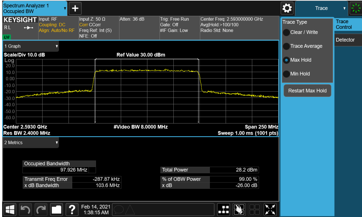
Plot 7-5. Occupied Bandwidth Plot (NR Band n41 - 100MHz 256-QAM - Full RB)
