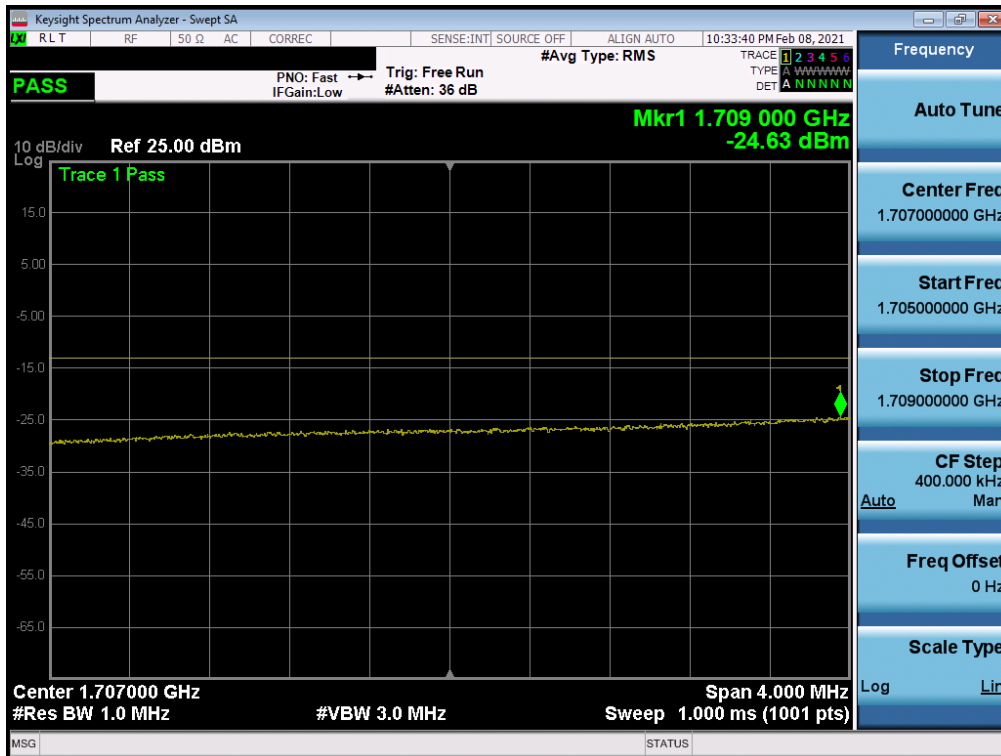
Plot 7-39. Lower Extended Band Edge Plot (LTE Band 66 - 15MHz QPSK – Full RB)
