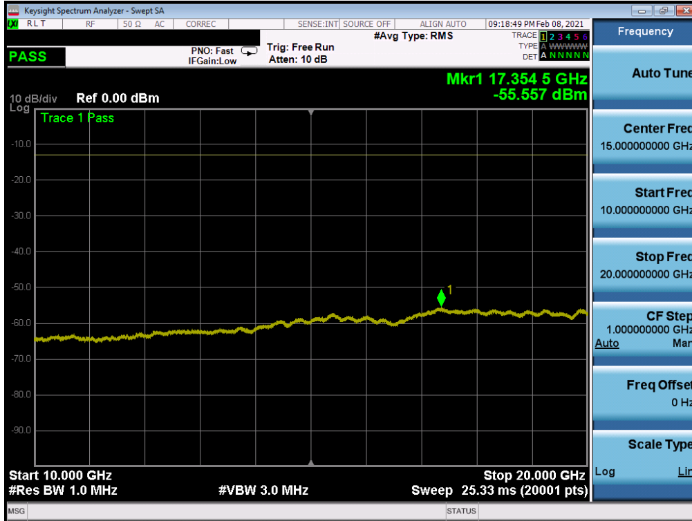
Plot 7-27. Conducted Spurious Plot (LTE Band 66 - 20MHz QPSK - RB Size 1, RB Offset 0 - Low Channel)
