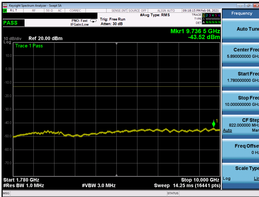
Plot 7-26. Conducted Spurious Plot (LTE Band 66 - 20MHz QPSK - RB Size 1, RB Offset 0 - Low Channel)
