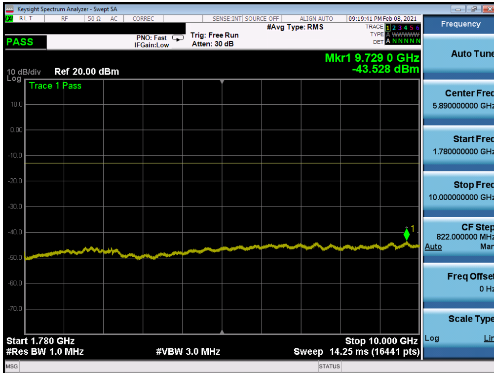
Plot 7-32. Conducted Spurious Plot (LTE Band 66 - 20MHz QPSK - RB Size 1, RB Offset 0 - High Channel)
