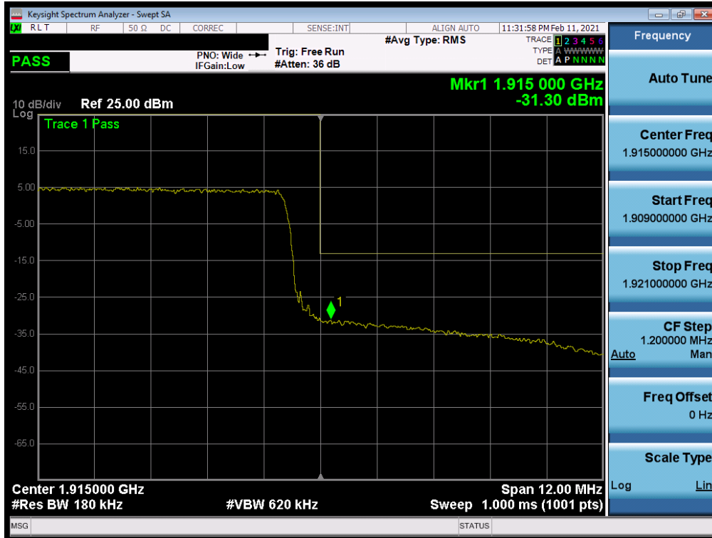
Plot 7-42. Upper Band Edge Plot (LTE Band 25 - 15MHz QPSK – Full RB Configuration)
