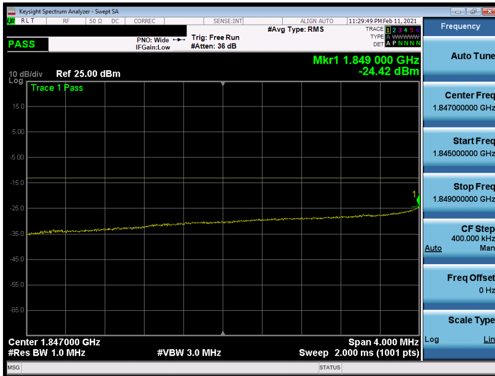
Plot 7-47. Extended Lower Band Edge Plot (LTE Band 25/2 - 10MHz QPSK – Full RB Configuration)
