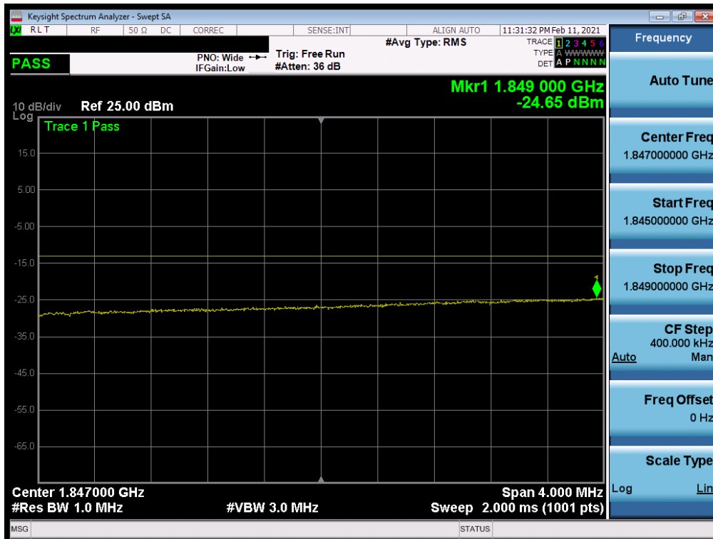
Plot 7-41. Extended Lower Band Edge Plot (LTE Band 25/2 - 15MHz QPSK – Full RB Configuration)
