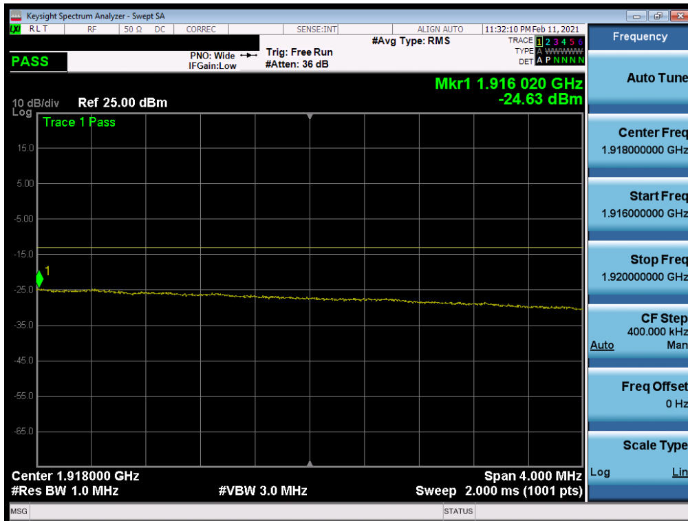
Plot 7-43. Extended Upper Band Edge Plot (LTE Band 25 - 15MHz QPSK – Full RB Configuration)
