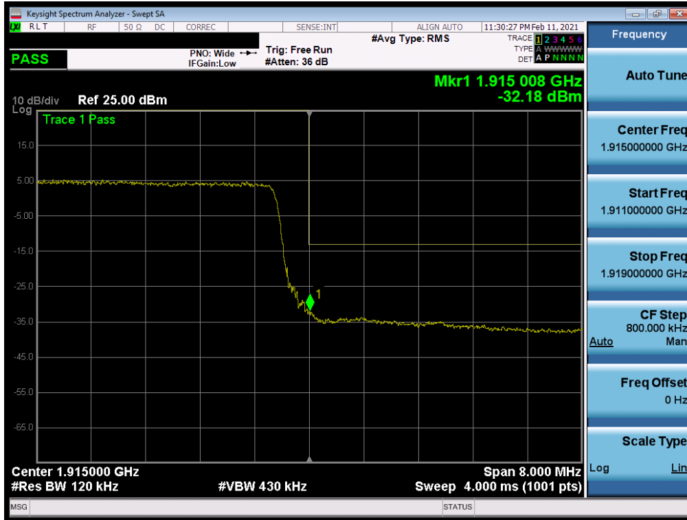
Plot 7-48. Upper Band Edge Plot (LTE Band 25 - 10MHz QPSK – Full RB Configuration)
