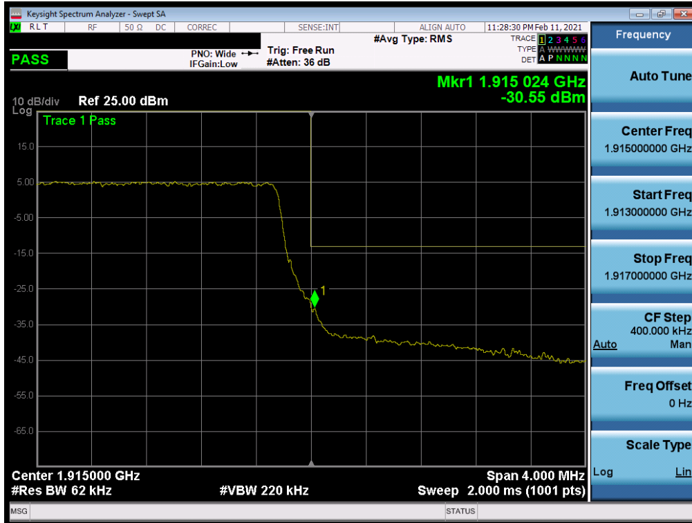
Plot 7-54. Upper Band Edge Plot (LTE Band 25 - 5MHz QPSK – Full RB Configuration)
