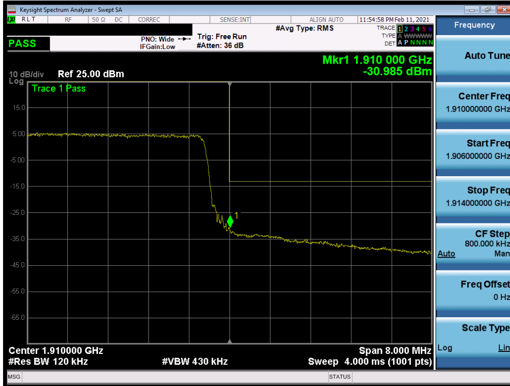
Plot 7-50. Upper Band Edge Plot (LTE Band 2 - 10MHz QPSK – Full RB Configuration)
