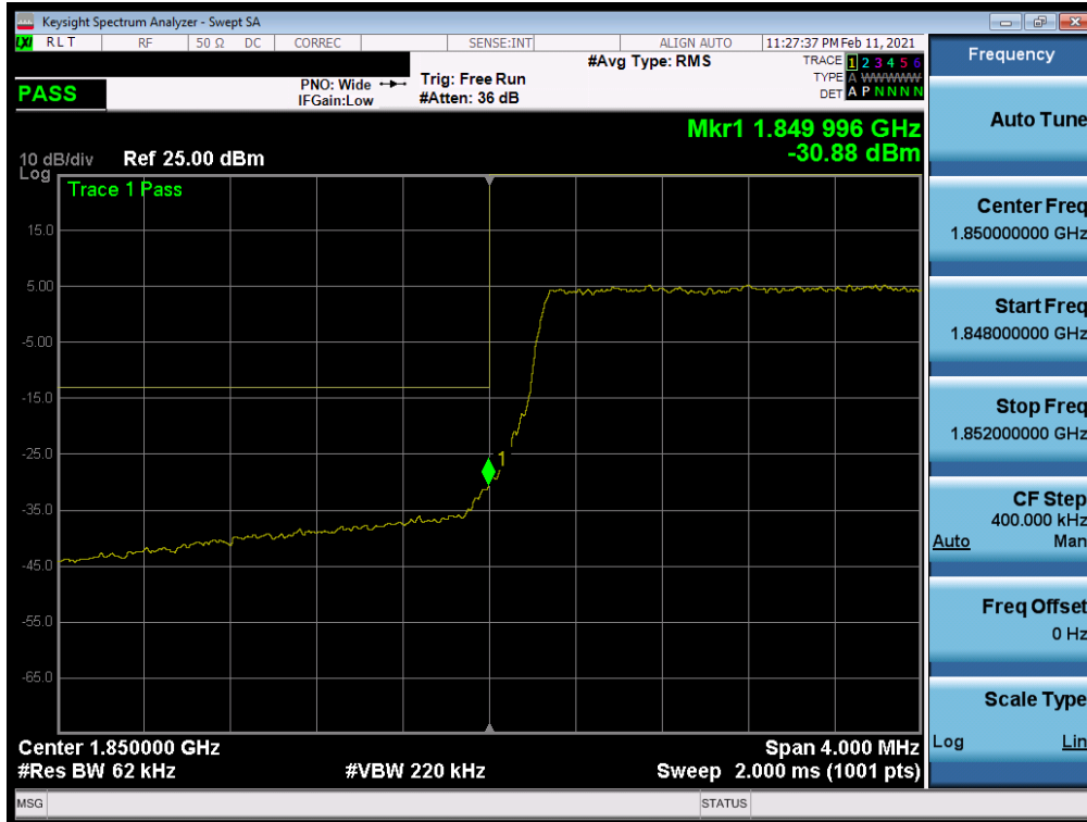
Plot 7-52. Lower Band Edge Plot (LTE Band 25/2 - 5MHz QPSK – Full RB Configuration)
