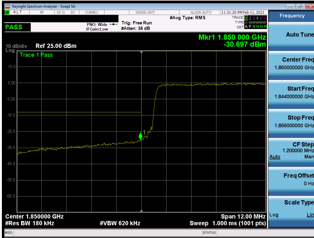
Plot 7-40. Lower Band Edge Plot (LTE Band 25/2 - 15MHz QPSK – Full RB Configuration)
