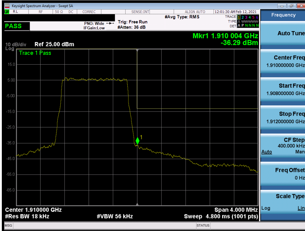
Plot 7-68. Upper Band Edge Plot (LTE Band 2 – 1.4MHz QPSK – Full RB Configuration)
