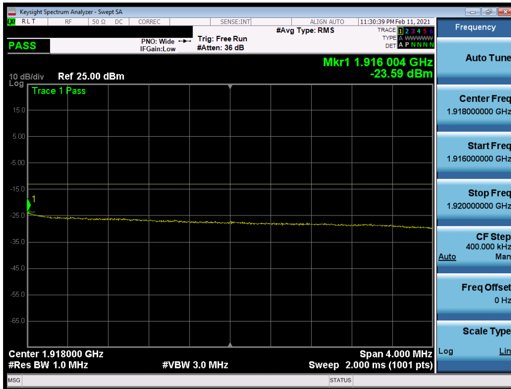
Plot 7-49. Extended Upper Band Edge Plot (LTE Band 25 - 10MHz QPSK – Full RB Configuration)
