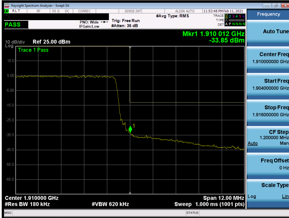
Plot 7-44. Upper Band Edge Plot (LTE Band 2 - 15MHz QPSK – Full RB Configuration)
