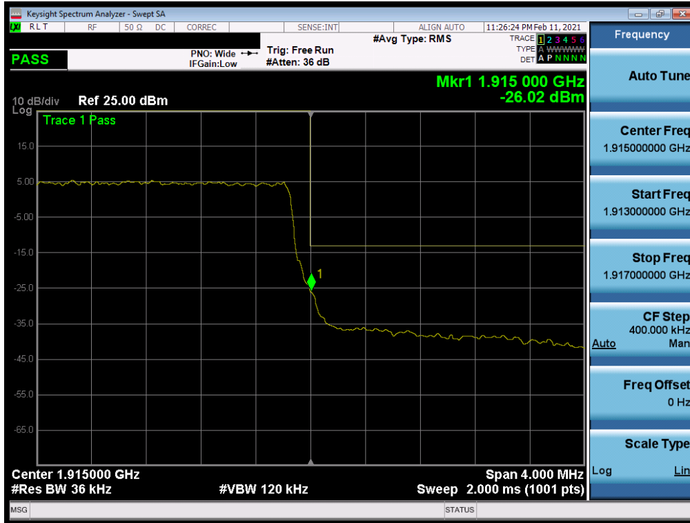
Plot 7-60. Upper Band Edge Plot (LTE Band 25 - 3MHz QPSK – Full RB Configuration)
