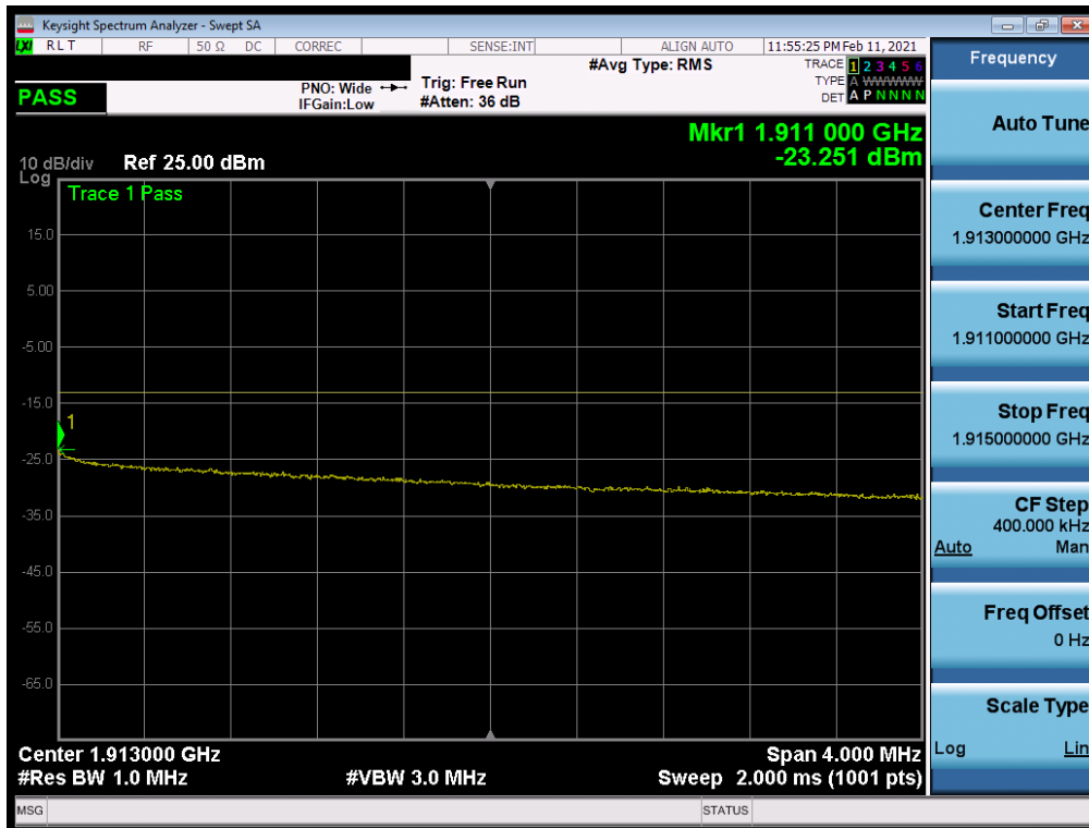
Plot 7-51. Extended Upper Band Edge Plot (LTE Band 2 - 10MHz QPSK – Full RB Configuration)
