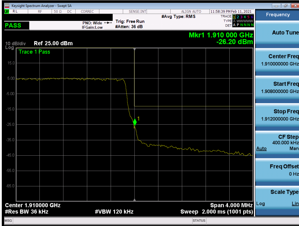
Plot 7-62. Upper Band Edge Plot (LTE Band 2 - 3MHz QPSK – Full RB Configuration)
