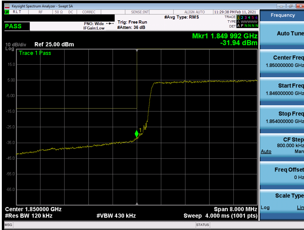
Plot 7-46. Lower Band Edge Plot (LTE Band 25/2 - 10MHz QPSK – Full RB Configuration)
