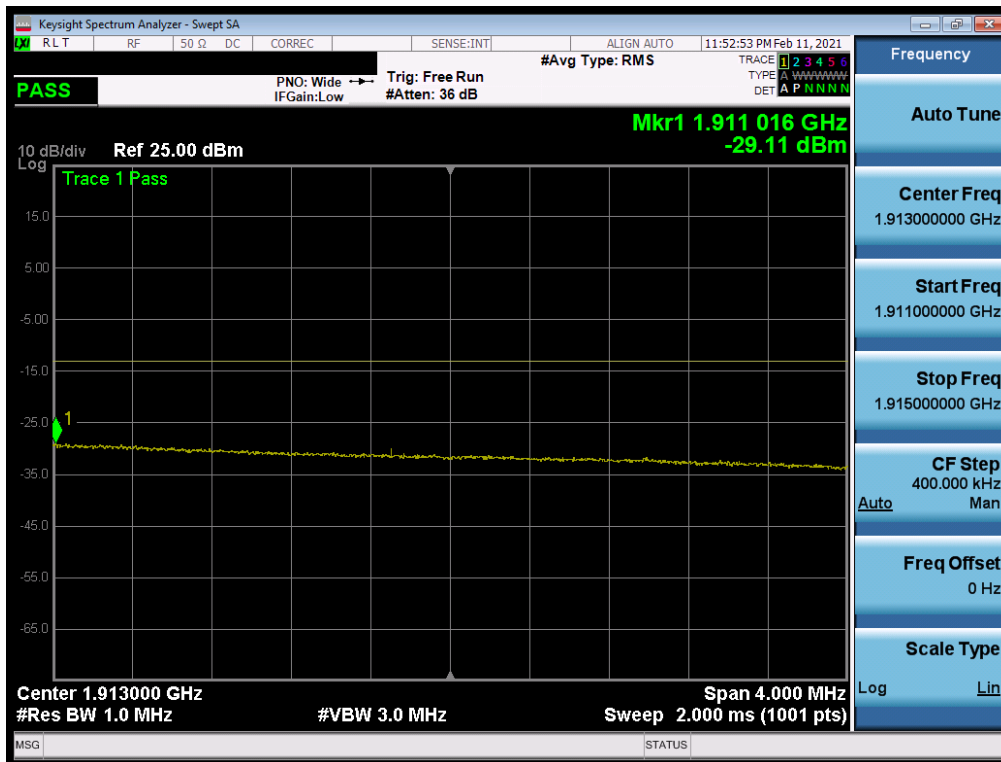
Plot 7-39. Extended Upper Band Edge Plot (LTE Band 2 - 20MHz QPSK – Full RB Configuration)
