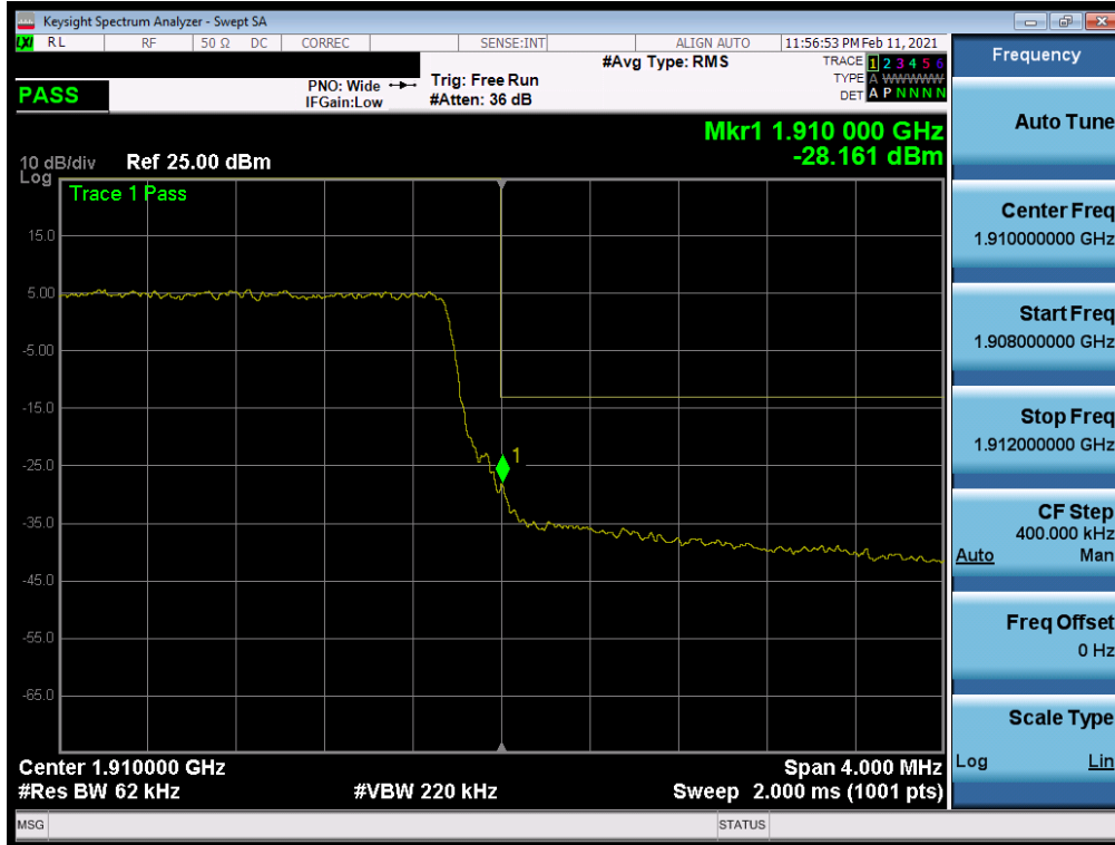
Plot 7-56. Upper Band Edge Plot (LTE Band 2 - 5MHz QPSK – Full RB Configuration)
