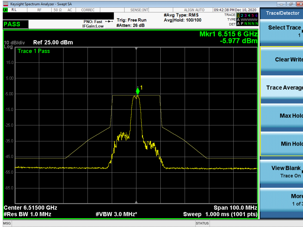
Plot 7-307. In-Band Emissions Plot MIMO ANT1 (20MHz BW 802.11ax (26 Tones) (UNII Band 6) – Ch. 113)
