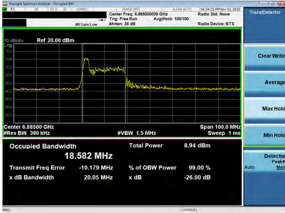
Plot 7-35. 26dB Bandwidth Plot MIMO ANT1 (40MHz BW 802.11ax (26 Tones) (UNII Band 8) – Ch. 187)
