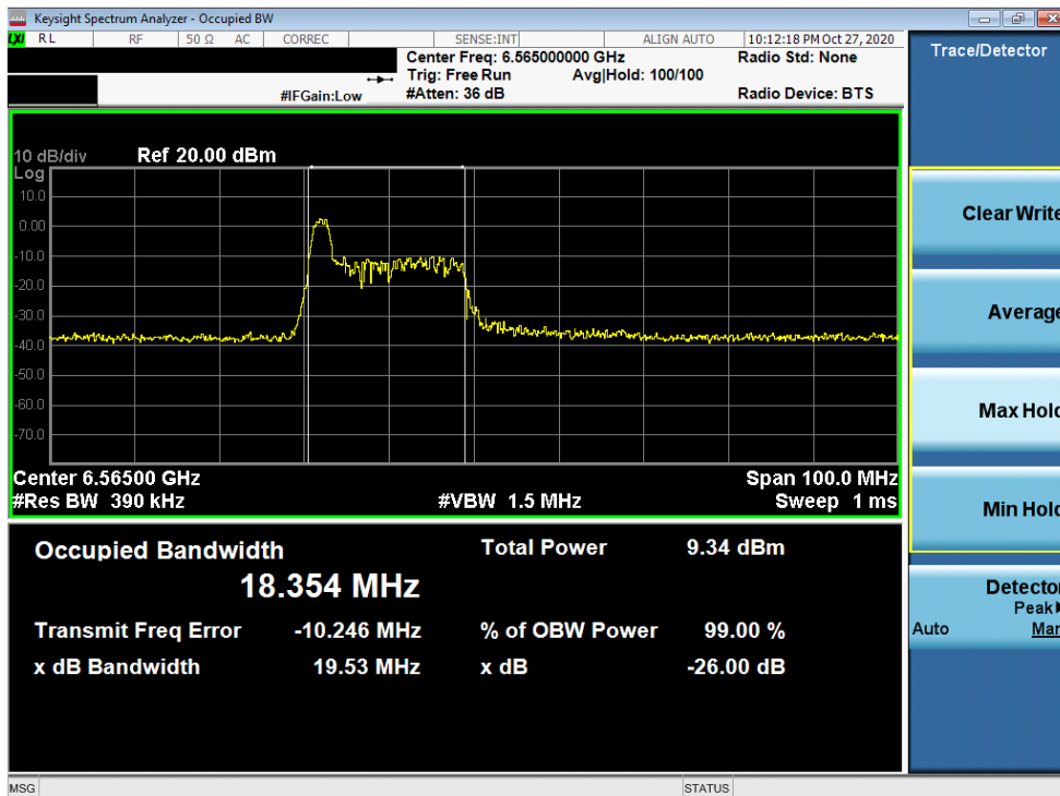
Plot 7-97. 26dB Bandwidth Plot MIMO ANT2 (40MHz BW 802.11ax (26 Tones) (UNII Band 7) – Ch. 123)
