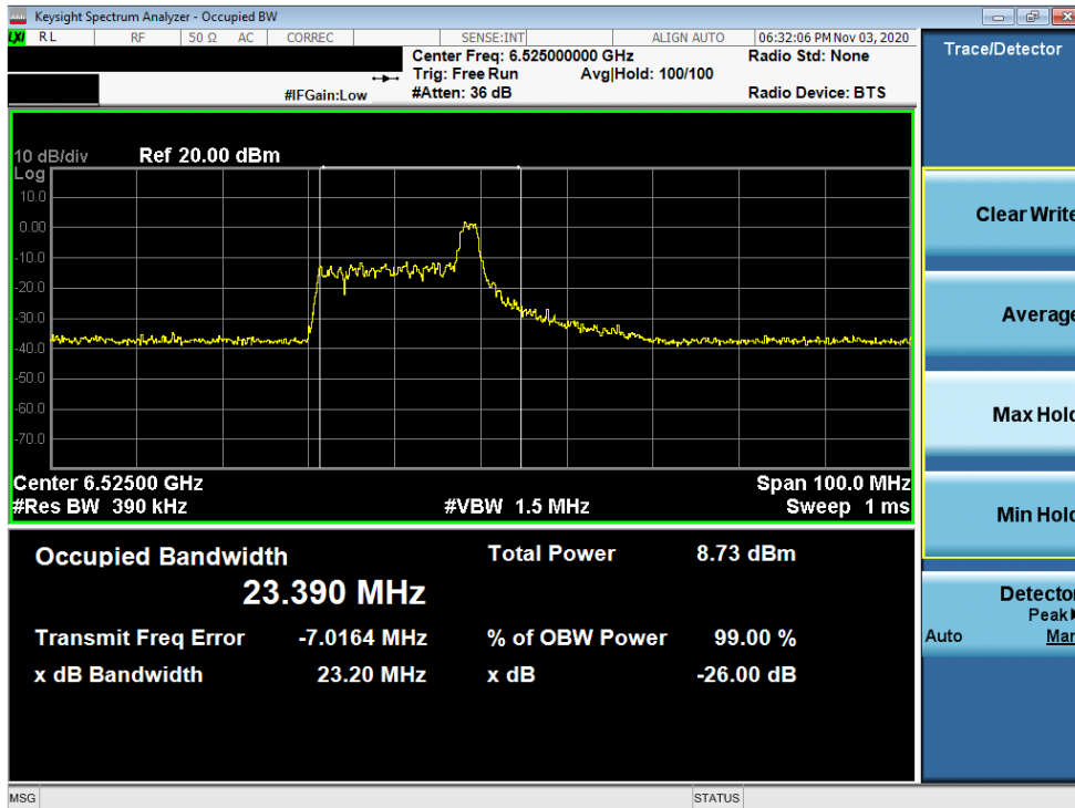
Plot 7-18. 26dB Bandwidth Plot MIMO ANT1 (40MHz BW 802.11ax (26 Tones) (UNII Band 6) – Ch. 115)
