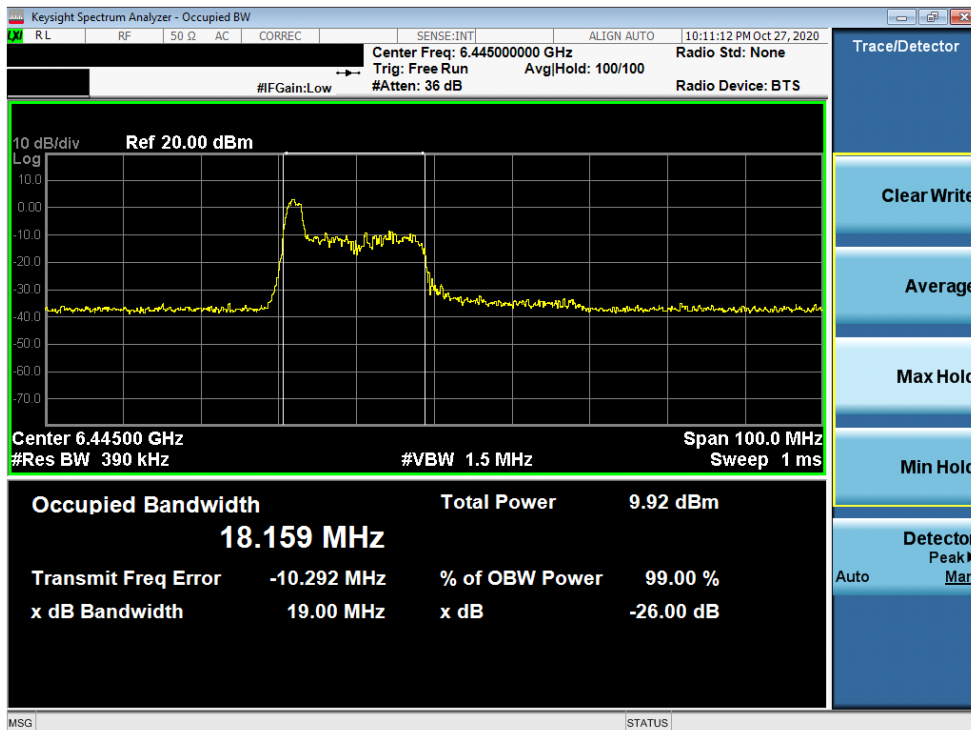
Plot 7-89. 26dB Bandwidth Plot MIMO ANT2 (40MHz BW 802.11ax (26 Tones) (UNII Band 6) – Ch. 99)
