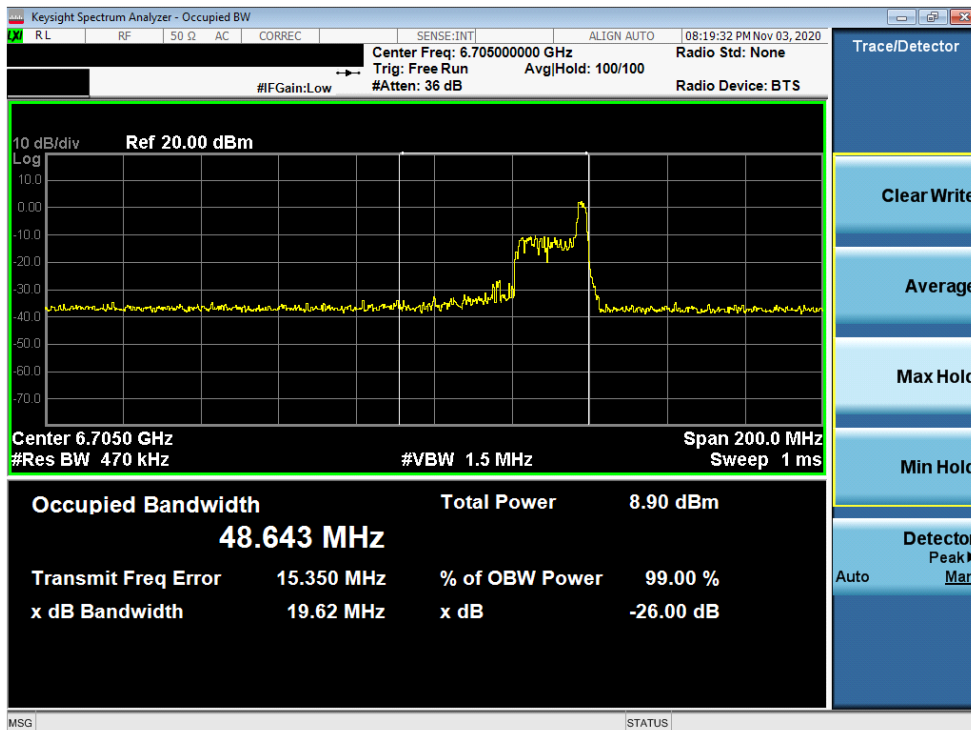
Plot 7-28. 26dB Bandwidth Plot MIMO ANT1 (80MHz BW 802.11ax (26 Tones) (UNII Band 7) – Ch. 151)
