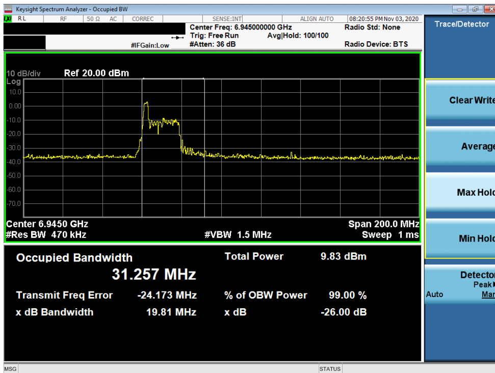
Plot 7-38. 26dB Bandwidth Plot MIMO ANT1 (80MHz BW 802.11ax (26 Tones) (UNII Band 8) – Ch. 199)
