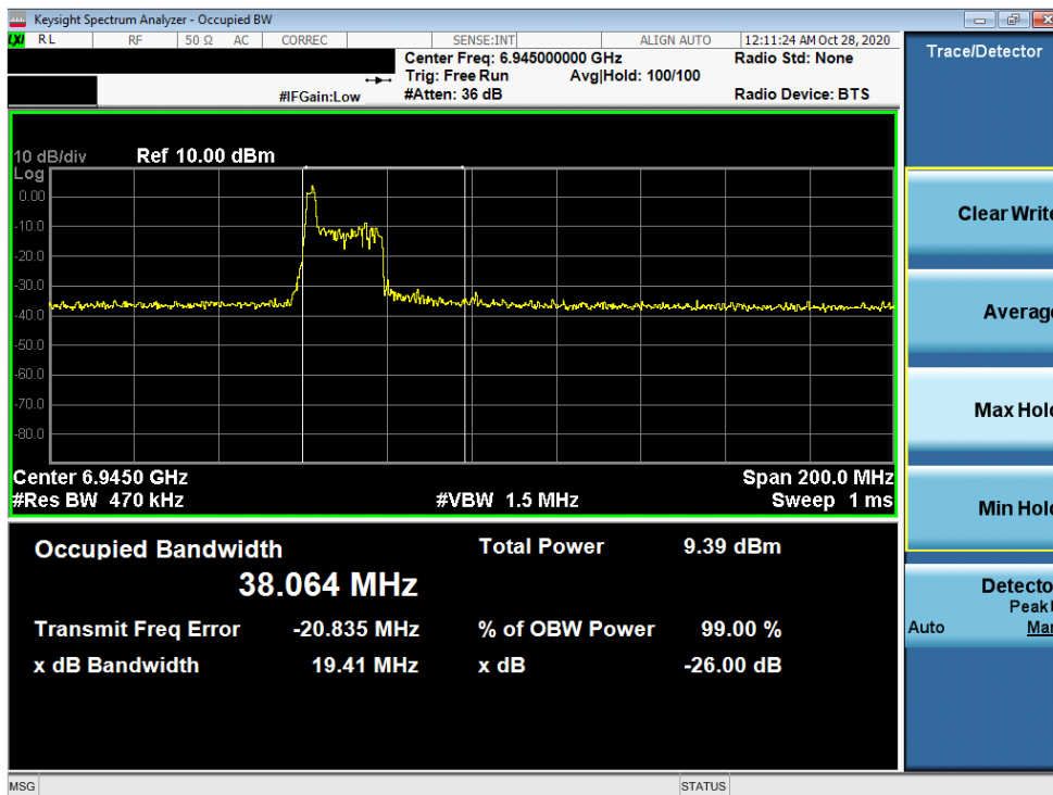
Plot 7-111. 26dB Bandwidth Plot MIMO ANT2 (80MHz BW 802.11ax (26 Tones) (UNII Band 8) – Ch. 199)
