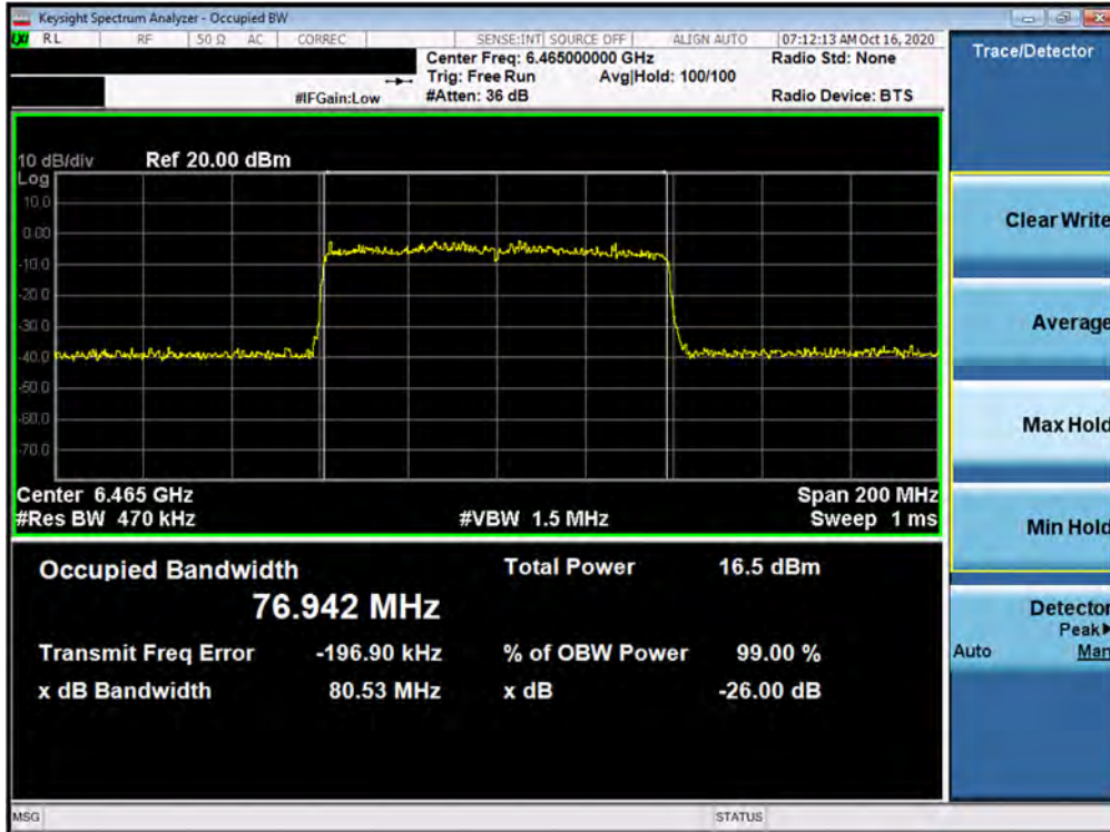
Plot 7-25. 26dB Bandwidth Plot MIMO ANT1 (80MHz BW 802.11ax (UNII Band 6) – Ch. 103)
