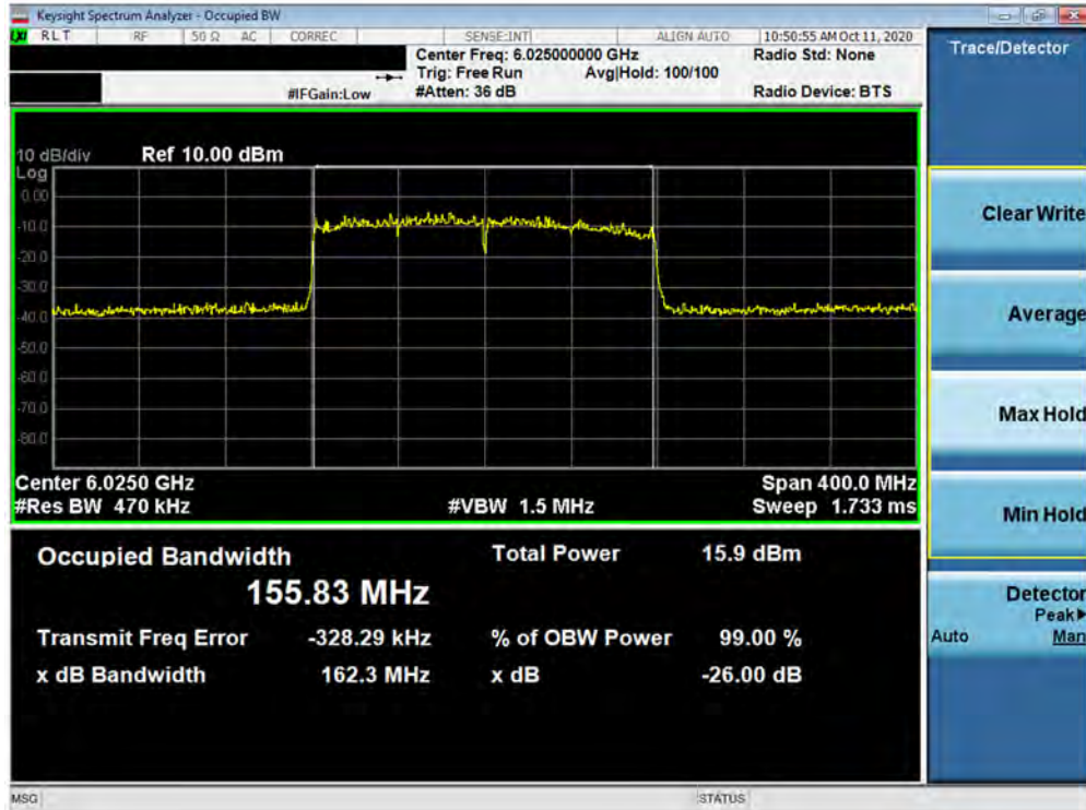
Plot 7-13. 26dB Bandwidth Plot MIMO ANT1 (160MHz BW 802.11ax (UNII Band 5) – Ch. 15)
