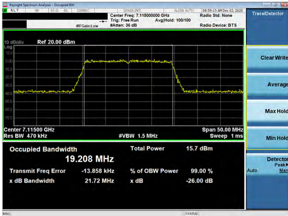
Plot 7-46. 26dB Bandwidth Plot MIMO ANT1 (20MHz BW 802.11ax (UNII Band 8) – Ch. 233)
