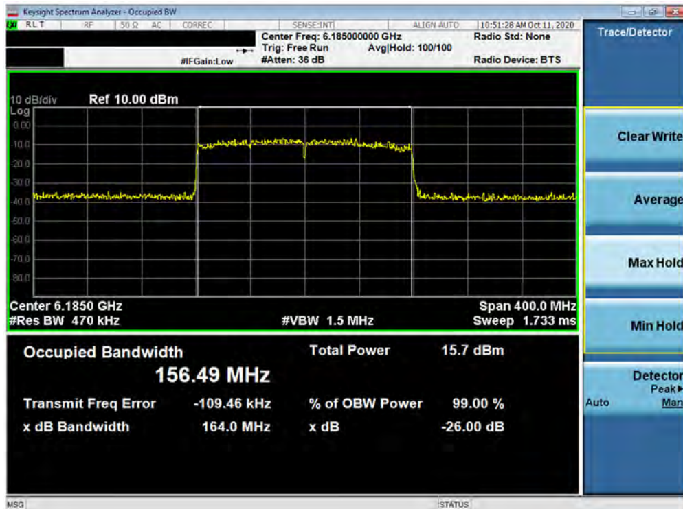
Plot 7-14. 26dB Bandwidth Plot MIMO ANT1 (160MHz BW 802.11ax (UNII Band 5) – Ch. 47)
