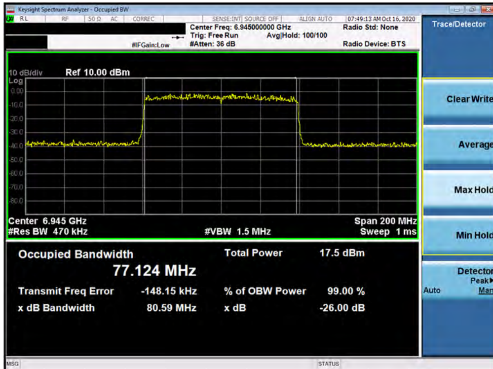
Plot 7-102. 26dB Bandwidth Plot MIMO ANT2 (80MHz BW 802.11ax (UNII Band 8) – Ch. 199)
