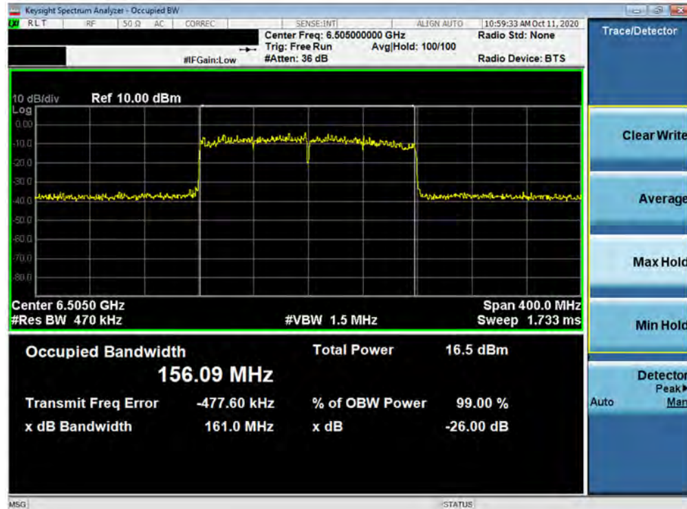
Plot 7-78. 26dB Bandwidth Plot MIMO ANT2 (160MHz BW 802.11ax (UNII Band 6) – Ch. 111)
