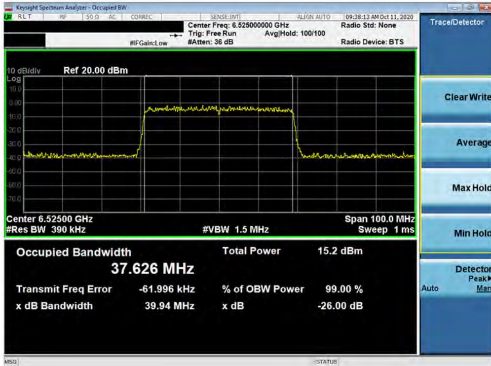
Plot 7-24. 26dB Bandwidth Plot MIMO ANT1 (40MHz BW 802.11ax (UNII Band 6) – Ch. 115)
