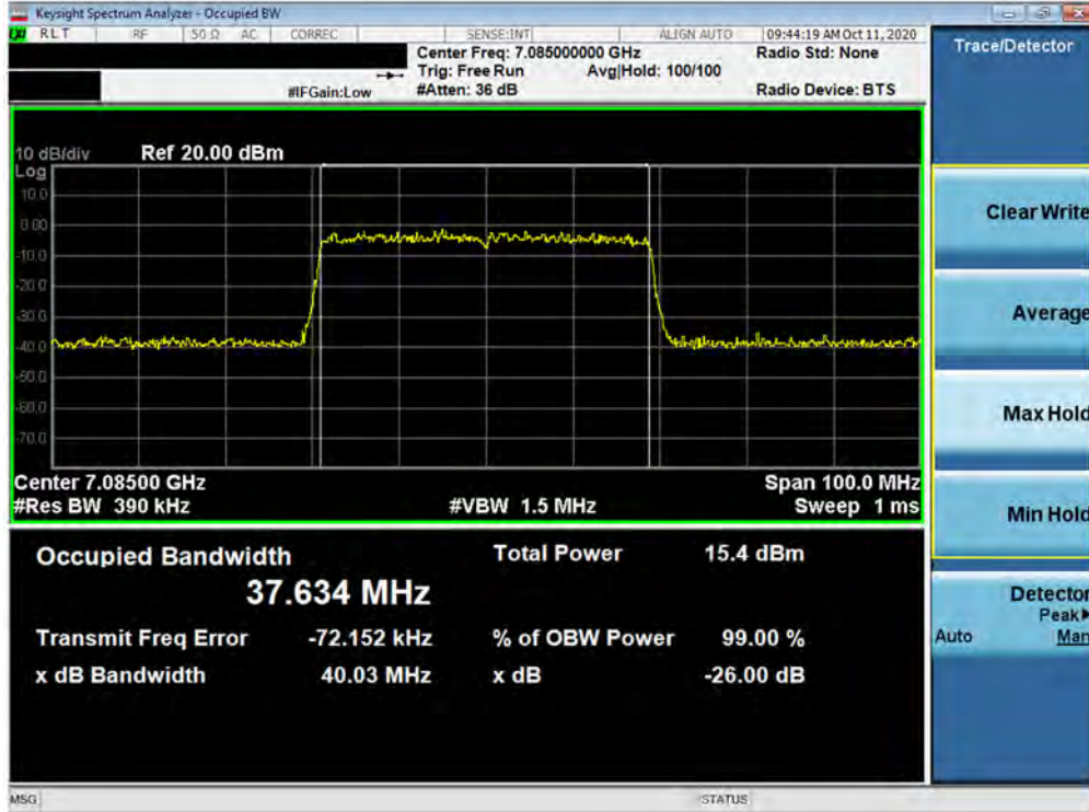
Plot 7-49. 26dB Bandwidth Plot MIMO ANT1 (40MHz BW 802.11ax (UNII Band 8) – Ch. 227)
