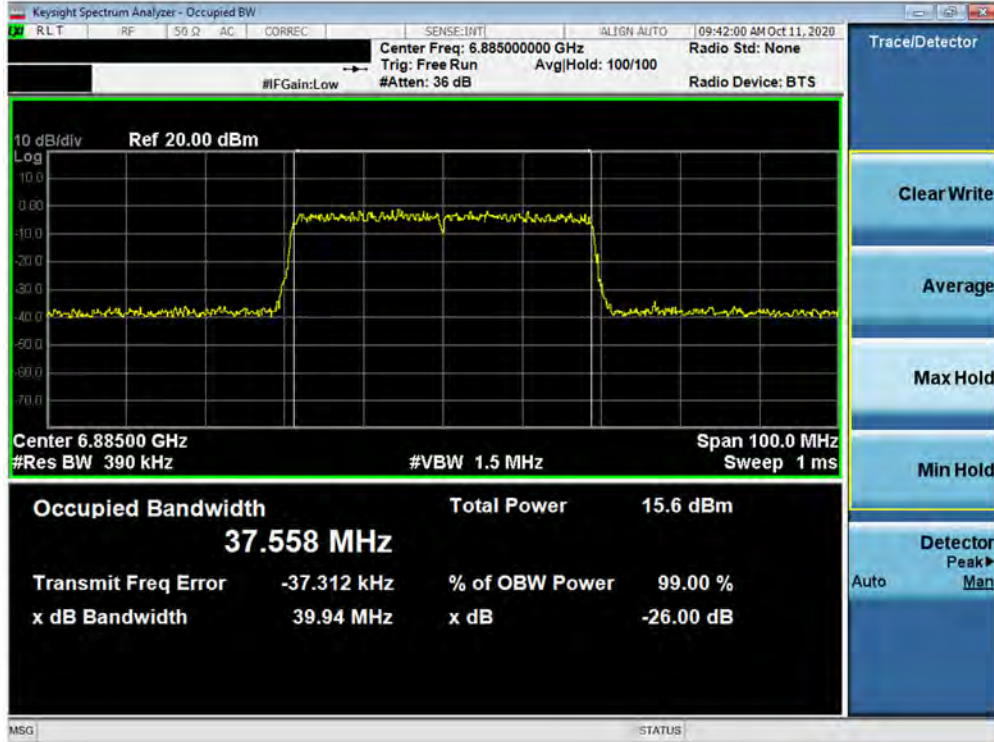
Plot 7-47. 26dB Bandwidth Plot MIMO ANT1 (40MHz BW 802.11ax (UNII Band 8) – Ch. 187)
