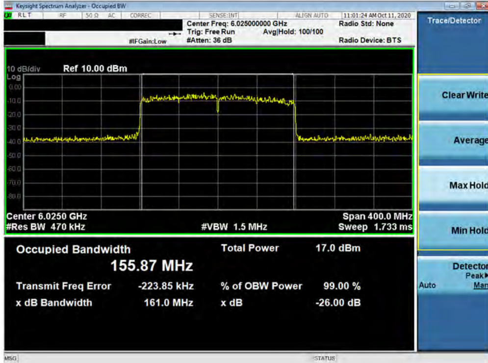
Plot 7-65. 26dB Bandwidth Plot MIMO ANT2 (160MHz BW 802.11ax (UNII Band 5) – Ch. 15)
