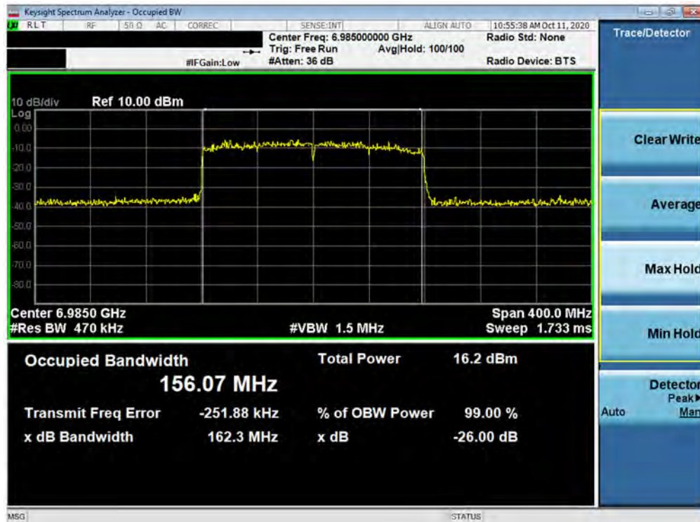
Plot 7-52. 26dB Bandwidth Plot MIMO ANT1 (160MHz BW 802.11ax (UNII Band 8) – Ch. 207)
