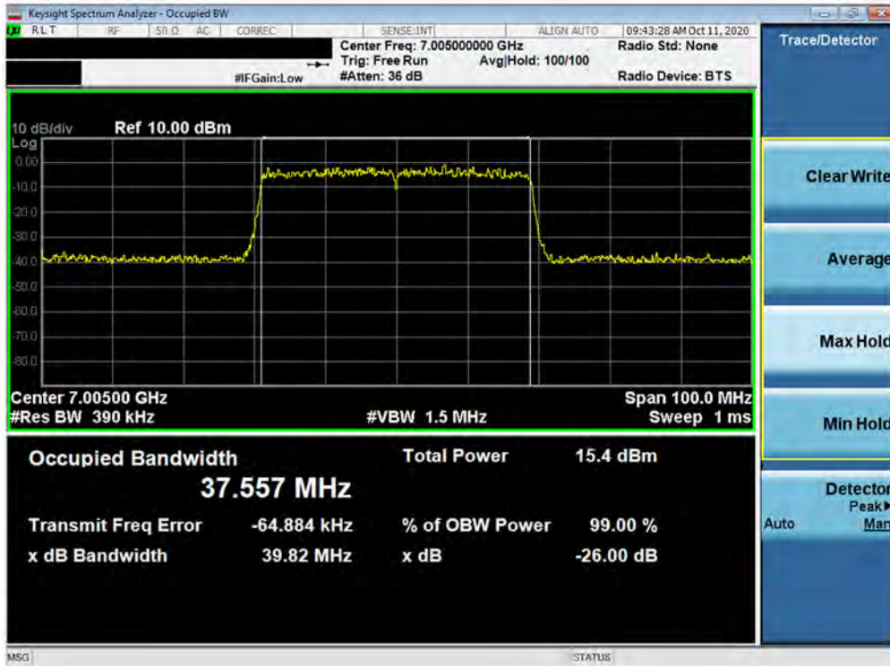
Plot 7-48. 26dB Bandwidth Plot MIMO ANT1 (40MHz BW 802.11ax (UNII Band 8) – Ch. 211)
