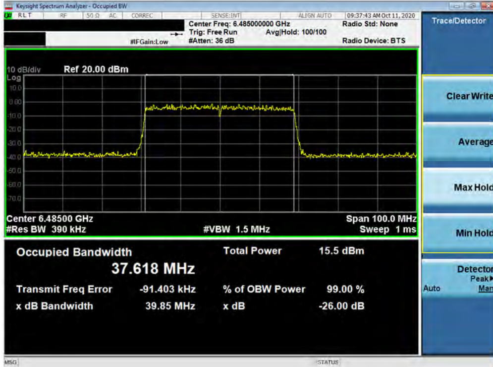
Plot 7-23. 26dB Bandwidth Plot MIMO ANT1 (40MHz BW 802.11ax (UNII Band 6) – Ch. 107)
