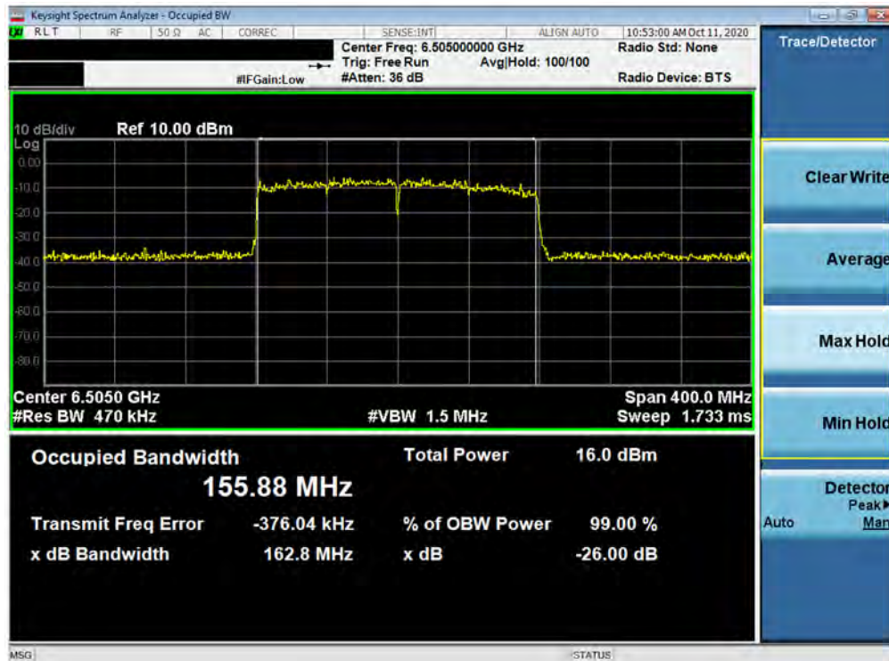
Plot 7-26. 26dB Bandwidth Plot MIMO ANT1 (160MHz BW 802.11ax (UNII Band 6) – Ch. 111)
