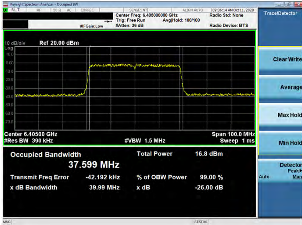
Plot 7-9. 26dB Bandwidth Plot MIMO ANT1 (40MHz BW 802.11ax (UNII Band 5) – Ch. 91)
