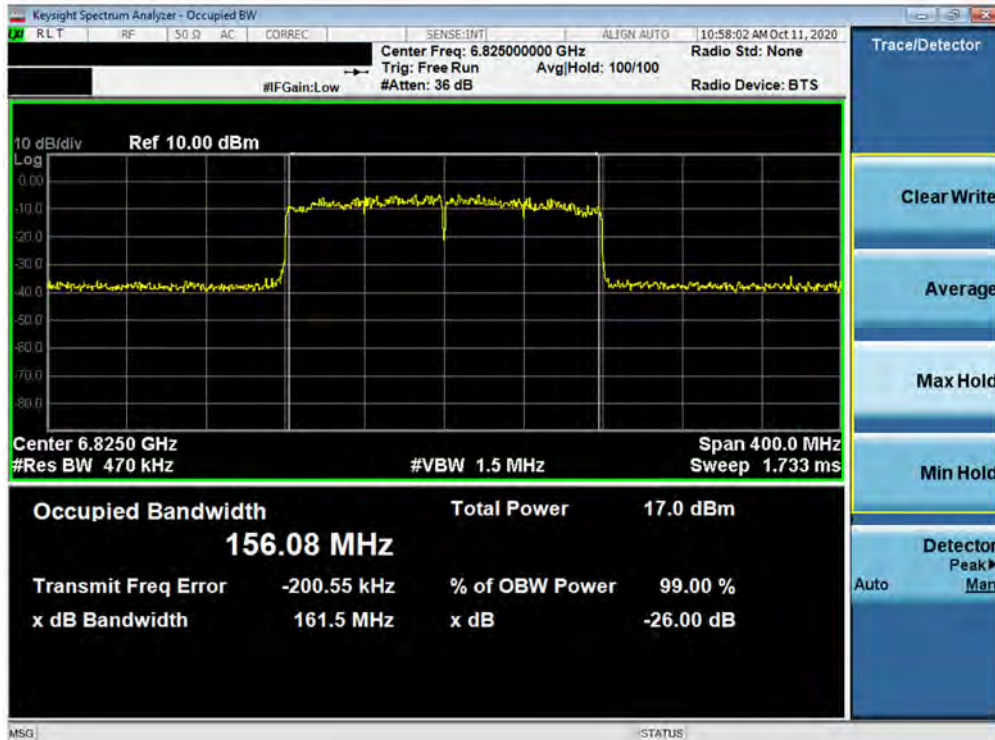
Plot 7-92. 26dB Bandwidth Plot MIMO ANT2 (160MHz BW 802.11ax (UNII Band 7) – Ch. 175)
