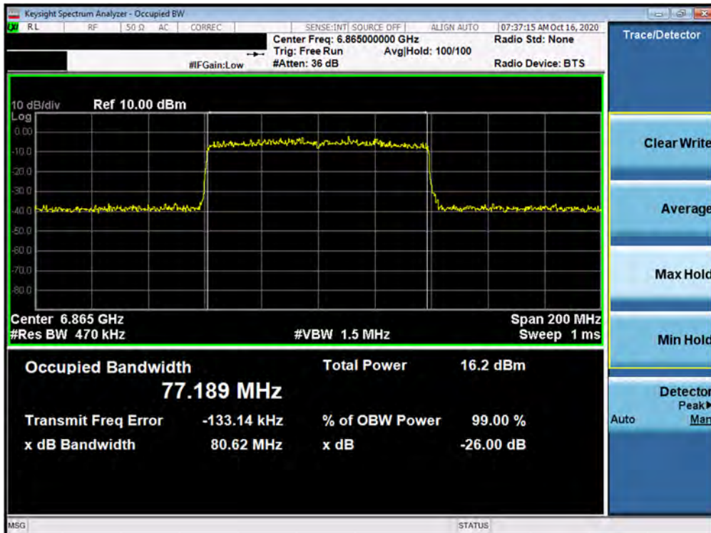
Plot 7-38. 26dB Bandwidth Plot MIMO ANT1 (80MHz BW 802.11ax (UNII Band 7) – Ch. 183)
