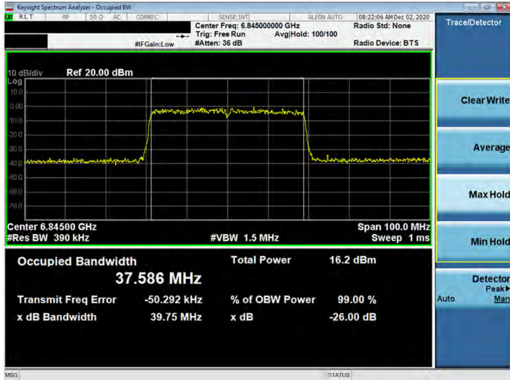
Plot 7-87. 26dB Bandwidth Plot MIMO ANT2 (40MHz BW 802.11ax (UNII Band 7) – Ch. 179)
