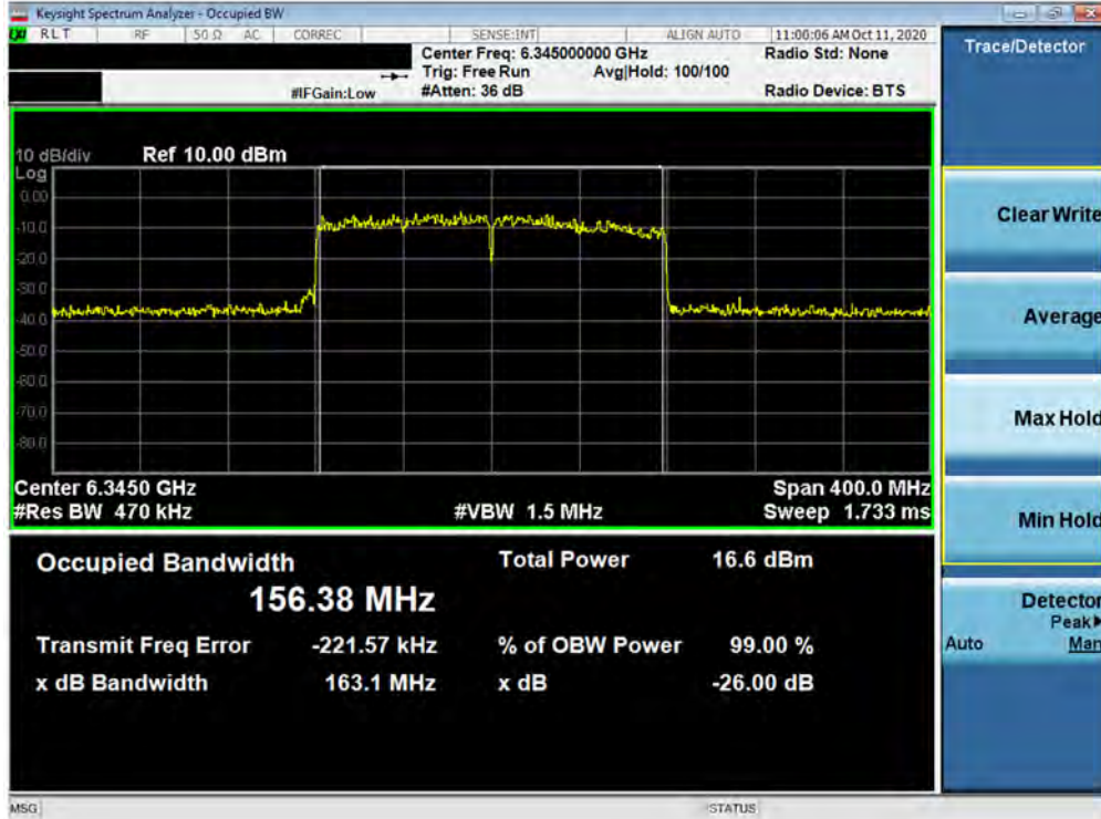
Plot 7-67. 26dB Bandwidth Plot MIMO ANT2 (160MHz BW 802.11ax (UNII Band 5) – Ch. 79)
