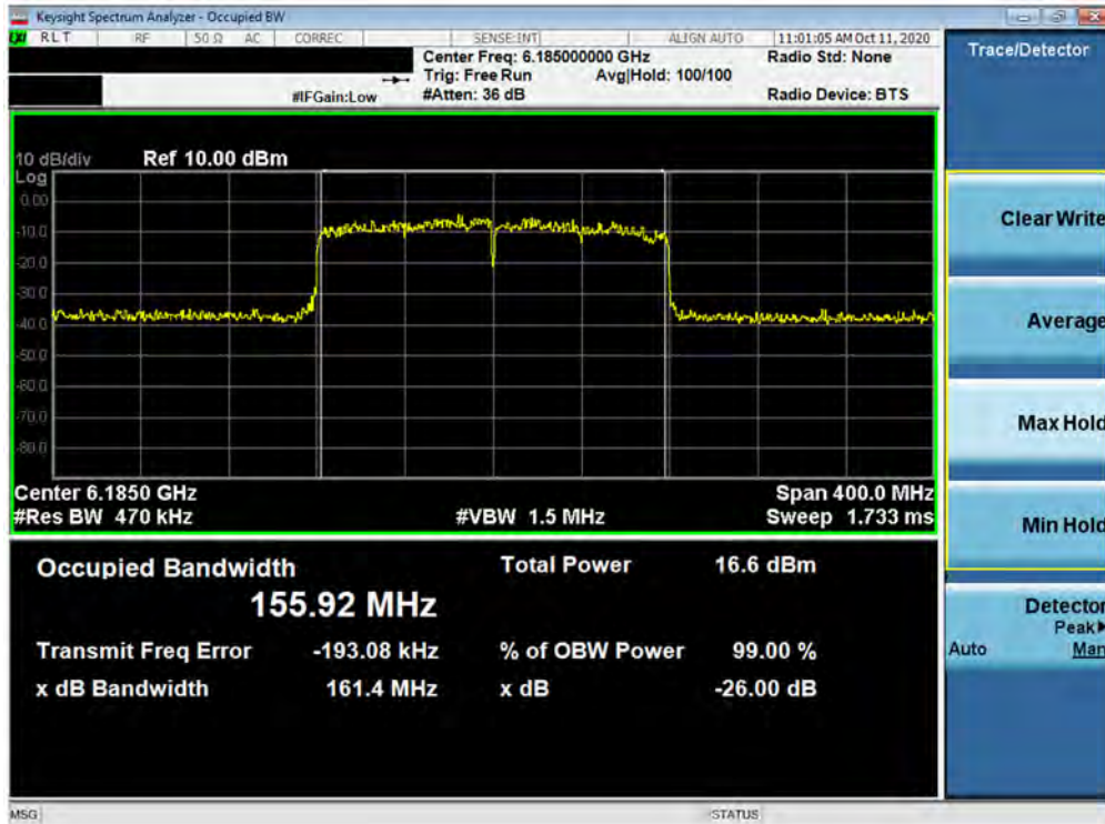
Plot 7-66. 26dB Bandwidth Plot MIMO ANT2 (160MHz BW 802.11ax (UNII Band 5) – Ch. 47)
