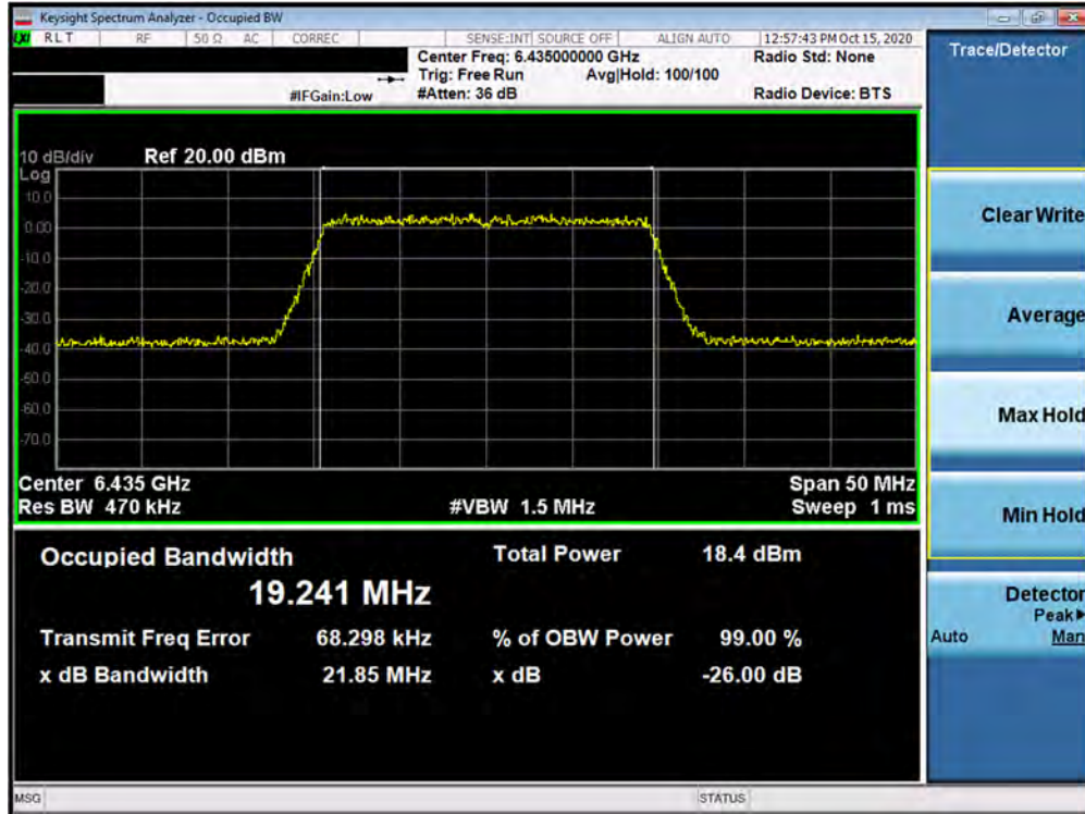
Plot 7-19. 26dB Bandwidth Plot MIMO ANT1 (20MHz BW 802.11ax (UNII Band 6) – Ch. 97)
