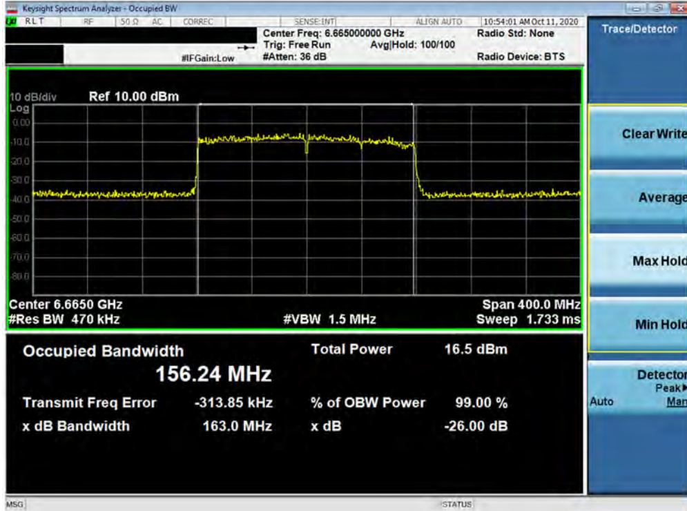
Plot 7-39. 26dB Bandwidth Plot MIMO ANT1 (160MHz BW 802.11ax (UNII Band 7) – Ch. 143)
