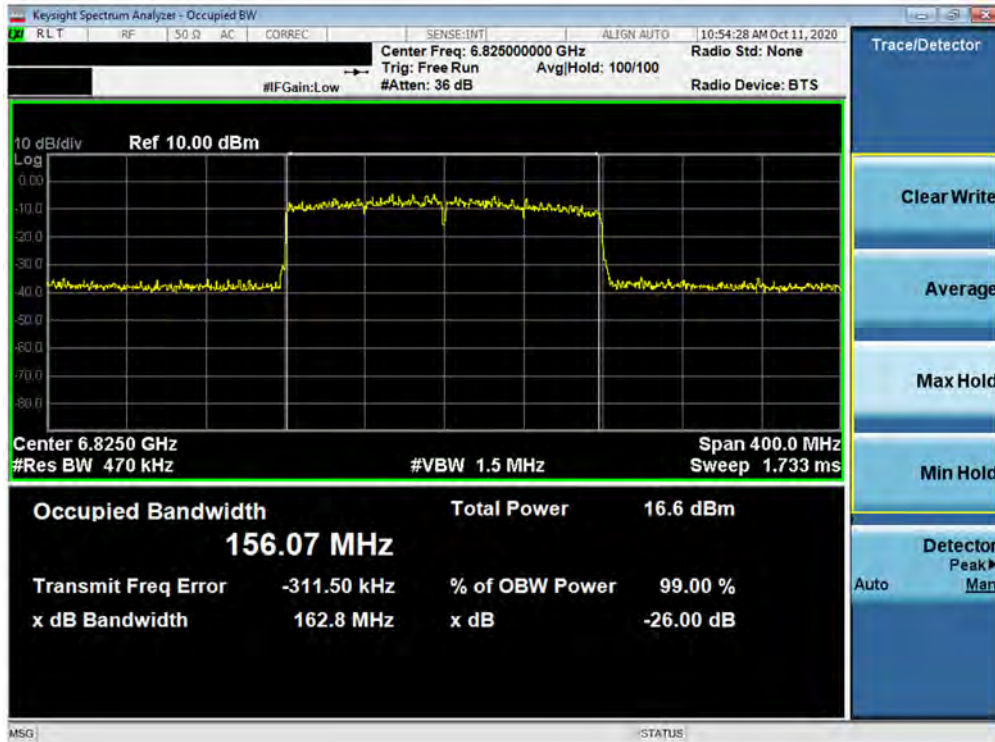
Plot 7-40. 26dB Bandwidth Plot MIMO ANT1 (160MHz BW 802.11ax (UNII Band 7) – Ch. 175)
