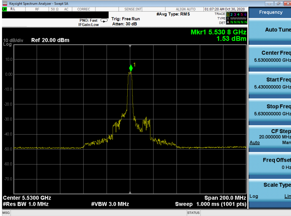
Plot 7-181. Power Spectral Density Plot MIMO ANT2 (80MHz BW 802.11ax – 26 Tones (UNII Band 2C) – Ch. 106)
