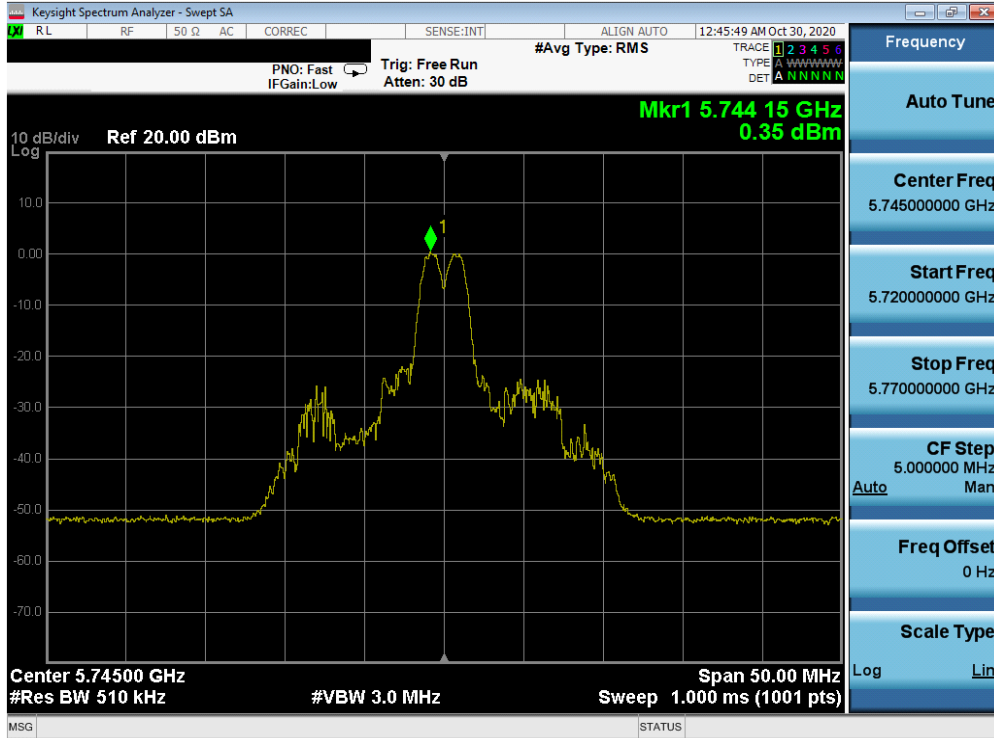
Plot 7-184. Power Spectral Density Plot MIMO ANT2 (20MHz BW 802.11ax – 26 Tones (UNII Band 3) – Ch. 149)
