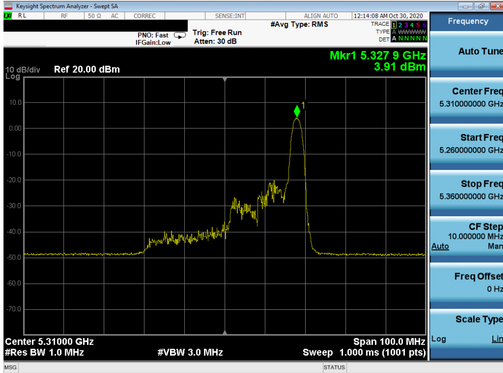
Plot 7-119. Power Spectral Density Plot MIMO ANT1 (40MHz BW 802.11ax – 26 Tones (UNII Band 2A) – Ch. 62)
