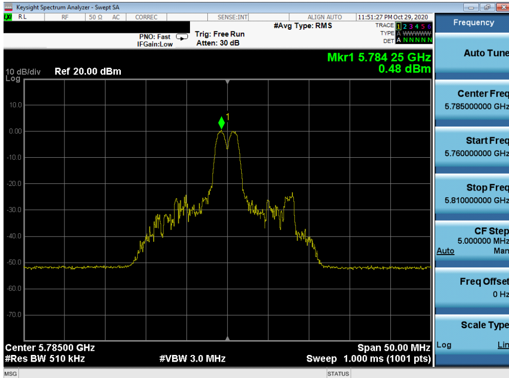
Plot 7-131. Power Spectral Density Plot MIMO ANT1 (20MHz BW 802.11ax – 26 Tones (UNII Band 3) – Ch. 157)
