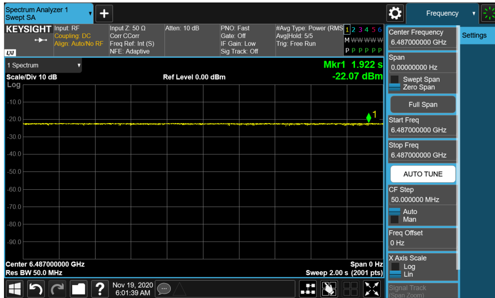
Plot 7-146. UWB Peak Power Measurement - ANT 1 - CH.5 – SP0 – BPRF
