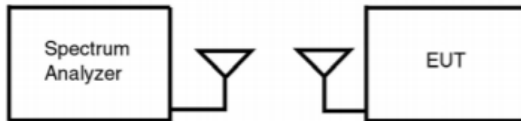
Figure 7-2. Test Instrument and Measurement Setup
