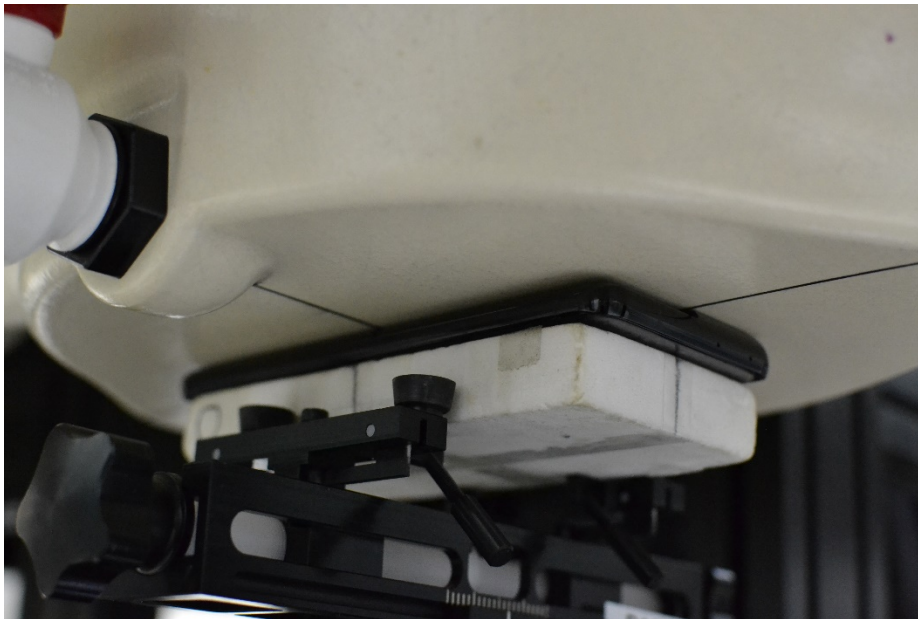
Figure C-8 SAR Test Setup Photo – Phablet Back Side at 0 mm
