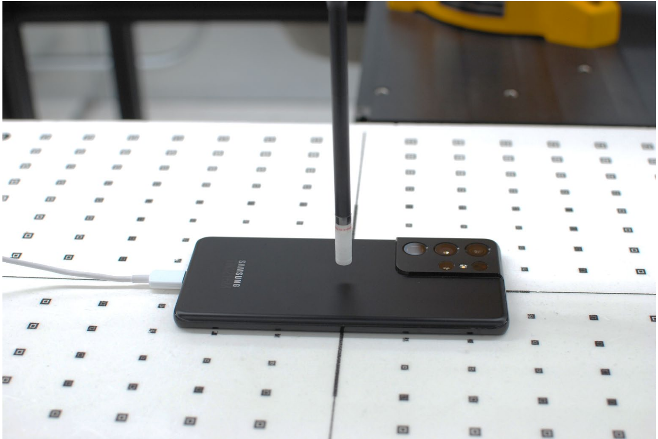
Figure C-13 Near Field Power Density Test Setup Photo – Back Side at 8.54 mm
