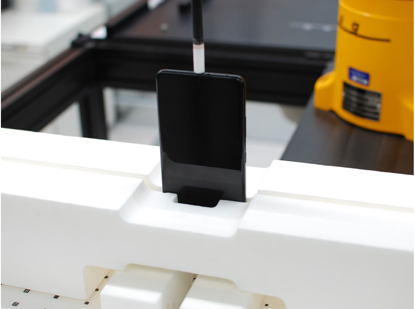
Figure C-17 Near Field Power Density Test Setup Photo – Top Edge at 2 mm
