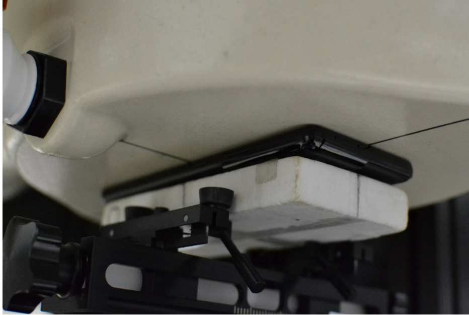
Figure C-9 SAR Test Setup Photo – Phablet Front Side at 0 mm
