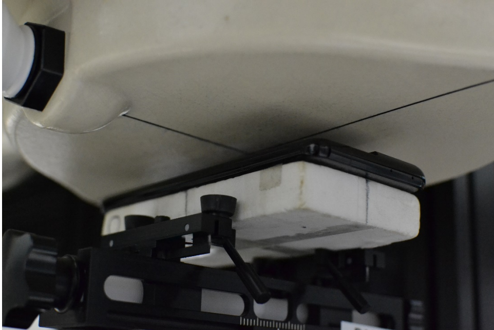
Figure C-7 SAR Test Setup Photo – Body-worn Back Side at 15 mm
