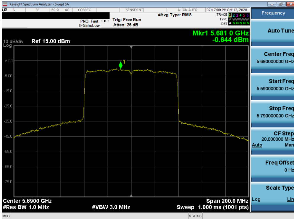
Plot 7-263. Power Spectral Density Plot MIMO ANT2 (80MHz BW 802.11ax (UNII Band 2C) – Ch. 138)
