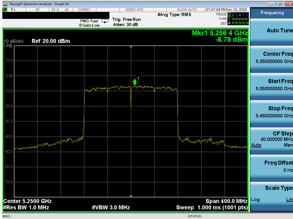
Plot 7-227. Power Spectral Density Plot MIMO ANT2 (160MHz BW 802.11ax (UNII Band 1) – Ch. 50)
