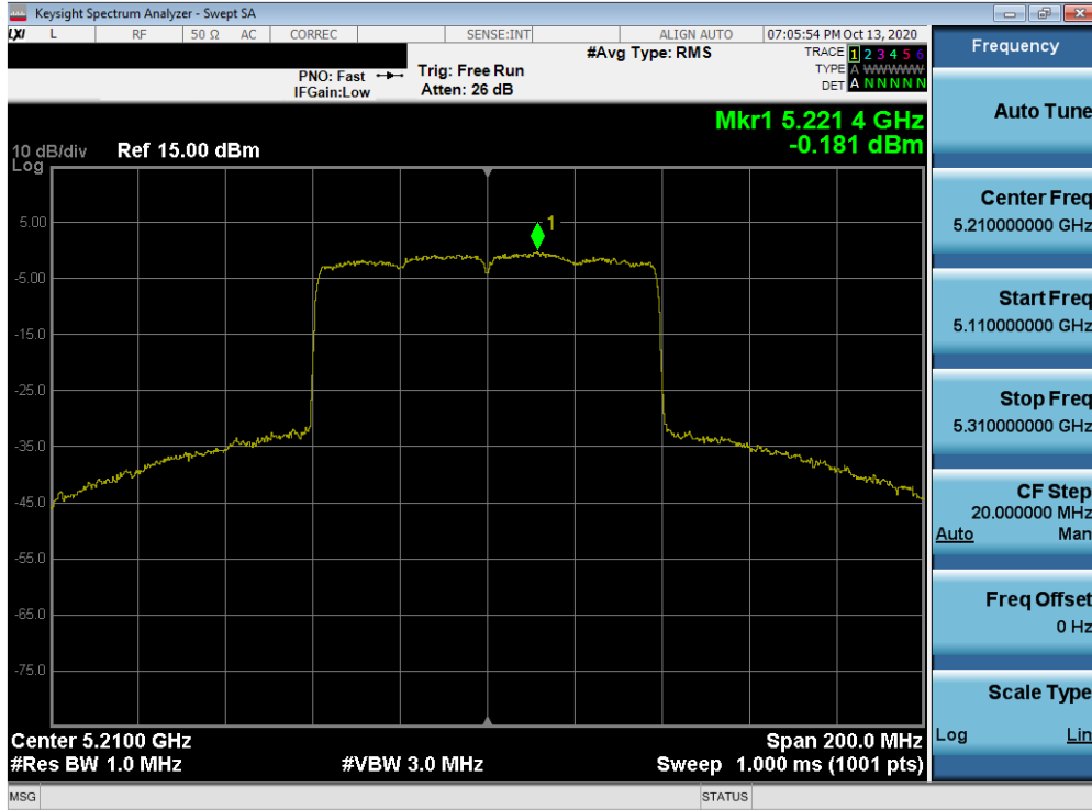
Plot 7-225. Power Spectral Density Plot MIMO ANT2 (80MHz BW 802.11ax (UNII Band 1) – Ch. 42)
