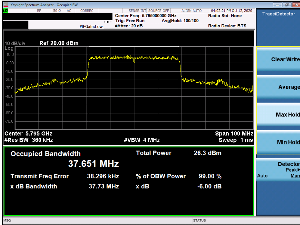
Plot 7-138. 6dB Bandwidth Plot MIMO ANT2 (40MHz BW 802.11ax (UNII Band 3) – Ch. 159)
