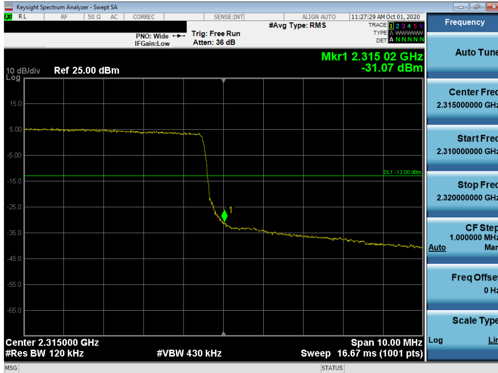
Plot 7-225. Upper Band Edge Plot (LTE Band 30 - 10MHz QPSK – Full RB Configuration)
