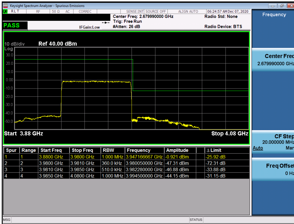
Plot 7-296. Upper ACP Plot (NR Band n77 - 60MHz CP-OFDM-QPSK – Full RB)
