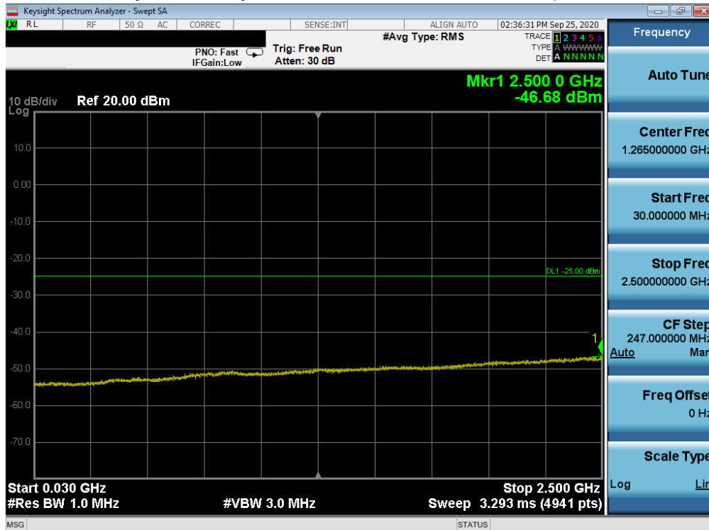
Plot 7-181. Conducted Spurious Plot (LTE Band 7 - 20MHz QPSK - RB Size 1, RB Offset 0 - Mid Channel)
