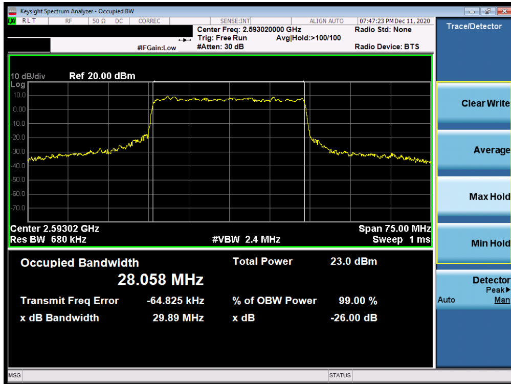
Plot 7-124. Occupied Bandwidth Plot (NR Band n41 - 30MHz CP-OFDM 64-QAM - Full RB)
