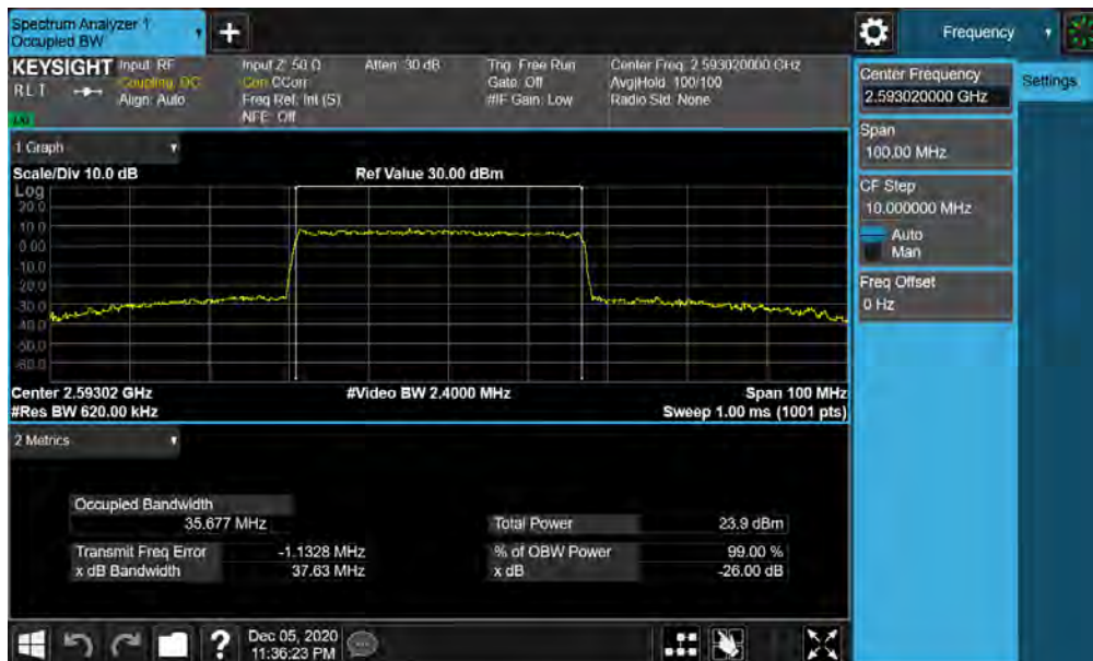
Plot 7-118. Occupied Bandwidth Plot (NR Band n41 - 40MHz CP-OFDM 16-QAM - Full RB)
