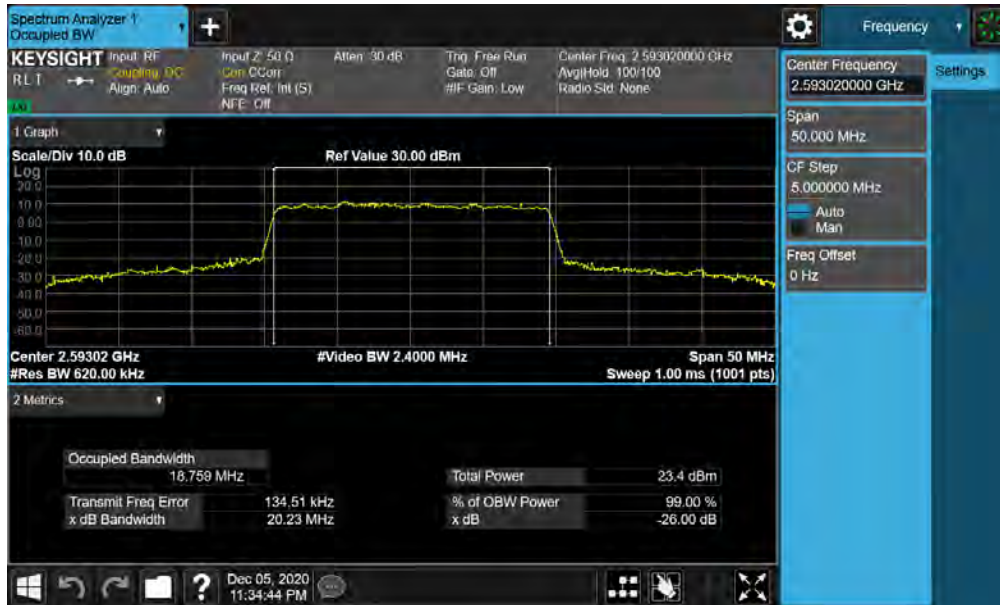
Plot 7-127. Occupied Bandwidth Plot (NR Band n41 - 20MHz CP-OFDM QPSK - Full RB)
