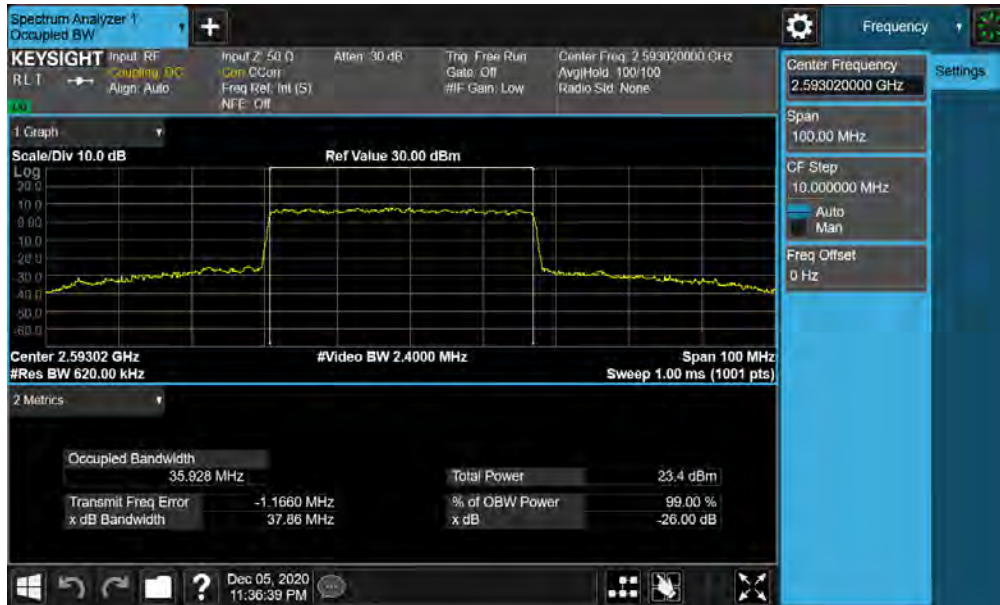
Plot 7-119. Occupied Bandwidth Plot (NR Band n41 - 40MHz CP-OFDM 64-QAM - Full RB)
