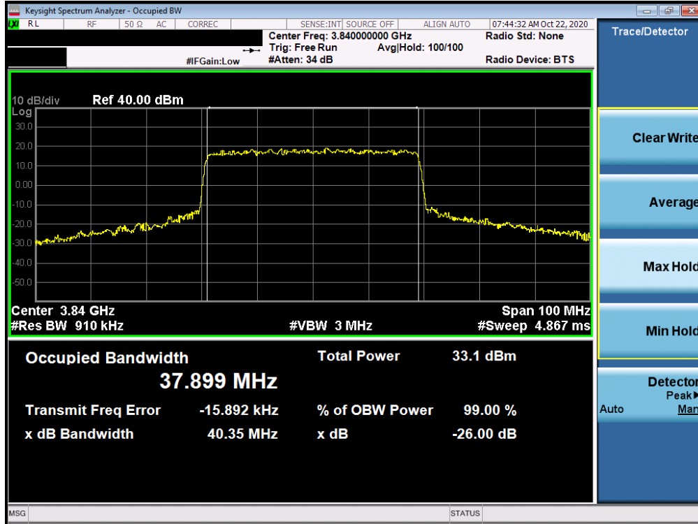
Plot 7-163. Occupied Bandwidth Plot (NR Band n77 - 40MHz CP-OFDM 64-QAM - Full RB)
