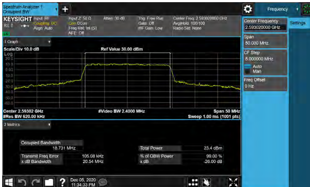
Plot 7-128. Occupied Bandwidth Plot (NR Band n41 - 20MHz CP-OFDM 16-QAM - Full RB)
