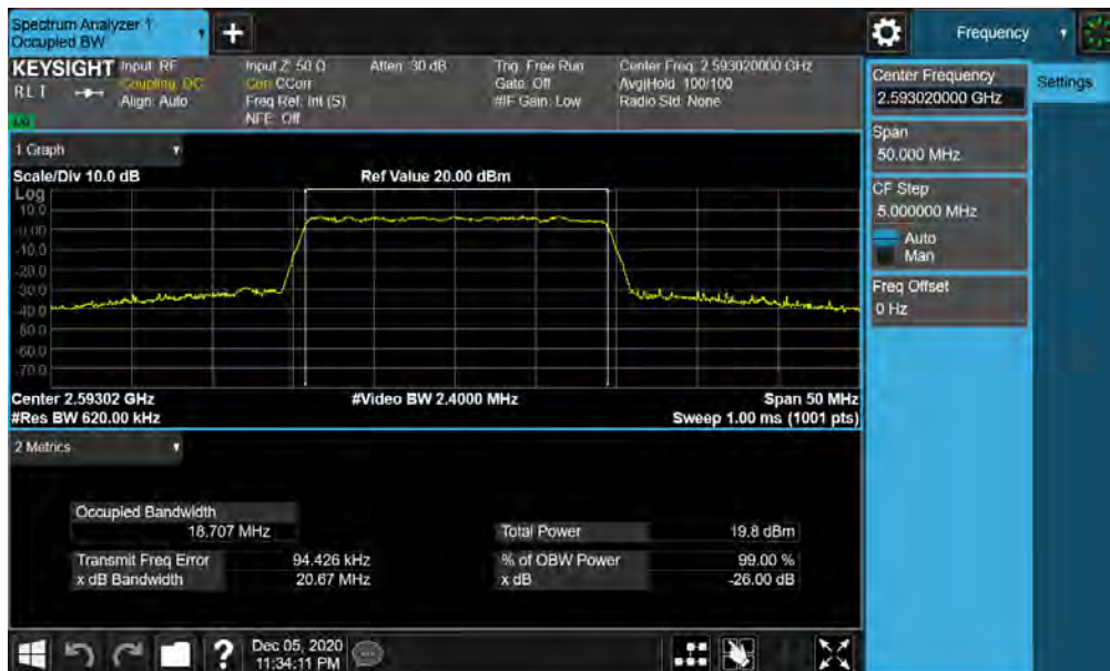
Plot 7-130. Occupied Bandwidth Plot (NR Band n41 - 20MHz CP-OFDM 256-QAM - Full RB)
