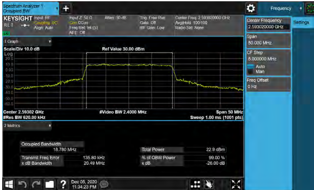
Plot 7-129. Occupied Bandwidth Plot (NR Band n41 - 20MHz CP-OFDM 64-QAM - Full RB)
