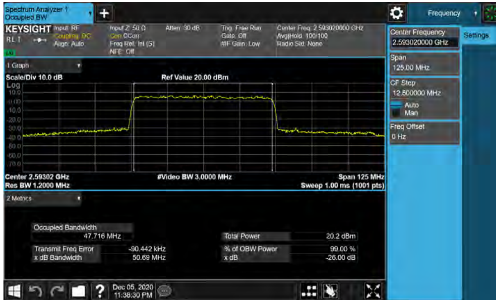
Plot 7-115. Occupied Bandwidth Plot (NR Band n41 - 50MHz CP-OFDM 256-QAM - Full RB)
