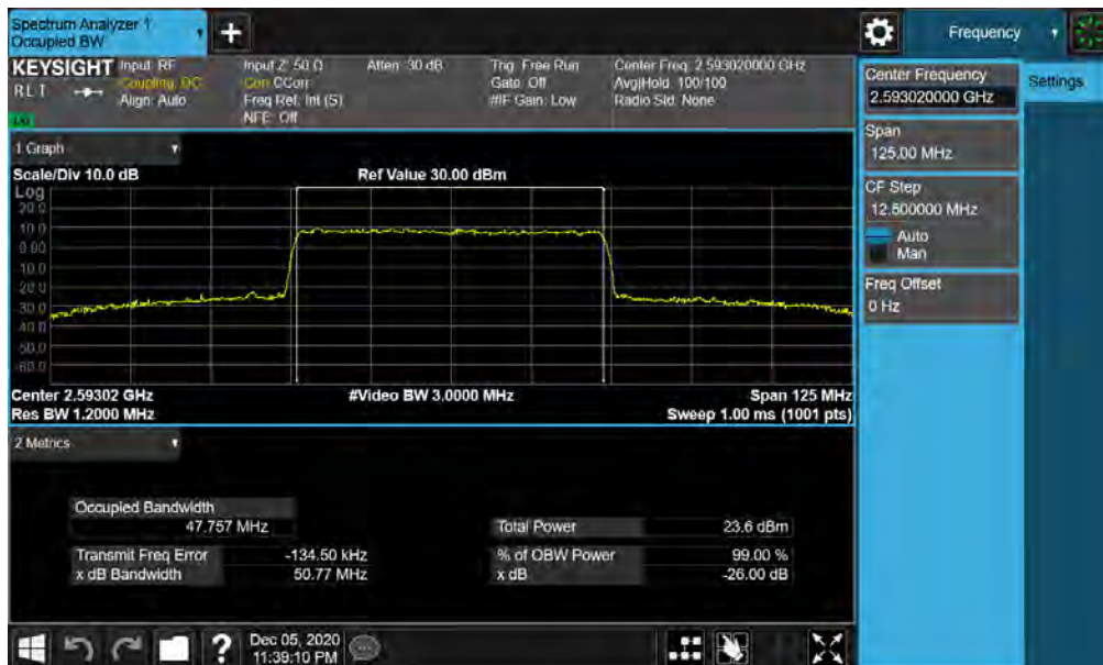
Plot 7-112. Occupied Bandwidth Plot (NR Band n41 - 50MHz CP-OFDM QPSK - Full RB)
