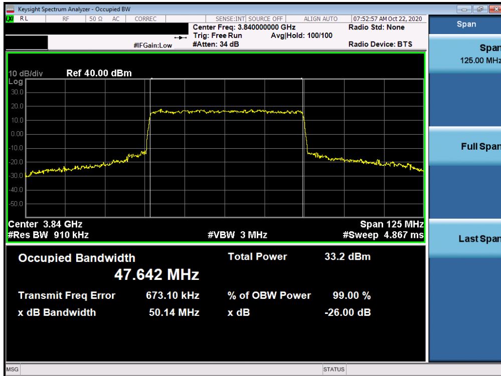
Plot 7-157. Occupied Bandwidth Plot (NR Band n77 - 50MHz CP-OFDM 16-QAM - Full RB)
