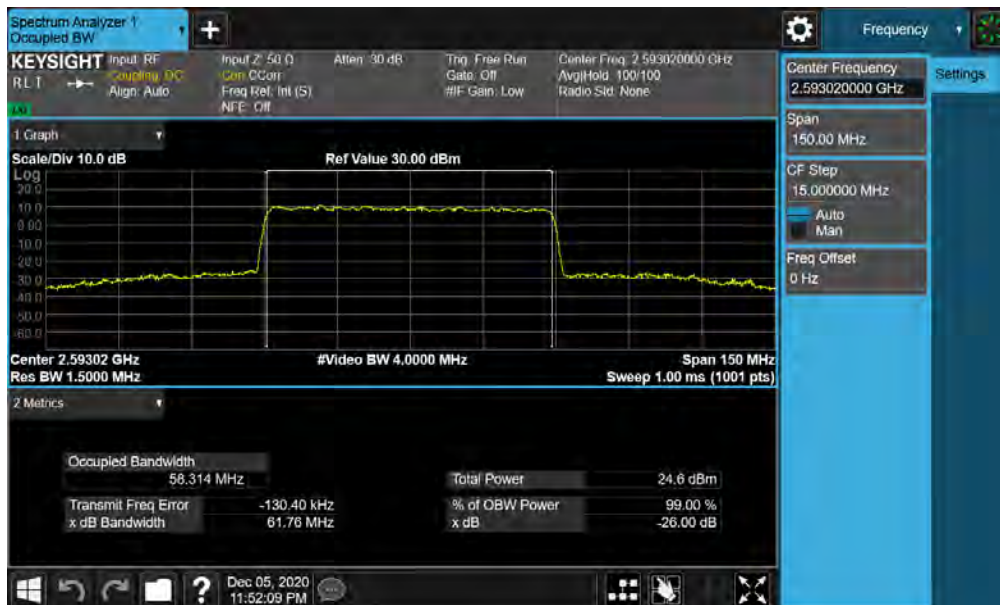
Plot 7-108. Occupied Bandwidth Plot (NR Band n41 - 60MHz CP-OFDM 16-QAM - Full RB)
