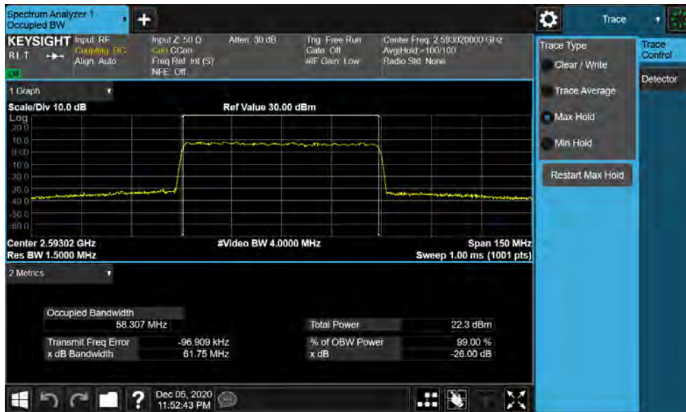
Plot 7-110. Occupied Bandwidth Plot (NR Band n41 - 60MHz CP-OFDM 256-QAM - Full RB)
