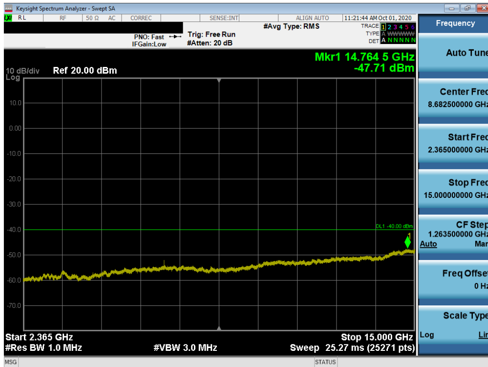
Plot 7-176. Conducted Spurious Plot (LTE Band 30 - 10MHz QPSK - RB Size 1, RB Offset 0)
