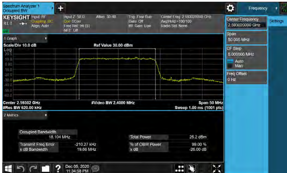
Plot 7-126. Occupied Bandwidth Plot (NR Band n41 - 20MHz \pi/2 BPSK - Full RB)
