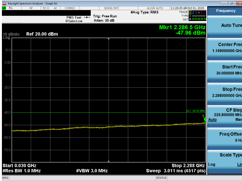
Plot 7-175. Conducted Spurious Plot (LTE Band 30 - 10MHz QPSK - RB Size 1, RB Offset 0)
