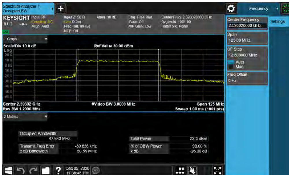
Plot 7-114. Occupied Bandwidth Plot (NR Band n41 - 50MHz CP-OFDM 64-QAM - Full RB)
