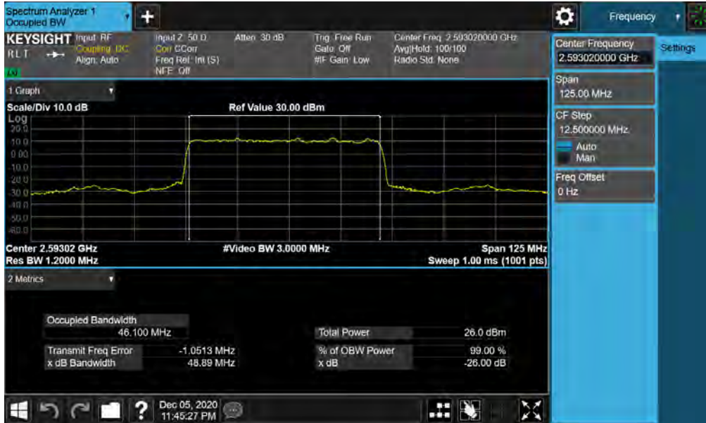
Plot 7-111. Occupied Bandwidth Plot (NR Band n41 - 50MHz \pi/2 BPSK - Full RB)
