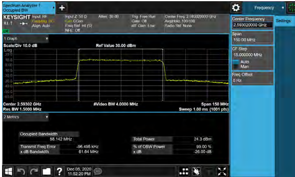
Plot 7-109. Occupied Bandwidth Plot (NR Band n41 - 60MHz CP-OFDM 64-QAM - Full RB)
