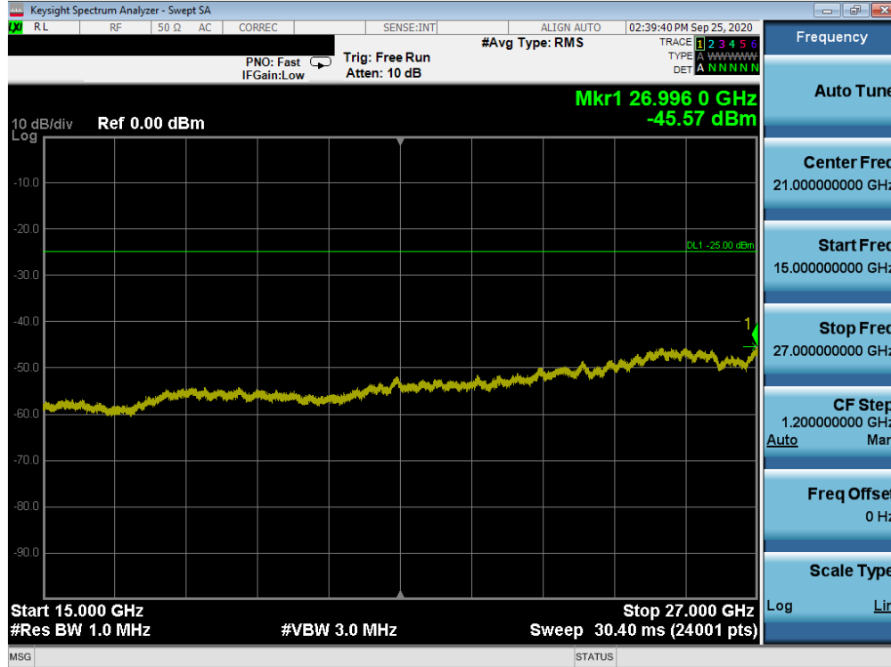
Plot 7-186. Conducted Spurious Plot (LTE Band 7 - 20MHz QPSK - RB Size 1, RB Offset 0 - High Channel)
