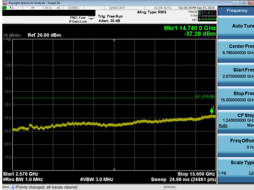
Plot 7-182. Conducted Spurious Plot (LTE Band 7 - 20MHz QPSK - RB Size 1, RB Offset 0 - Mid Channel)
