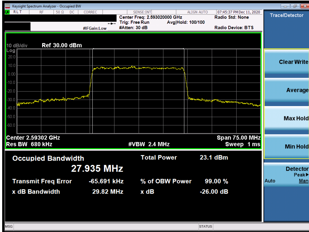
Plot 7-123. Occupied Bandwidth Plot (NR Band n41 - 30MHz CP-OFDM 16-QAM - Full RB)
