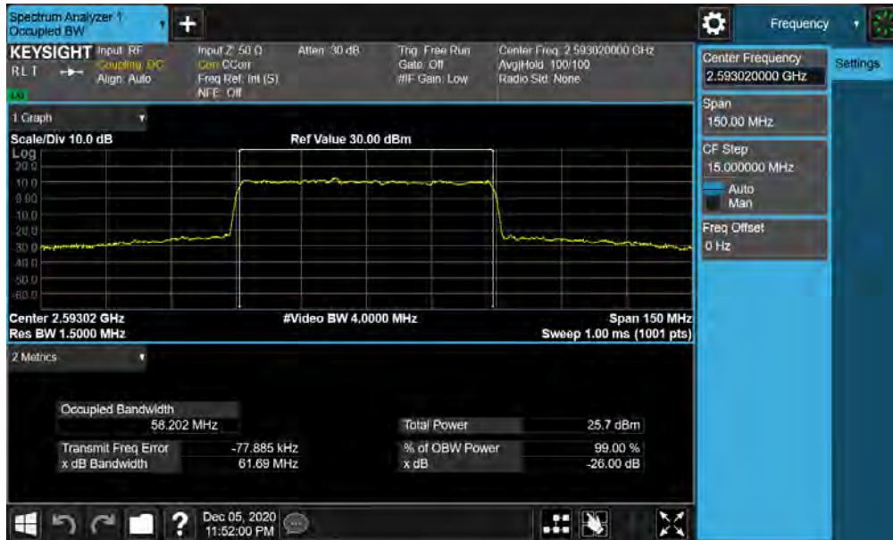
Plot 7-107. Occupied Bandwidth Plot (NR Band n41 - 60MHz CP-OFDM QPSK - Full RB)
