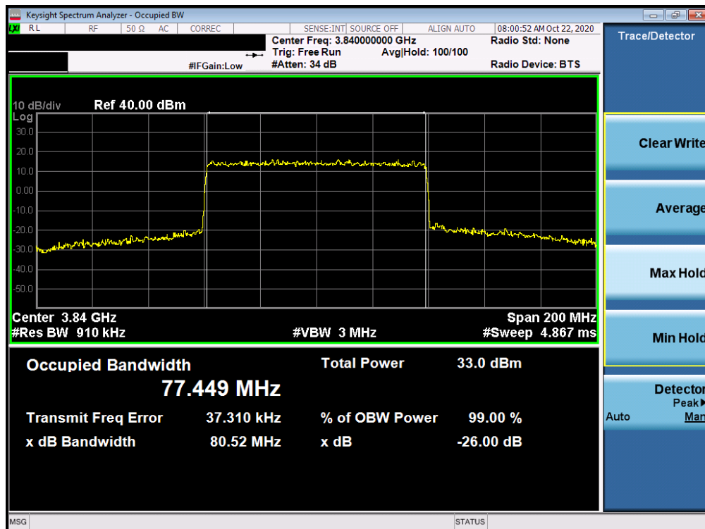
Plot 7-142. Occupied Bandwidth Plot (NR Band n77 - 80MHz CP-OFDM QPSK - Full RB)
