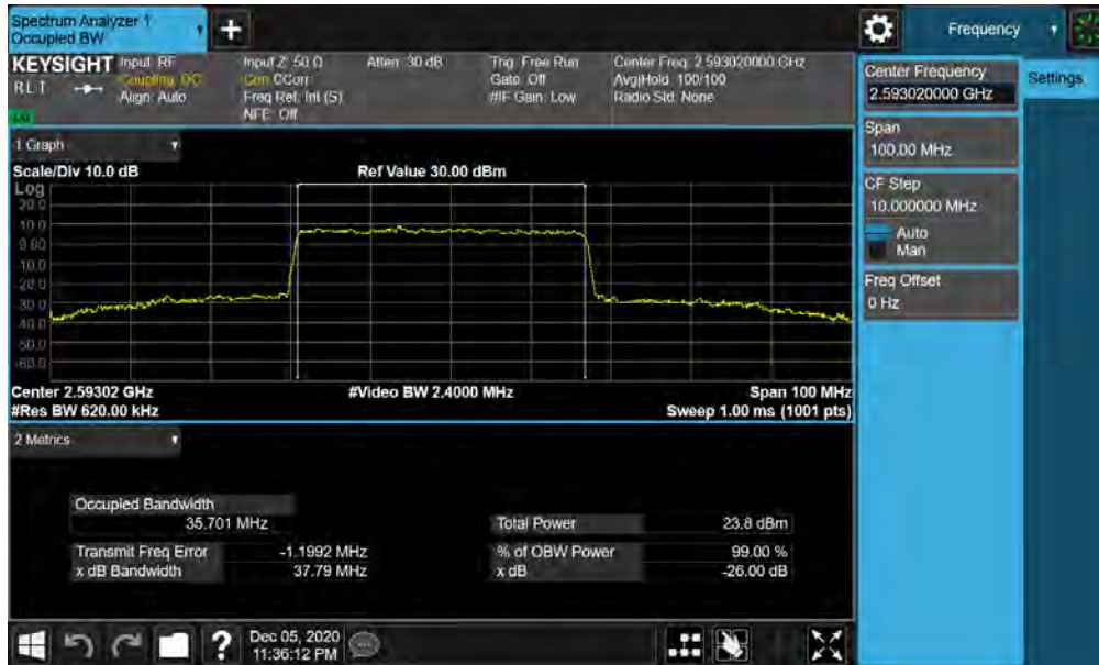
Plot 7-117. Occupied Bandwidth Plot (NR Band n41 - 40MHz CP-OFDM QPSK - Full RB)
