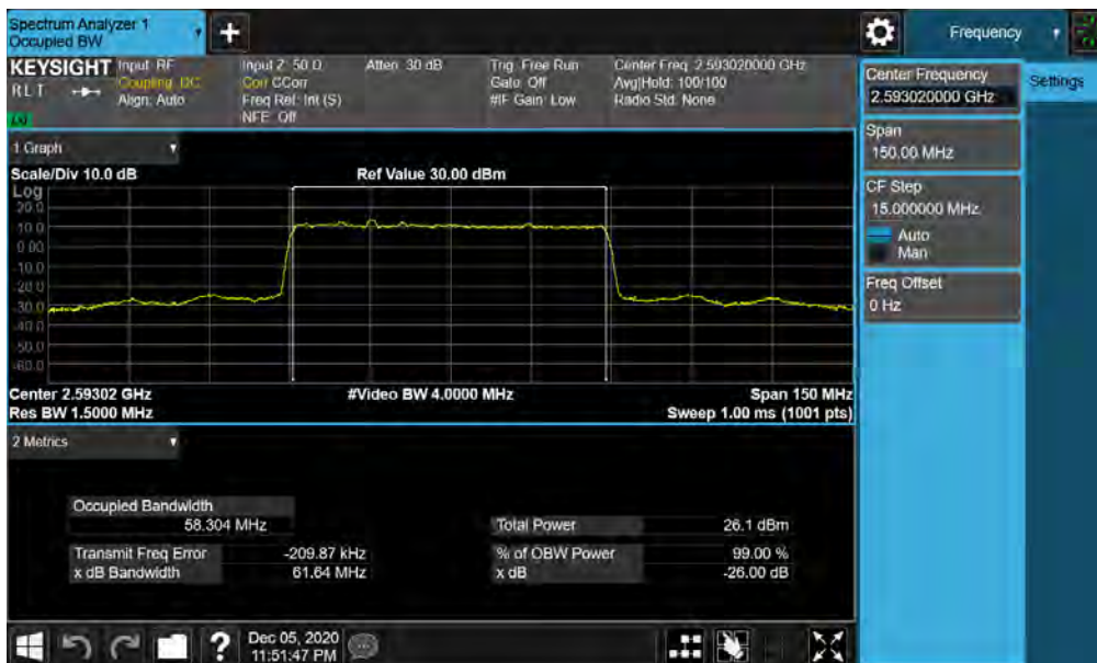
Plot 7-106. Occupied Bandwidth Plot (NR Band n41 - 60MHz \pi/2 BPSK - Full RB)
