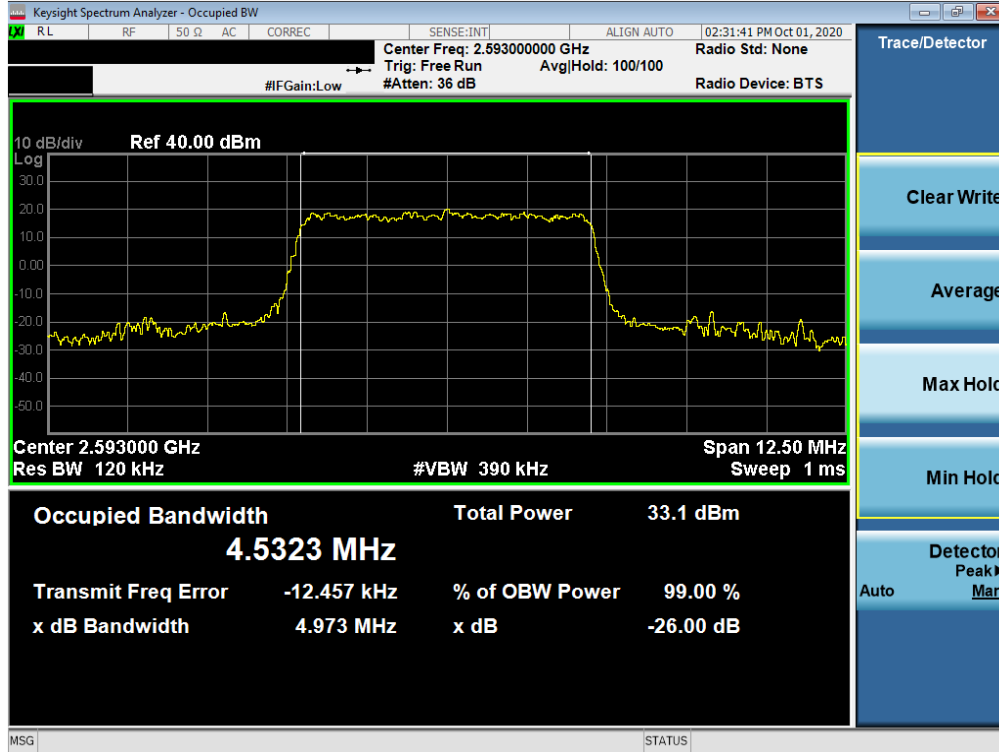
Plot 7-39. Occupied Bandwidth Plot (LTE Band 41(PC2) - 5MHz 64-QAM - Full RB Configuration)
