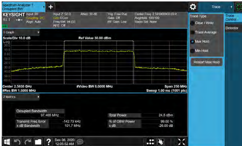
Plot 7-92. Occupied Bandwidth Plot (NR Band n41 - 100MHz CP-OFDM QPSK - Full RB)
