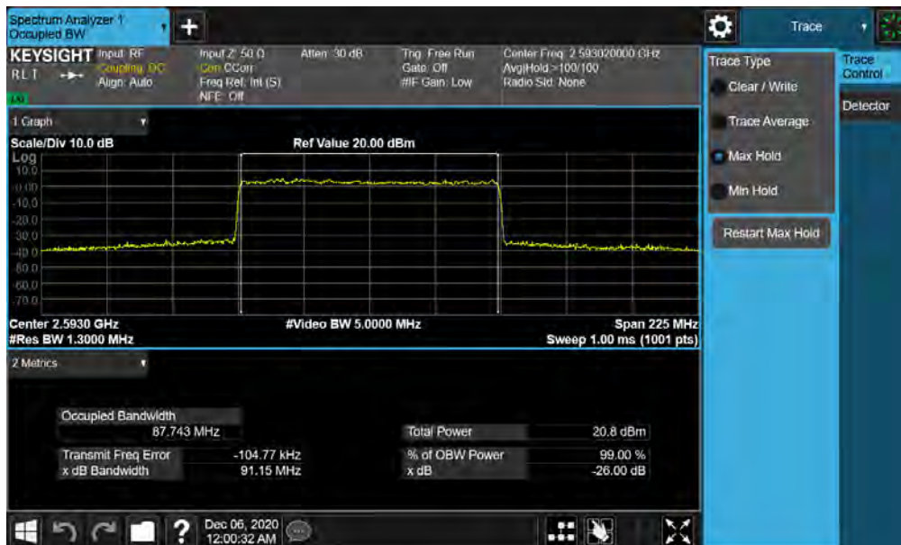
Plot 7-100. Occupied Bandwidth Plot (NR Band n41 - 90MHz CP-OFDM 256-QAM - Full RB)
