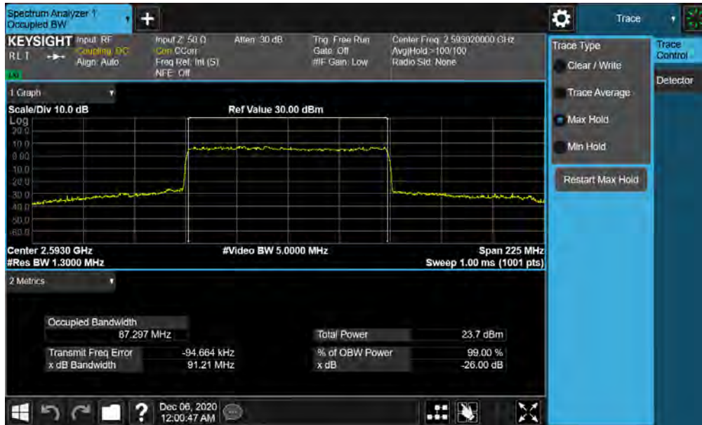
Plot 7-99. Occupied Bandwidth Plot (NR Band n41 - 90MHz CP-OFDM 64-QAM - Full RB)
