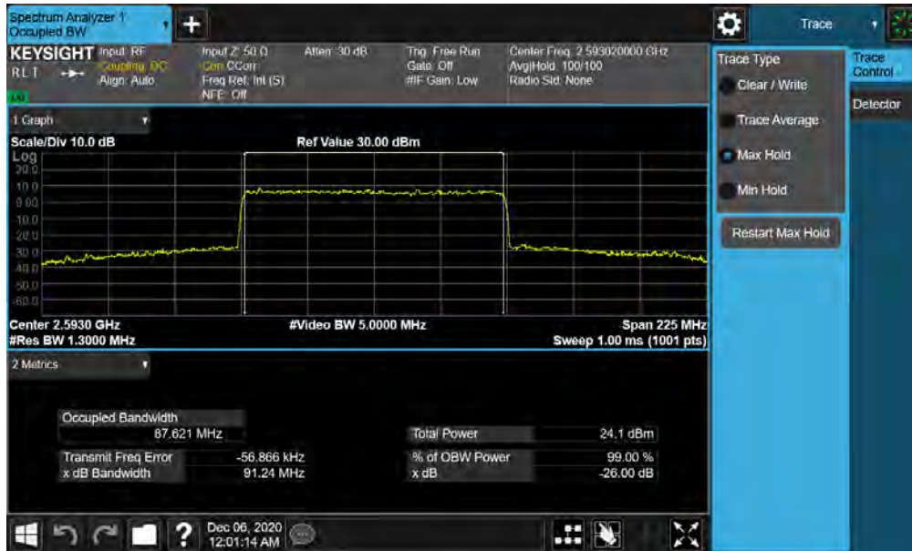
Plot 7-97. Occupied Bandwidth Plot (NR Band n41 - 90MHz CP-OFDM QPSK - Full RB)
