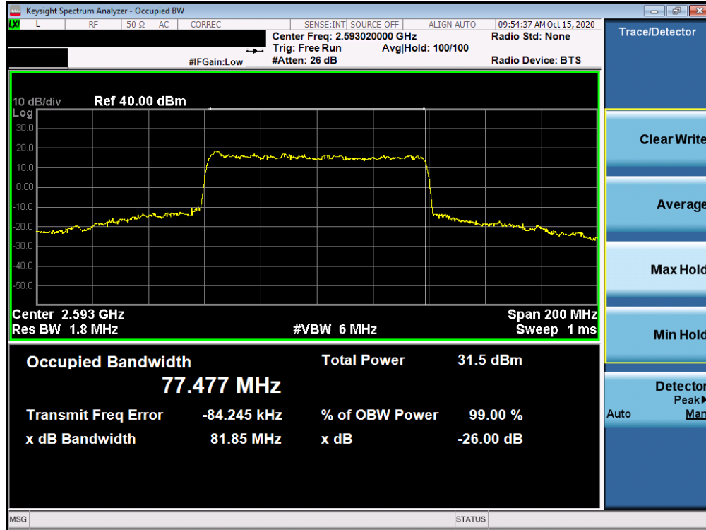
Plot 7-65. Occupied Bandwidth Plot (NR Band n41 - 80MHz CP-OFDM 256-QAM - Full RB)
