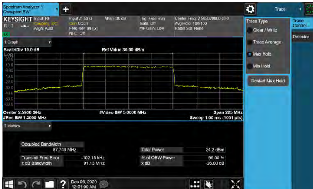
Plot 7-98. Occupied Bandwidth Plot (NR Band n41 - 90MHz CP-OFDM 16-QAM - Full RB)
