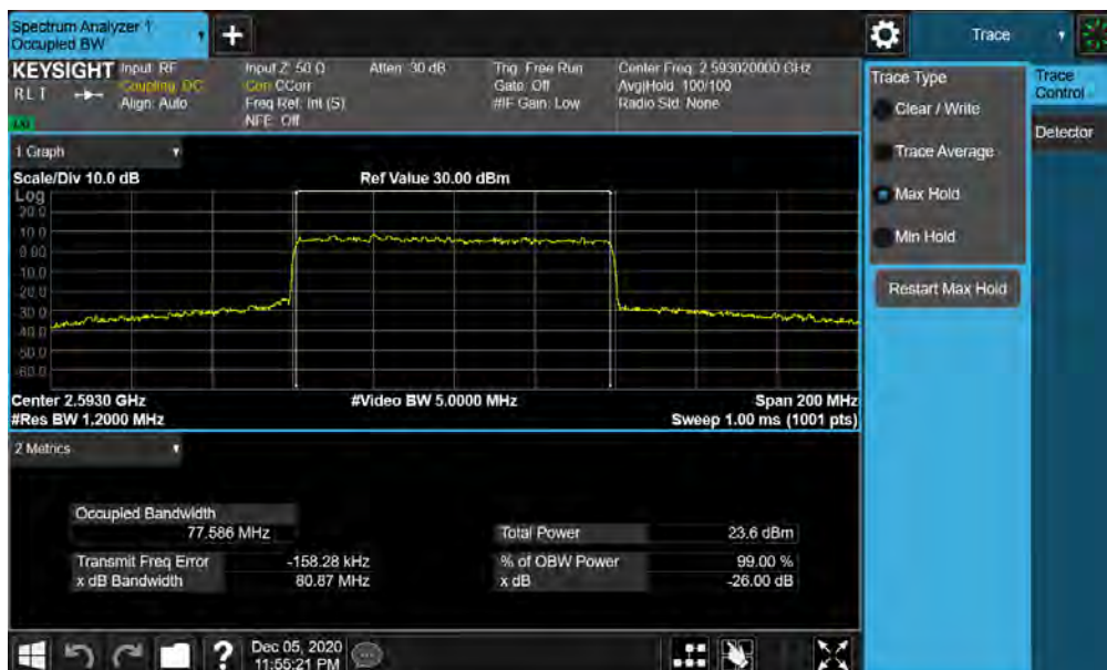
Plot 7-104. Occupied Bandwidth Plot (NR Band n41 - 80MHz CP-OFDM 64-QAM - Full RB)
