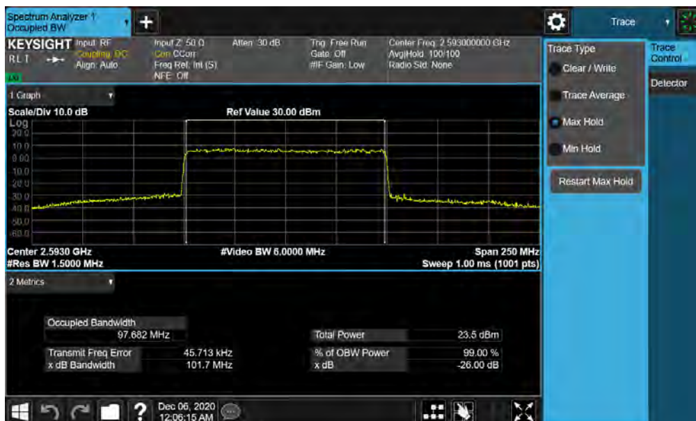
Plot 7-94. Occupied Bandwidth Plot (NR Band n41 - 100MHz CP-OFDM 64-QAM - Full RB)
