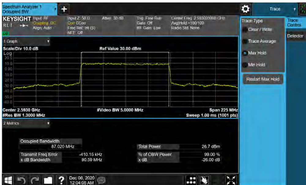
Plot 7-96. Occupied Bandwidth Plot (NR Band n41 - 90MHz \pi/2 BPSK - Full RB)
