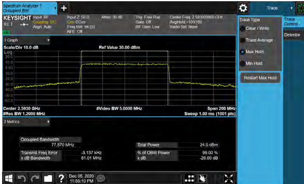
Plot 7-103. Occupied Bandwidth Plot (NR Band n41 - 80MHz CP-OFDM 16-QAM - Full RB)
