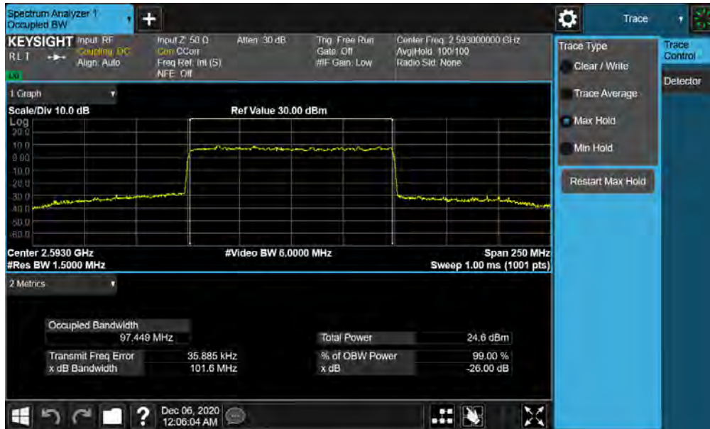
Plot 7-93. Occupied Bandwidth Plot (NR Band n41 - 100MHz CP-OFDM 16-QAM - Full RB)
