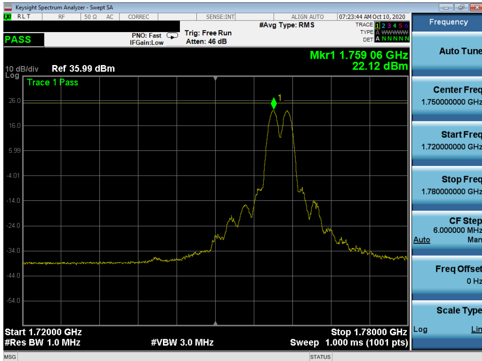
Plot 7-430. Conducted Spurious Plot (Band 66 – 20.0MHz QPSK – PCC 1/0 SCC 1/99 – High Channel)
