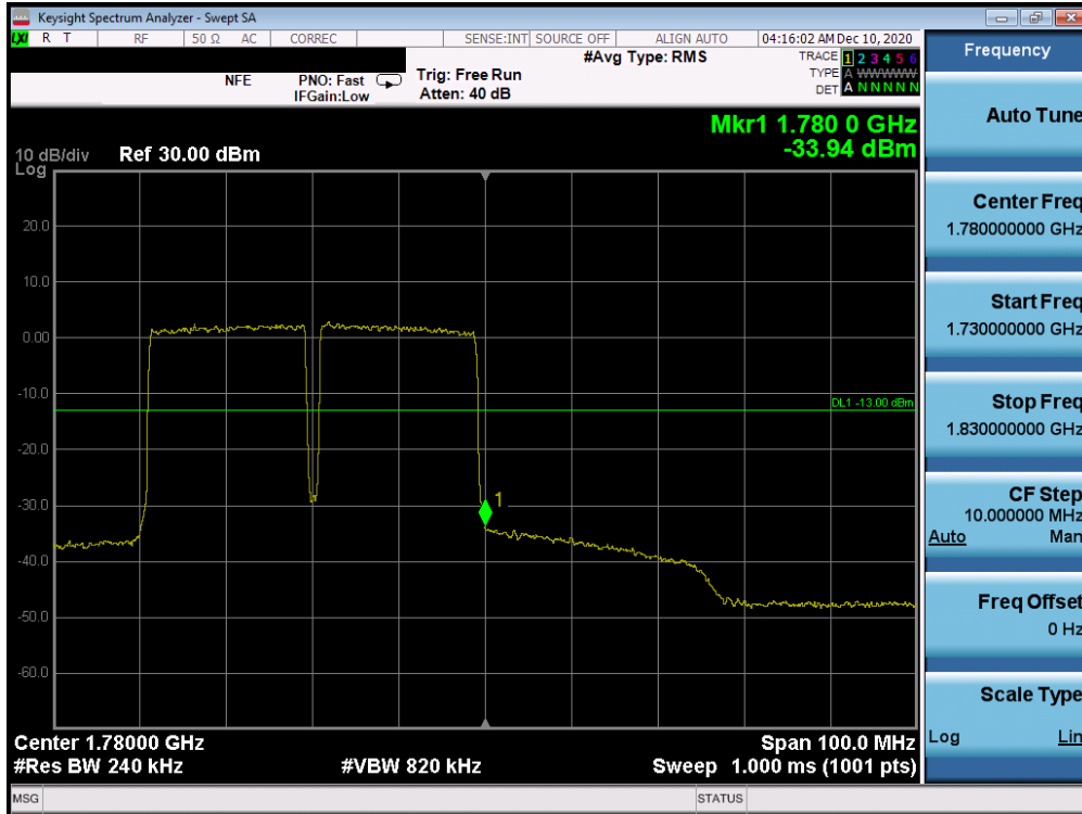
Plot 7-435. Upper Band Edge Plot (Band 66 QPSK – PCC:20 MHz SCC:20 MHz – Full RB)
