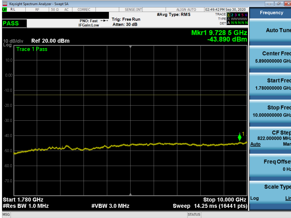
Plot 7-331. Conducted Spurious Plot (NR Band n66 - 20.0MHz - RB Size 1, RB Offset 0 - Mid Channel)
