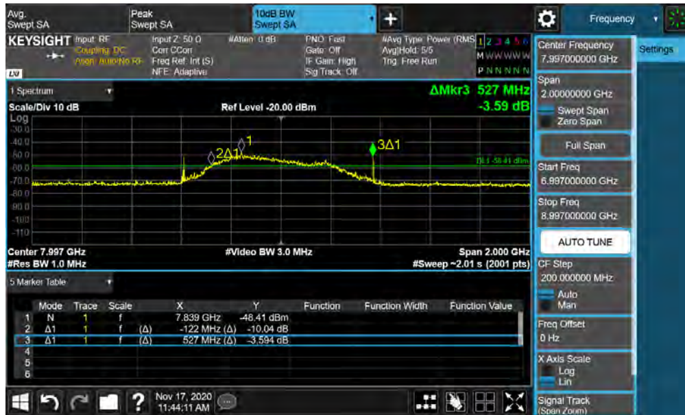
Plot 7-20. BANDWIDTH Plot – ANT1 - CH.9 – SP1 – Preamble 12
