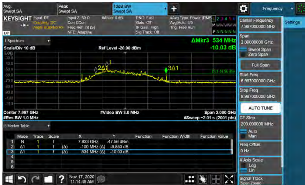
Plot 7-8. BANDWIDTH Plot – ANT1 - CH.9 – SP1 – Preamble 10
