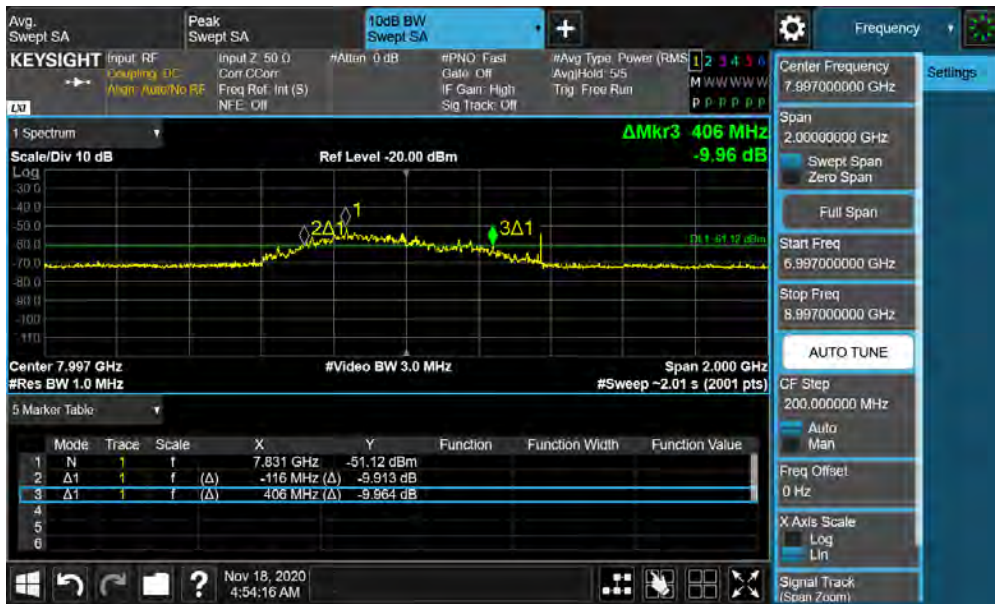
Plot 7-4. BANDWIDTH Plot – ANT2 - CH.9 - SP0 – Preamble 9
