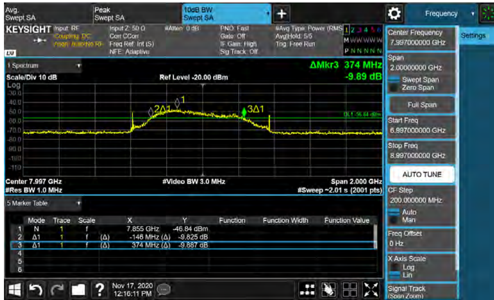
Plot 7-31. BANDWIDTH Plot – ANT1 - CH.9 - SP0 – Preamble 26
