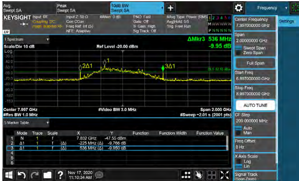
Plot 7-7. BANDWIDTH Plot – ANT1 - CH.9 - SP0 – Preamble 10
