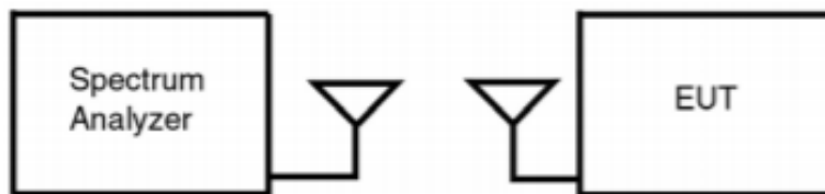
Figure 7-1. Test Instrument and Measurement Setup
