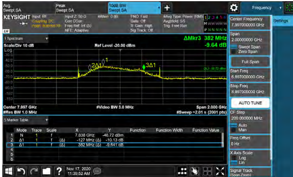
Plot 7-19. BANDWIDTH Plot – ANT1 - CH.9 - SP0 – Preamble 12
