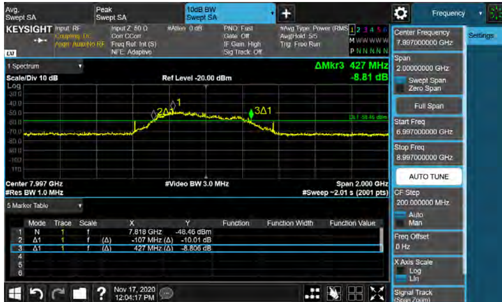
Plot 7-26. BANDWIDTH Plot – ANT1 - CH.9 – SP1 – Preamble 25
