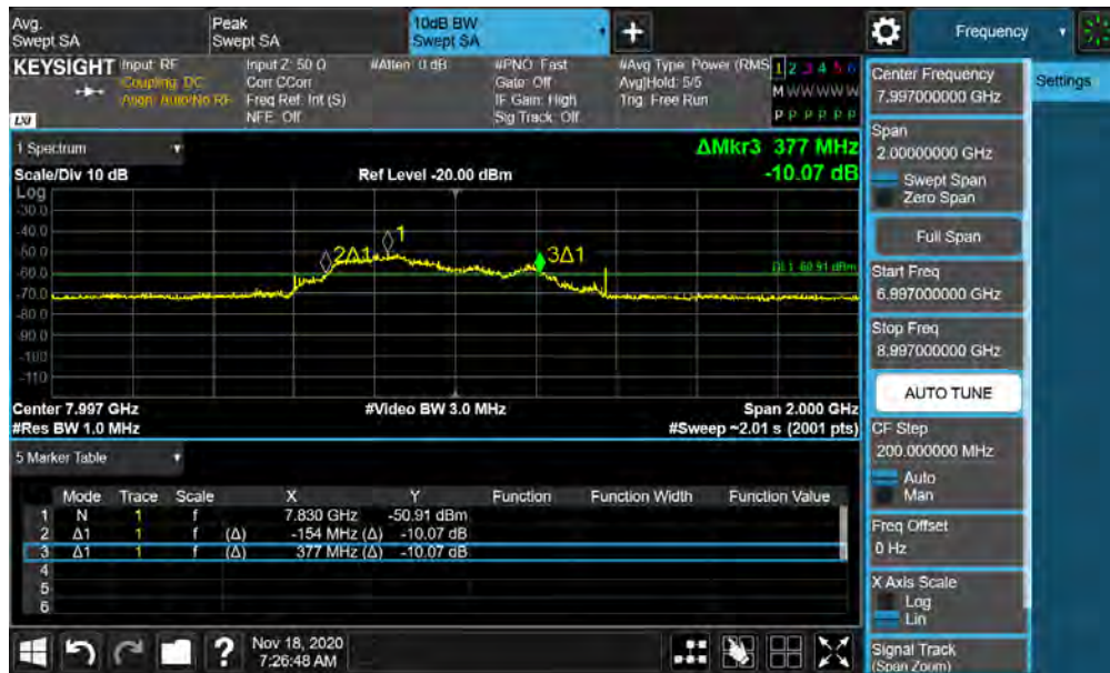
Plot 7-66. BANDWIDTH Plot – ANT2 - CH.9 – SP3 – Preamble 31
