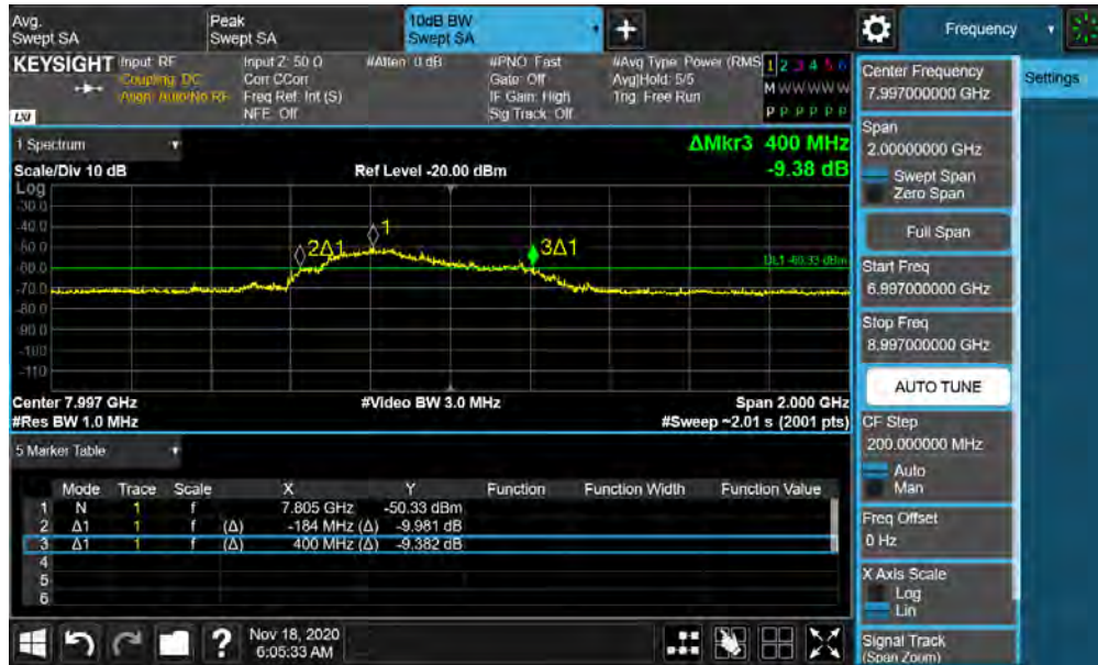
Plot 7-29. BANDWIDTH Plot – ANT2 - CH.9 – SP1 – Preamble 25
