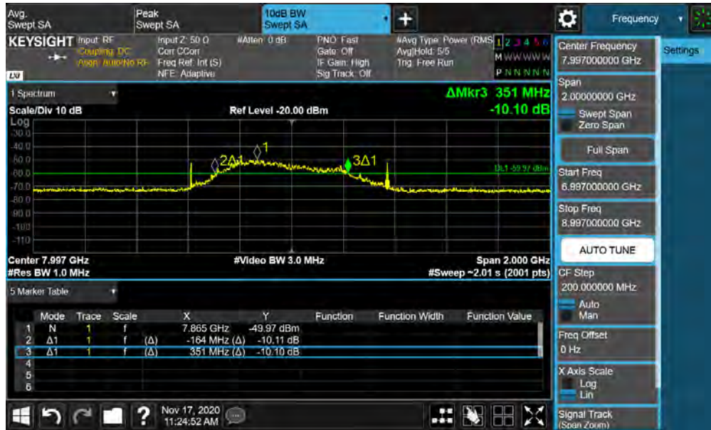
Plot 7-13. BANDWIDTH Plot – ANT1 - CH.9 - SP0 – Preamble 11
