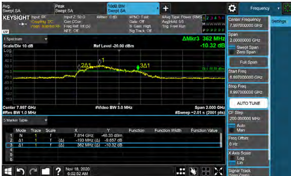
Plot 7-28. BANDWIDTH Plot – ANT2 - CH.9 - SP0 – Preamble 25
