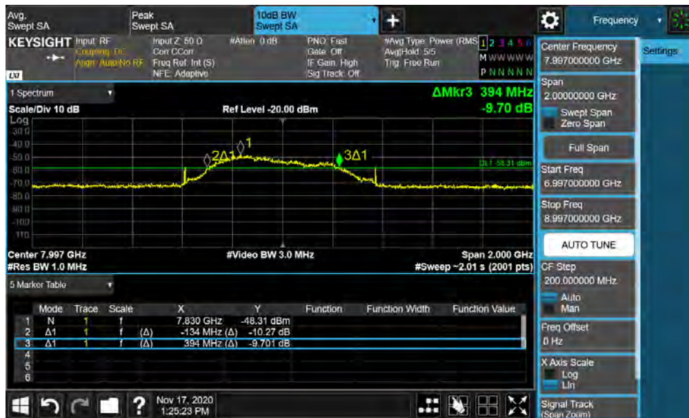
Plot 7-62. BANDWIDTH Plot – ANT1 - CH.9 – SP1 – Preamble 31
