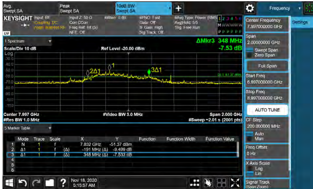
Plot 7-11. BANDWIDTH Plot – ANT2 - CH.9 – SP1 – Preamble 10
