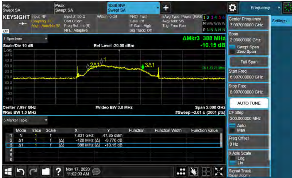
Plot 7-3. BANDWIDTH Plot – ANT1 - CH.9 – SP3 – Preamble 9
