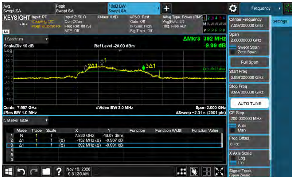
Plot 7-42. BANDWIDTH Plot – ANT2 - CH.9 – SP3 – Preamble 27
