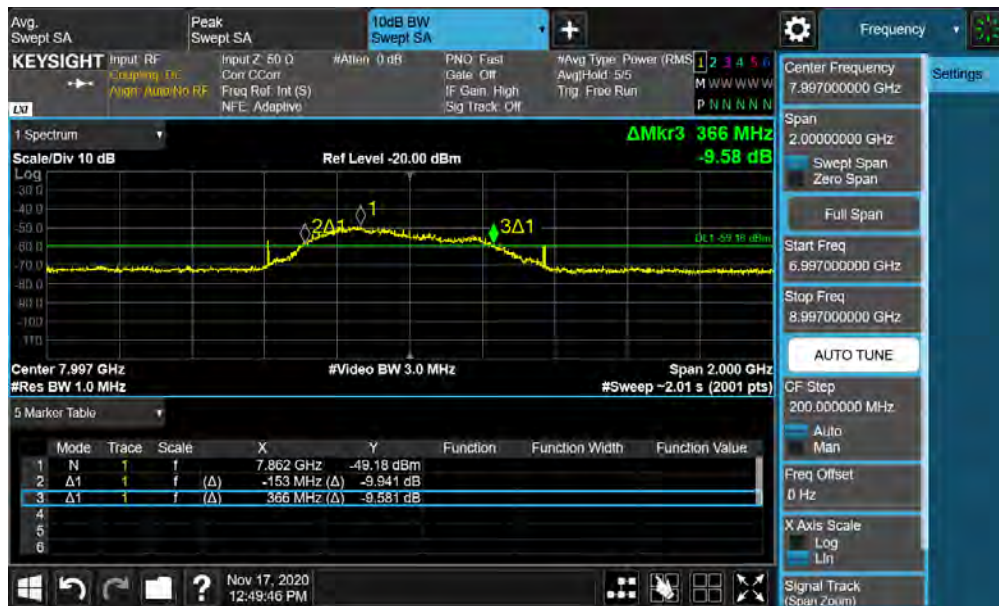
Plot 7-44. BANDWIDTH Plot – ANT1 - CH.9 – SP1 – Preamble 28
