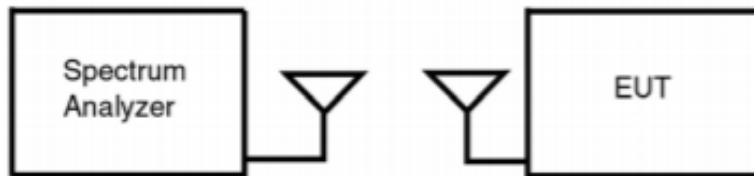
Figure 7-2. Test Instrument and Measurement Setup
