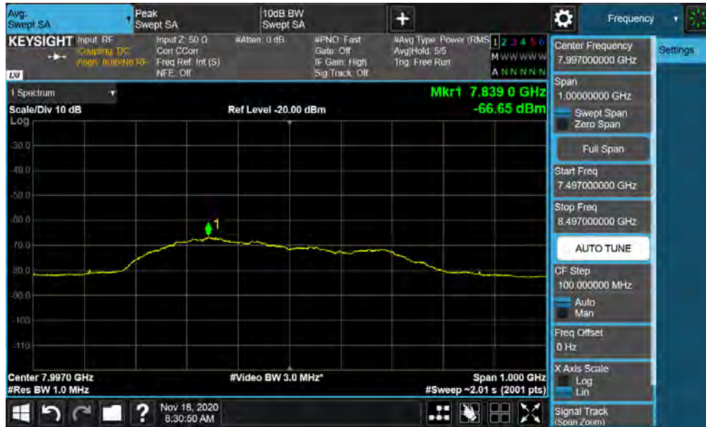
Plot 7-75. UWB Average Power Measurement - ANT 1 - CH.9 – SP3 - BPRF
