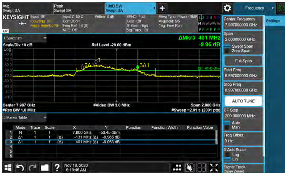
Plot 7-36. BANDWIDTH Plot – ANT2 - CH.9 – SP3 – Preamble 26
