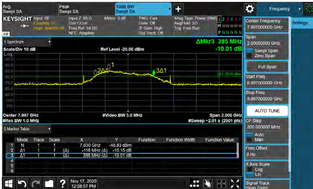
Plot 7-50. BANDWIDTH Plot – ANT1 - CH.9 – SP1 – Preamble 29
