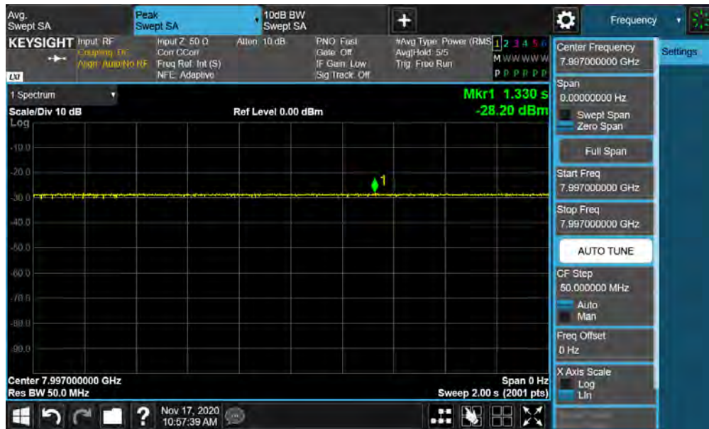
Plot 7-74. UWB Peak Power Measurement - ANT 1 - CH.9 – SP1 – BPRF
