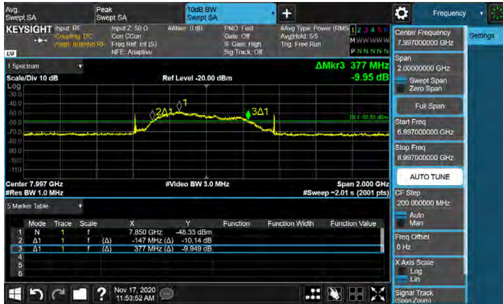
Plot 7-21. BANDWIDTH Plot – ANT1 - CH.9 – SP3 – Preamble 12
