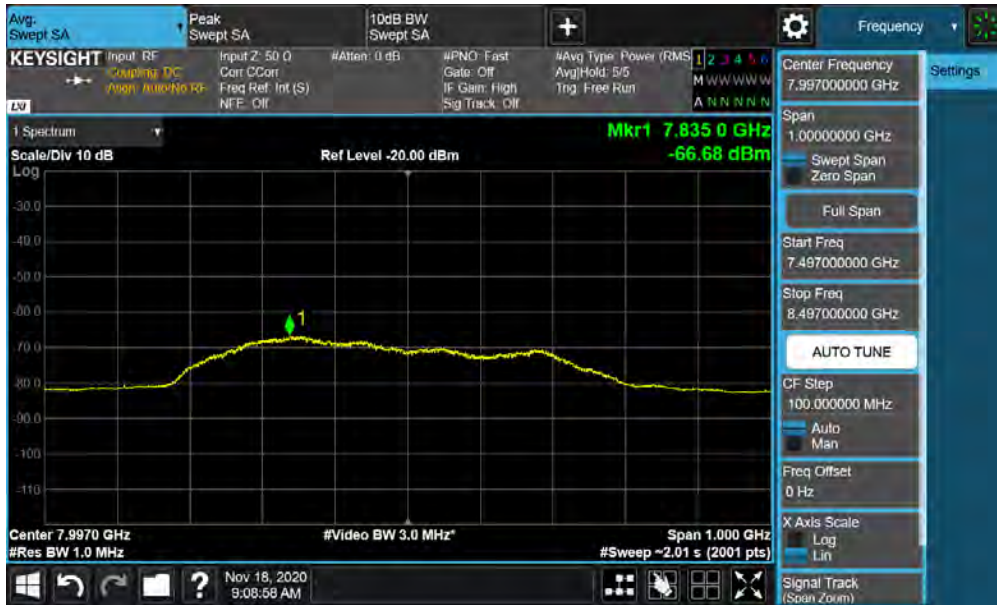
Plot 7-79. UWB Average Power Measurement - ANT 1 - CH.9 – SP3 - BPRF
