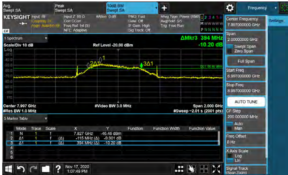
Plot 7-55. BANDWIDTH Plot – ANT1 - CH.9 - SP0 – Preamble 30
