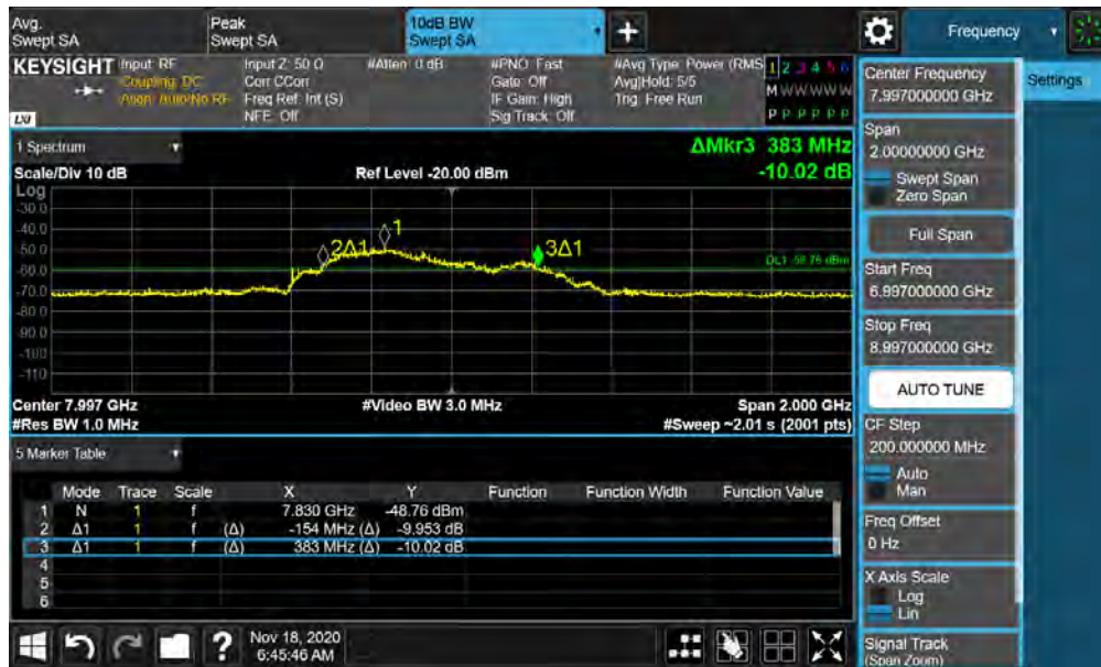
Plot 7-48. BANDWIDTH Plot – ANT2 - CH.9 – SP3 – Preamble 28
