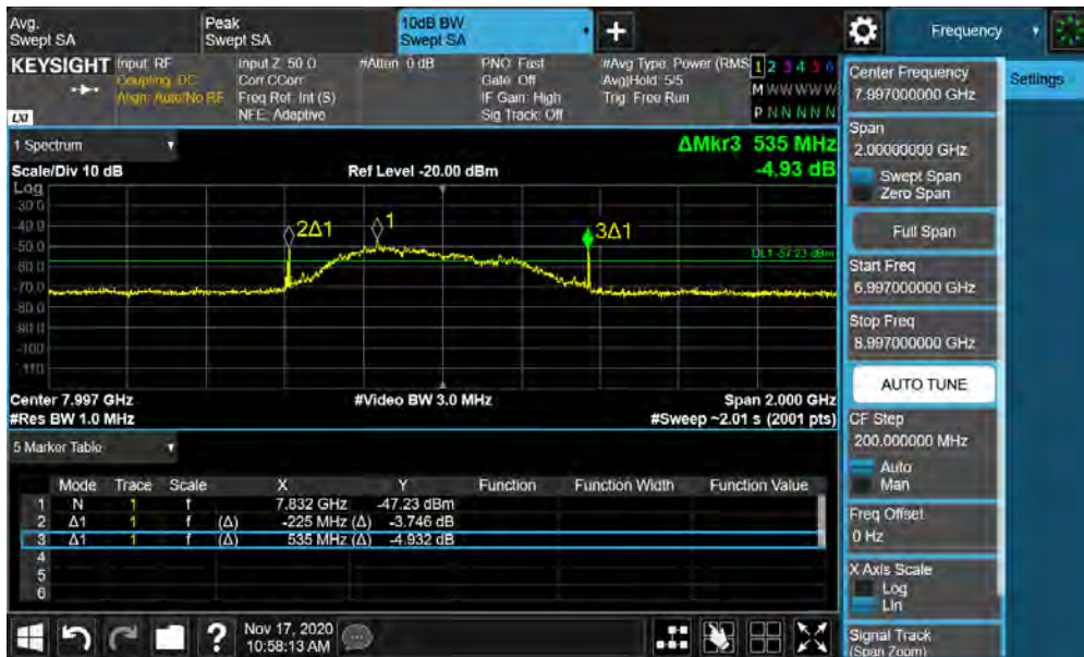
Plot 7-2. BANDWIDTH Plot – ANT1 - CH.9 – SP1 – Preamble 9
