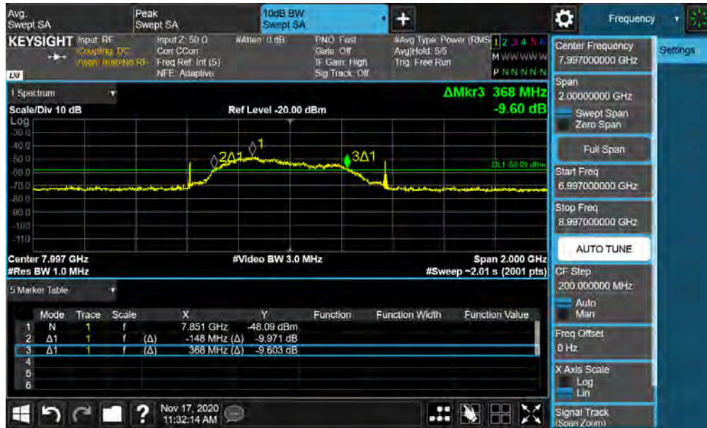
Plot 7-15. BANDWIDTH Plot – ANT1 - CH.9 – SP3 – Preamble 11
