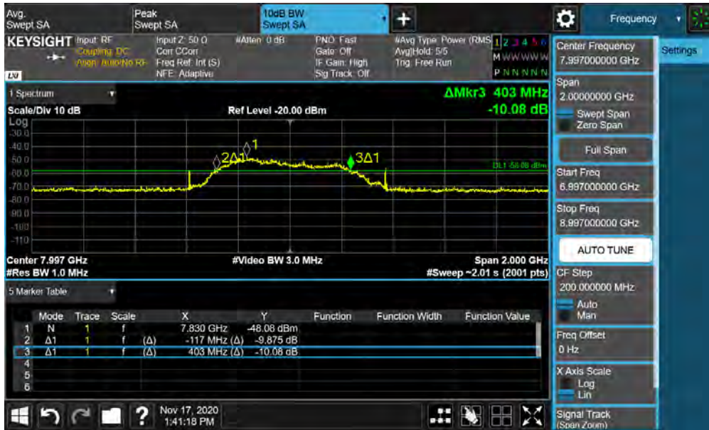
Plot 7-69. BANDWIDTH Plot – ANT1 - CH.9 – SP3 – Preamble 32
