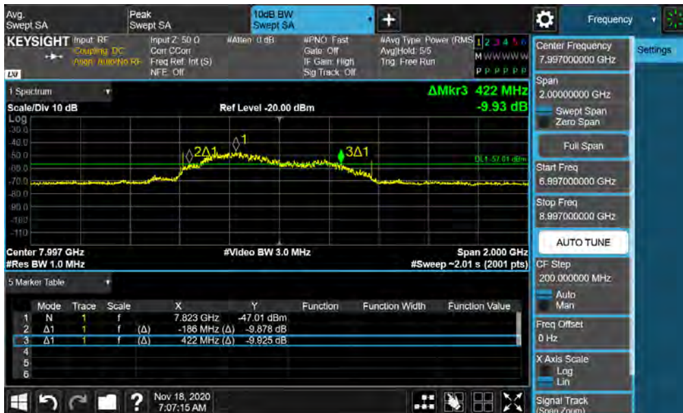
Plot 7-58. BANDWIDTH Plot – ANT2 - CH.9 - SP0 – Preamble 30
