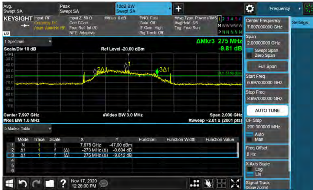
Plot 7-37. BANDWIDTH Plot – ANT1 - CH.9 - SP0 – Preamble 27
