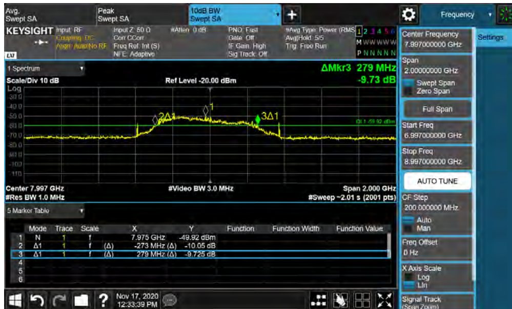
Plot 7-38. BANDWIDTH Plot – ANT1 - CH.9 – SP1 – Preamble 27
