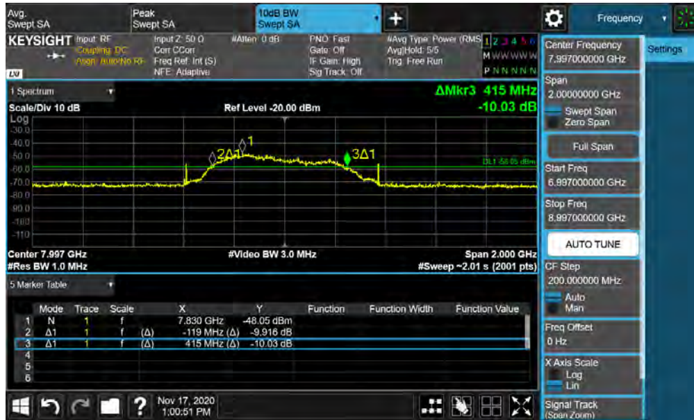
Plot 7-51. BANDWIDTH Plot – ANT1 - CH.9 – SP3 – Preamble 29
