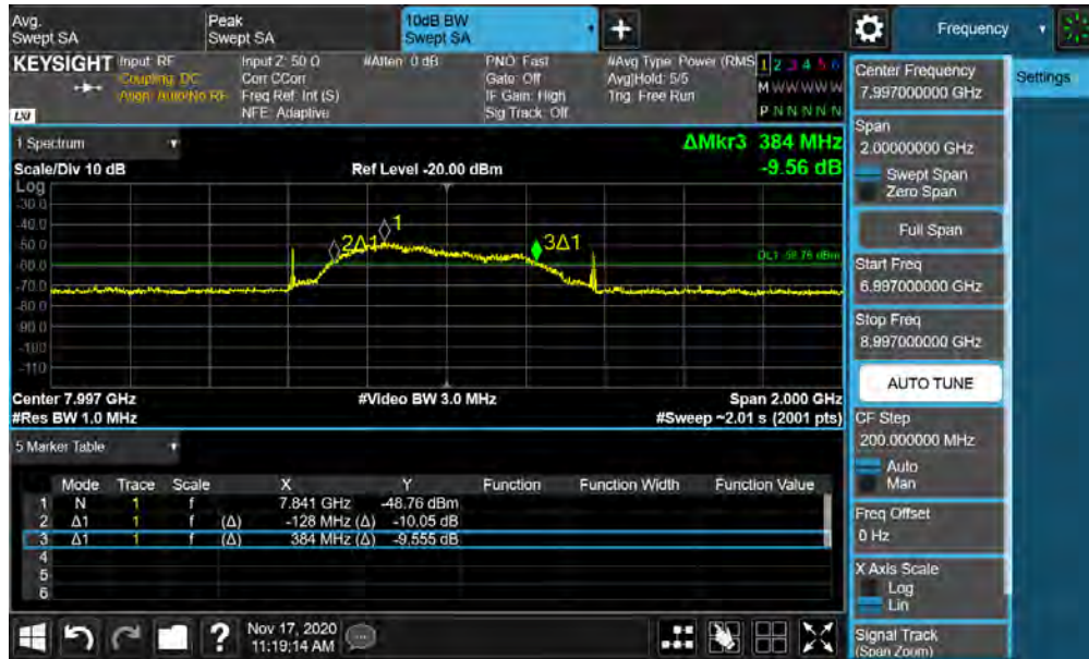
Plot 7-9. BANDWIDTH Plot – ANT1 - CH.9 – SP3 – Preamble 10
