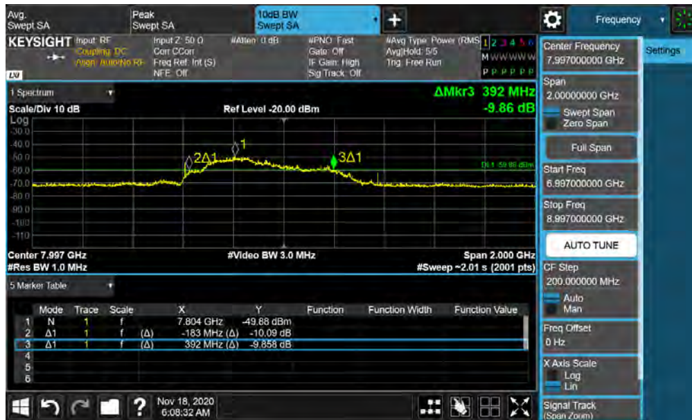
Plot 7-30. BANDWIDTH Plot – ANT2 - CH.9 – SP3 – Preamble 25
