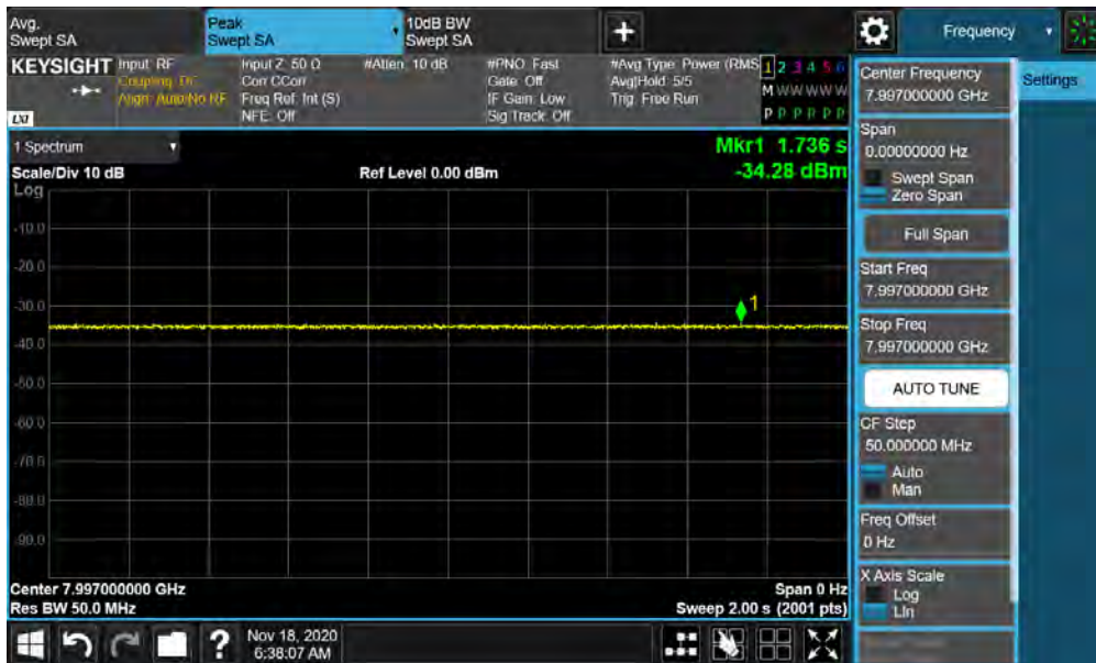
Plot 7-80. UWB Peak Power Measurement - ANT 2 - CH.9 – SP0 – BPRF
