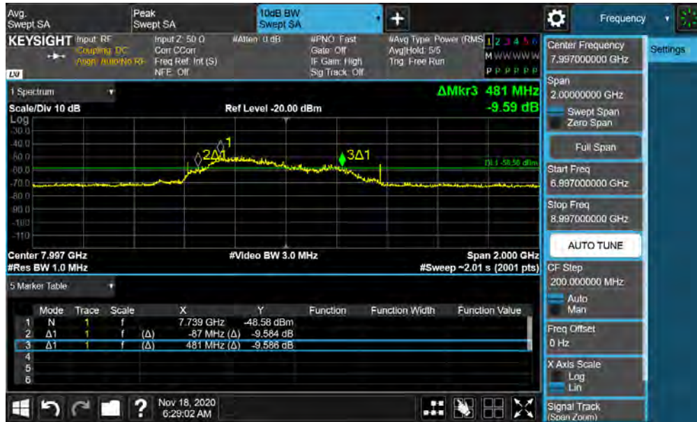
Plot 7-41. BANDWIDTH Plot – ANT2 - CH.9 – SP1 – Preamble 27
