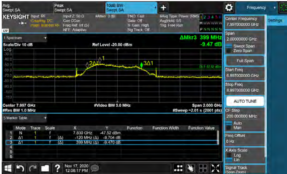
Plot 7-27. BANDWIDTH Plot – ANT1 - CH.9 – SP3 – Preamble 25
