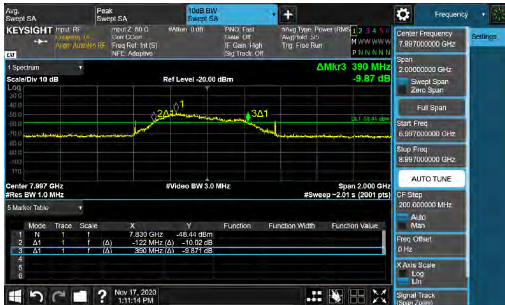
Plot 7-56. BANDWIDTH Plot – ANT1 - CH.9 – SP1 – Preamble 30
