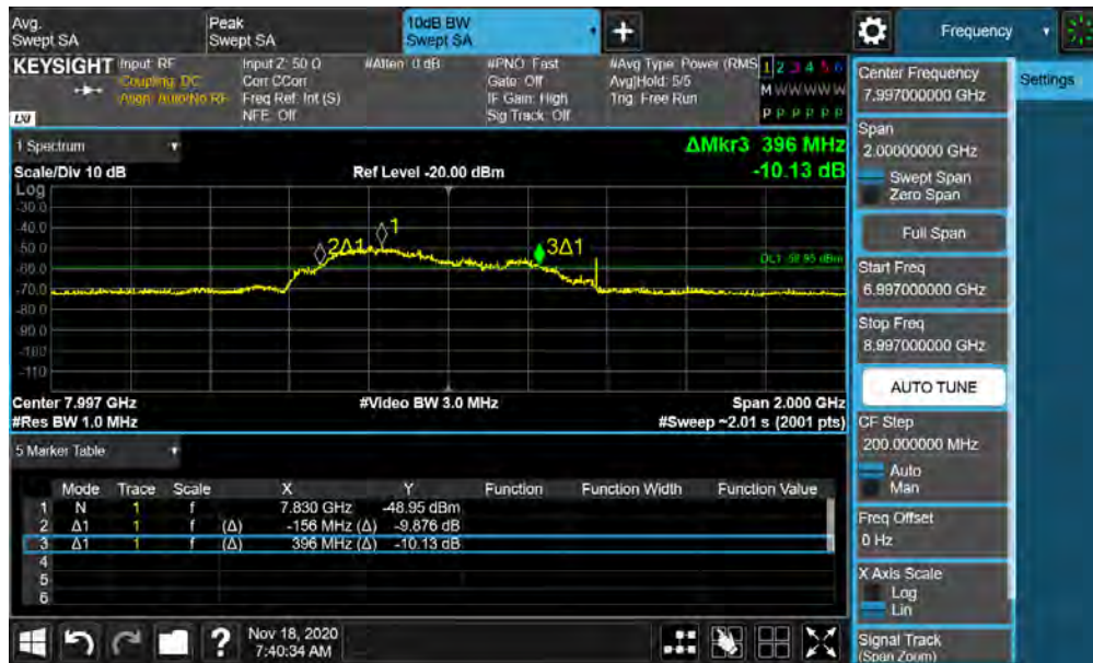
Plot 7-72. BANDWIDTH Plot – ANT2 - CH.9 – SP3 – Preamble 32
