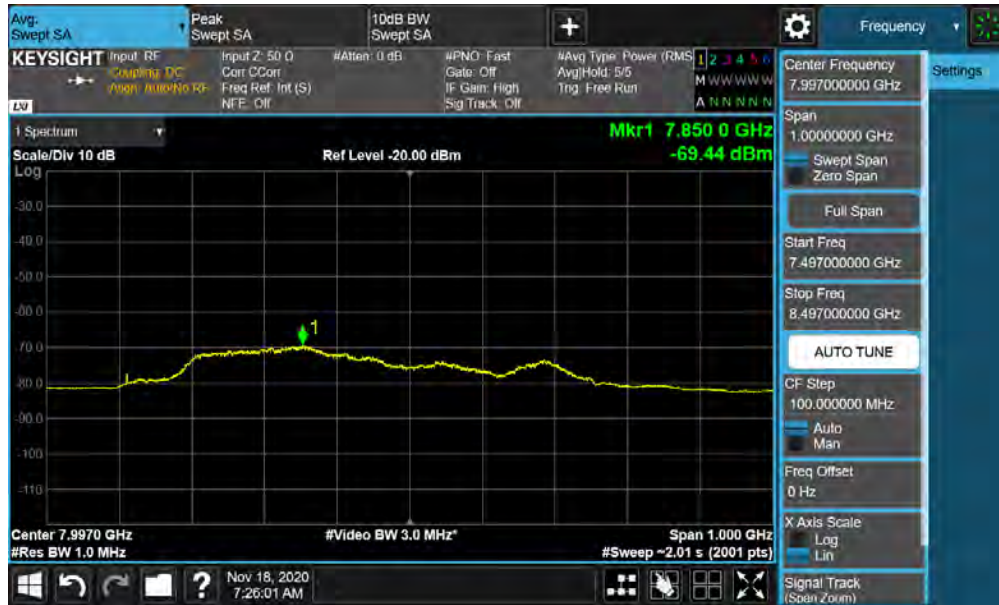
Plot 7-81. UWB Average Power Measurement - ANT 2 - CH.9 – SP3 - BPRF
