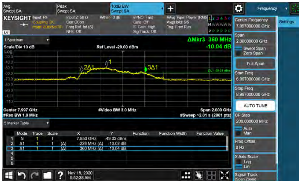
Plot 7-24. BANDWIDTH Plot – ANT2 - CH.9 – SP3 – Preamble 12
