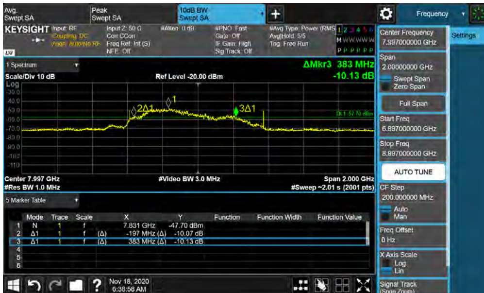
Plot 7-46. BANDWIDTH Plot – ANT2 - CH.9 - SP0 – Preamble 28
