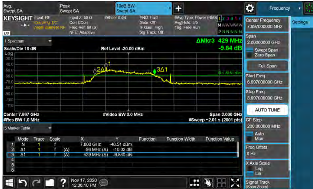
Plot 7-39. BANDWIDTH Plot – ANT1 - CH.9 – SP3 – Preamble 27
