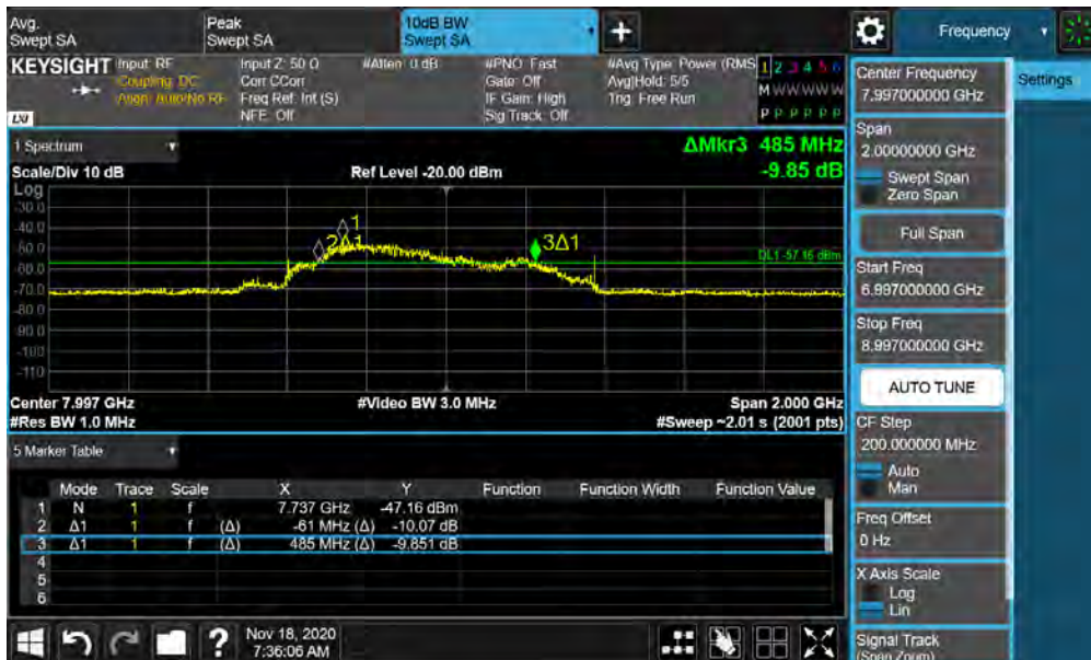
Plot 7-70. BANDWIDTH Plot – ANT2 - CH.9 - SP0 – Preamble 32
