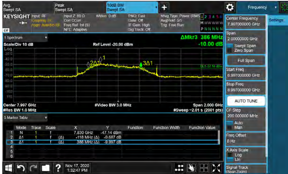
Plot 7-67. BANDWIDTH Plot – ANT1 - CH.9 - SP0 – Preamble 32
