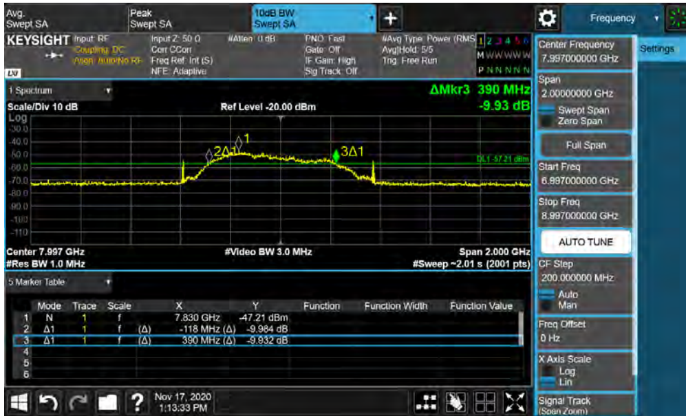
Plot 7-57. BANDWIDTH Plot – ANT1 - CH.9 – SP3 – Preamble 30
