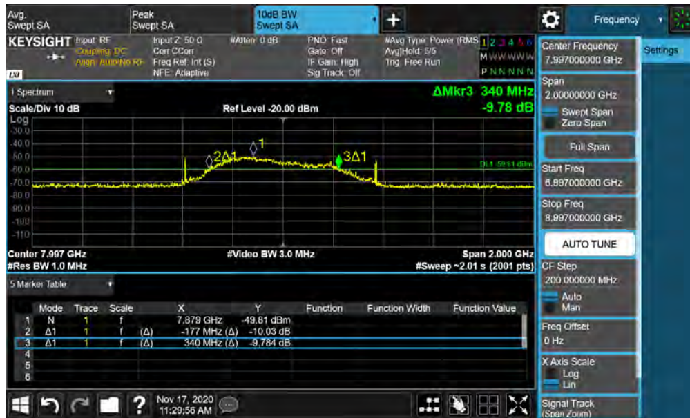
Plot 7-14. BANDWIDTH Plot – ANT1 - CH.9 – SP1 – Preamble 11
