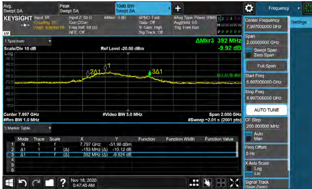
Plot 7-23. BANDWIDTH Plot – ANT2 - CH.9 – SP1 – Preamble 12
