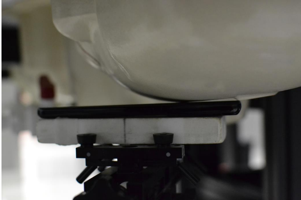
SAR Test Setup Photo 3 – Left Cheek
