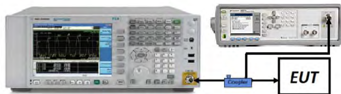
Figure 7-7. Test Instrument & Measurement Setup
