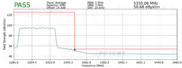
Plot 7-303. Radiated Upper Band Edge Plot MIMO (Average – UNII Band 2A) – WCP
