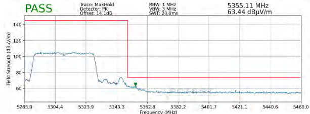
Plot 7-304. Radiated Upper Band Edge Plot MIMO (Peak – UNII Band 2A) – WCP
