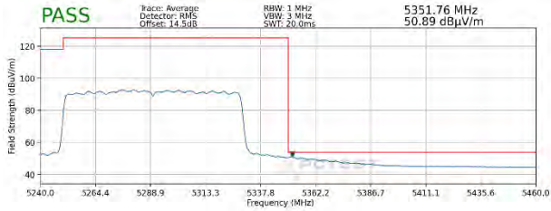
Plot 7-312. Radiated Lower Band Edge Plot MIMO (Average – UNII Band 2C) – WCP
