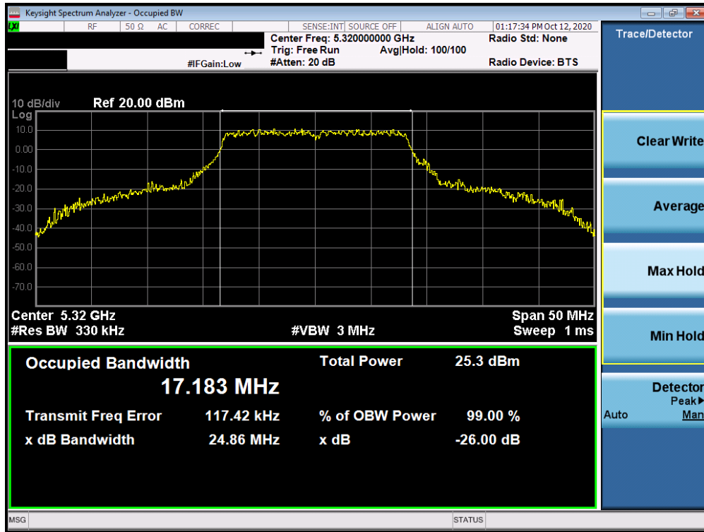
Plot 7-75. 26dB Bandwidth Plot MIMO ANT2 (802.11a (UNII Band 2A) – Ch. 64)
