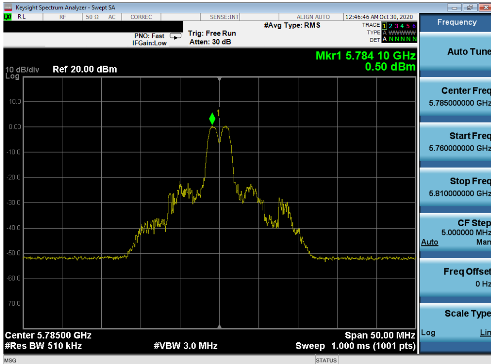
Plot 7-185. Power Spectral Density Plot MIMO ANT2 (20MHz BW 802.11ax – 26 Tones (UNII Band 3) – Ch. 157)
