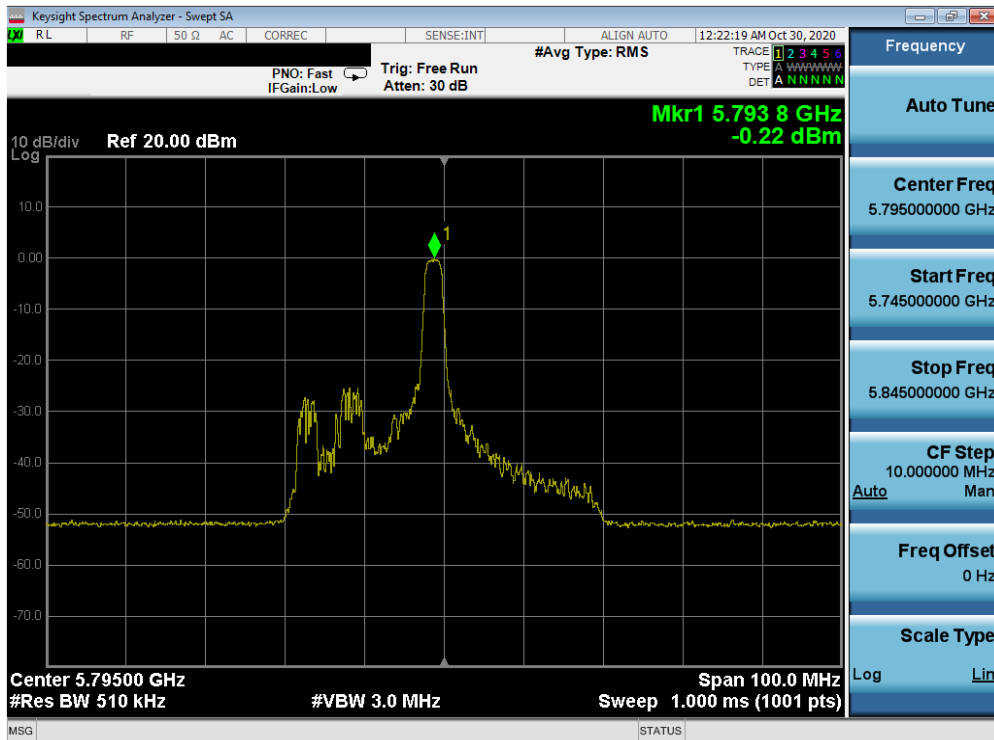
Plot 7-134. Power Spectral Density Plot MIMO ANT1 (40MHz BW 802.11ax – 26 Tones (UNII Band 3) – Ch. 159)
