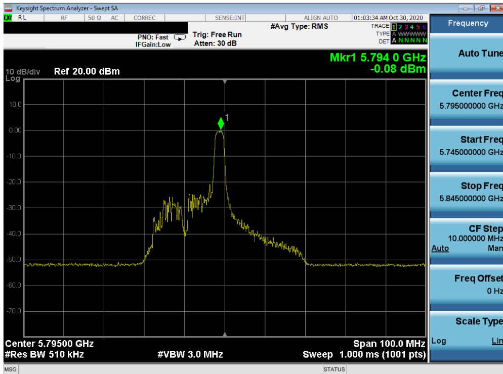
Plot 7-188. Power Spectral Density Plot MIMO ANT2 (40MHz BW 802.11ax – 26 Tones (UNII Band 3) – Ch. 159)
