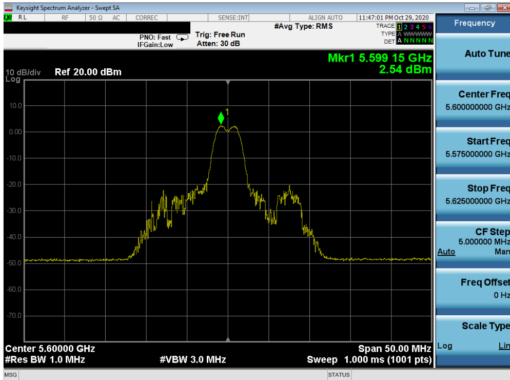
Plot 7-122. Power Spectral Density Plot MIMO ANT1 (20MHz BW 802.11ax – 26 Tones (UNII Band 2C) – Ch. 120)
