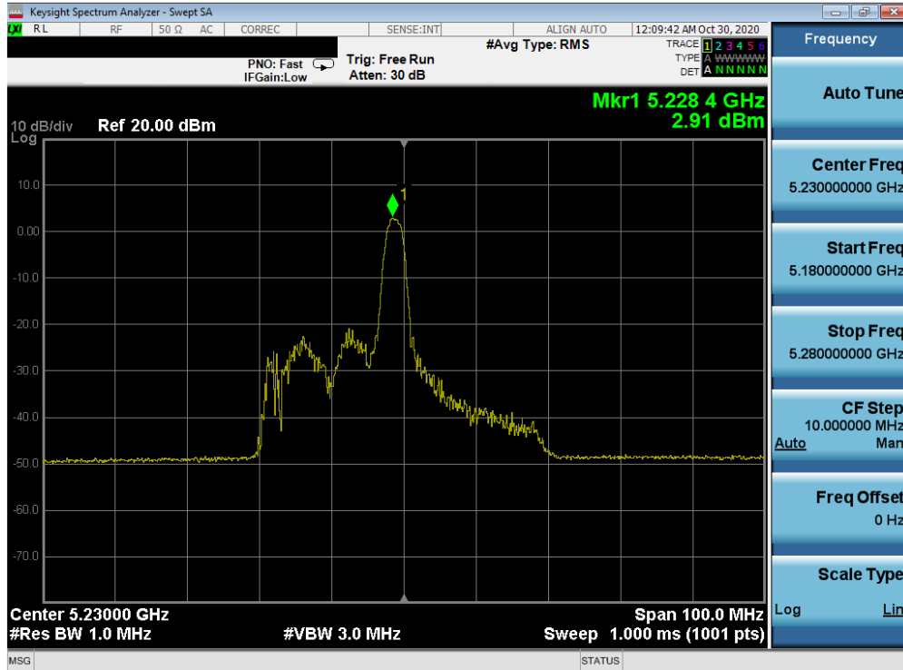
Plot 7-113. Power Spectral Density Plot MIMO ANT1 (40MHz BW 802.11ax – 26 Tones (UNII Band 1) – Ch. 46)
