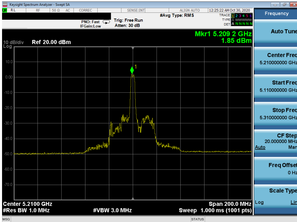
Plot 7-114. Power Spectral Density Plot MIMO ANT1 (80MHz BW 802.11ax – 26 Tones (UNII Band 1) – Ch. 42)
