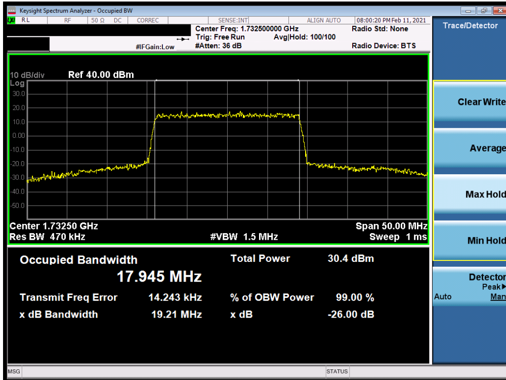
Plot 7-1. Occupied Bandwidth Plot (LTE Band 4 - 20MHz QPSK - Full RB Configuration)
