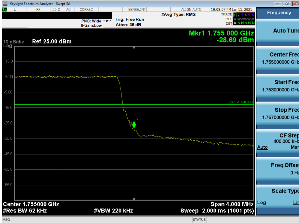
Plot 7-72. Upper Band Edge Plot (LTE Band 4 - 5MHz QPSK – Full RB)
