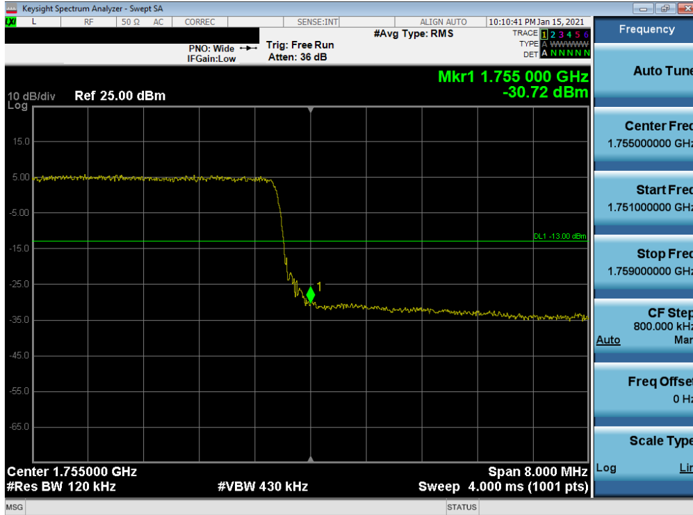
Plot 7-68. Upper Band Edge Plot (LTE Band 4 - 10MHz QPSK – Full RB)
