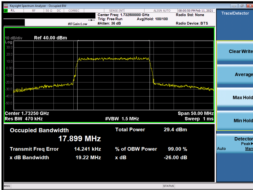
Plot 7-2. Occupied Bandwidth Plot (LTE Band 4 - 20MHz 16-QAM - Full RB Configuration)
