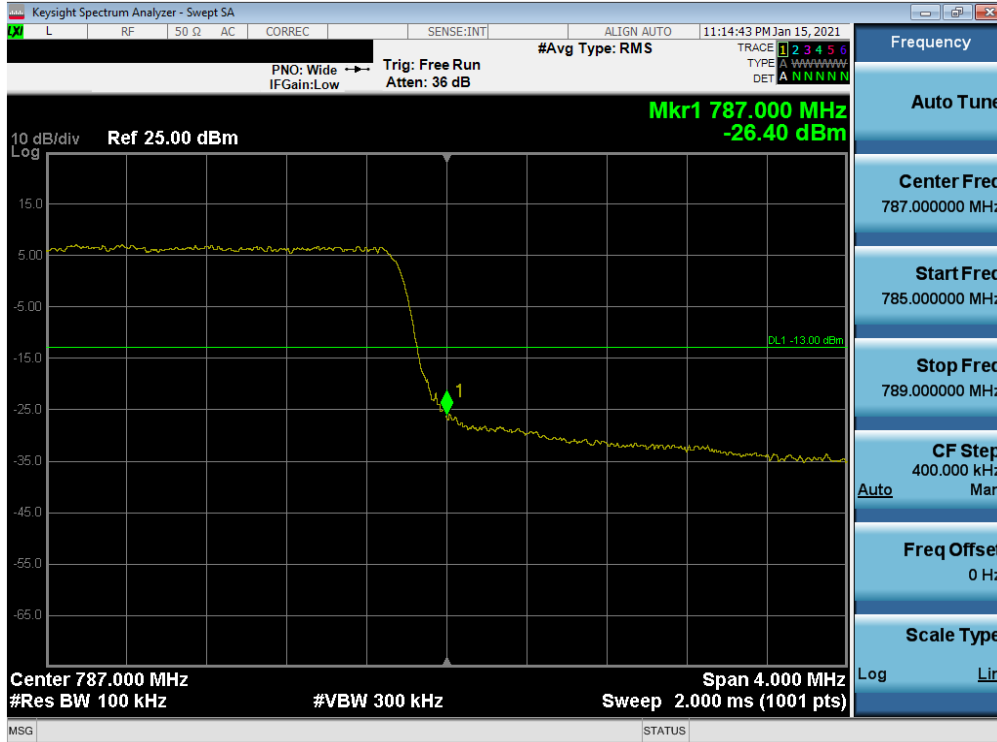
Plot 7-96. Upper Band Edge Plot (LTE Band 13 - 5MHz QPSK – Full RB)
