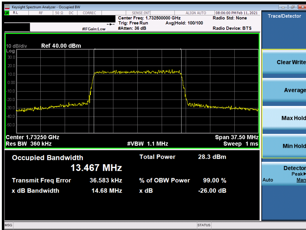
Plot 7-6. Occupied Bandwidth Plot (LTE Band 4 - 15MHz 64-QAM - Full RB Configuration)
