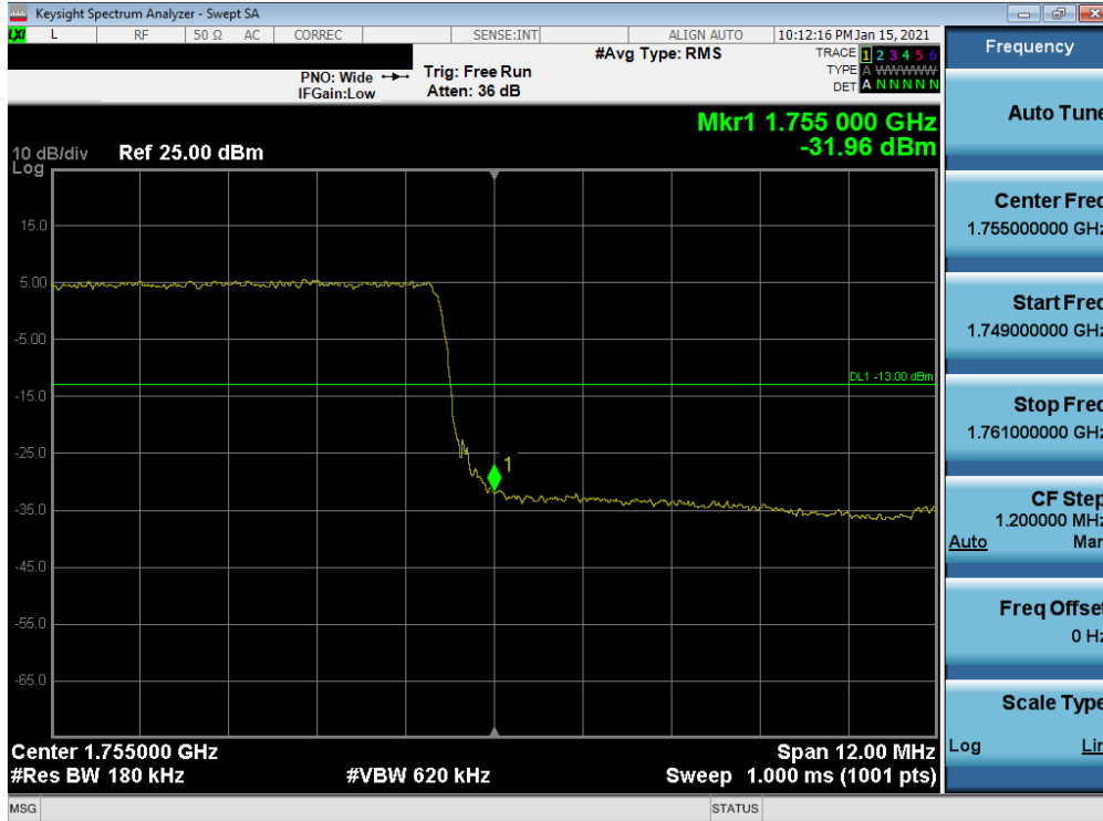
Plot 7-64. Upper Band Edge Plot (LTE Band 4 - 15MHz QPSK – Full RB)
