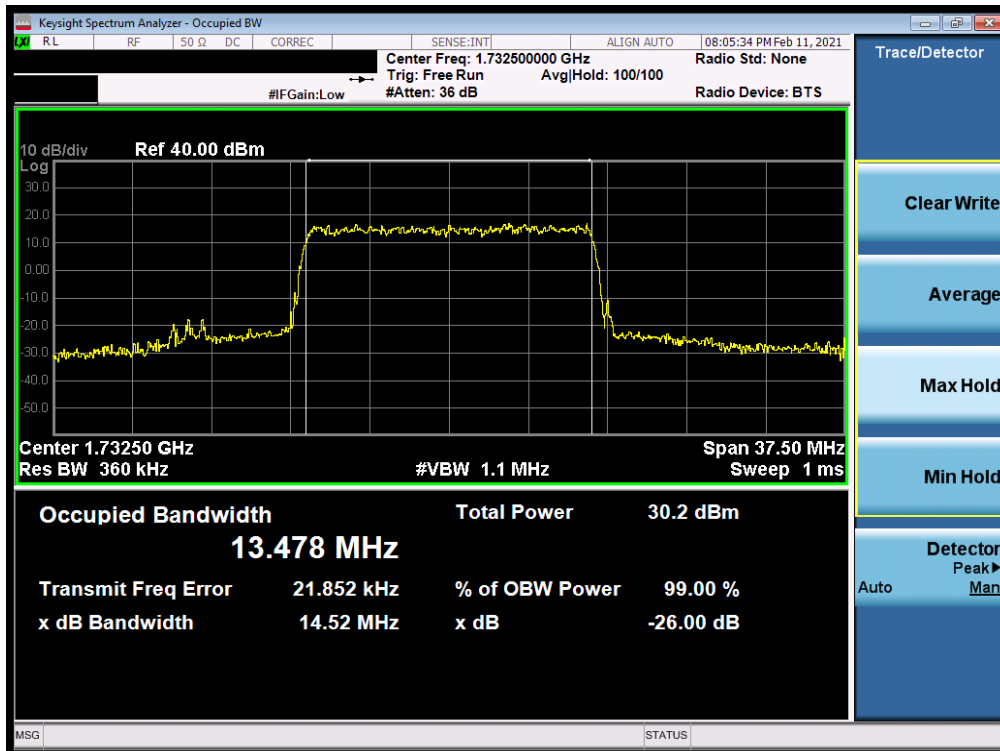
Plot 7-4. Occupied Bandwidth Plot (LTE Band 4 - 15MHz QPSK - Full RB Configuration)
