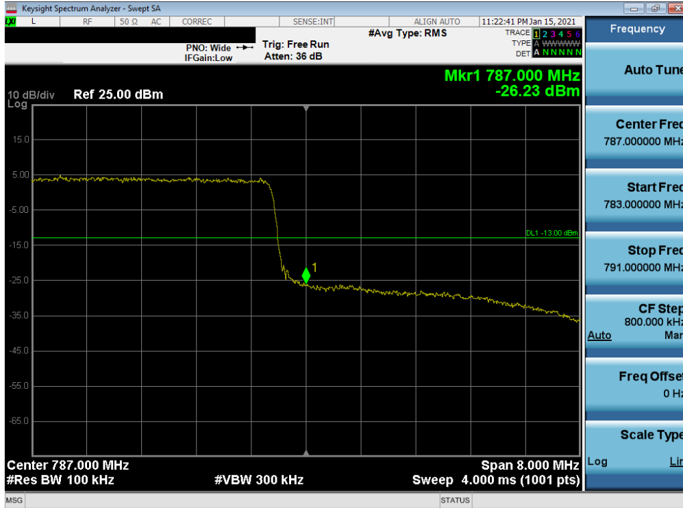
Plot 7-92. Upper Band Edge Plot (LTE Band 13 - 10MHz QPSK – Full RB)
