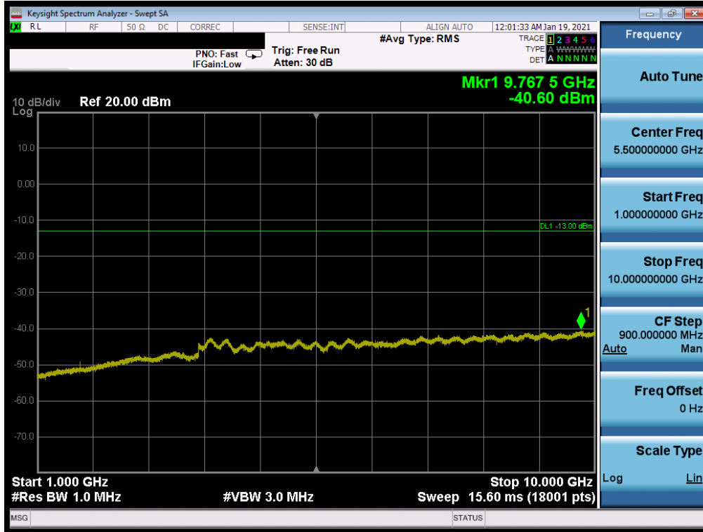
Plot 7-42. Conducted Spurious Plot (WCDMA Ch. 4233)
