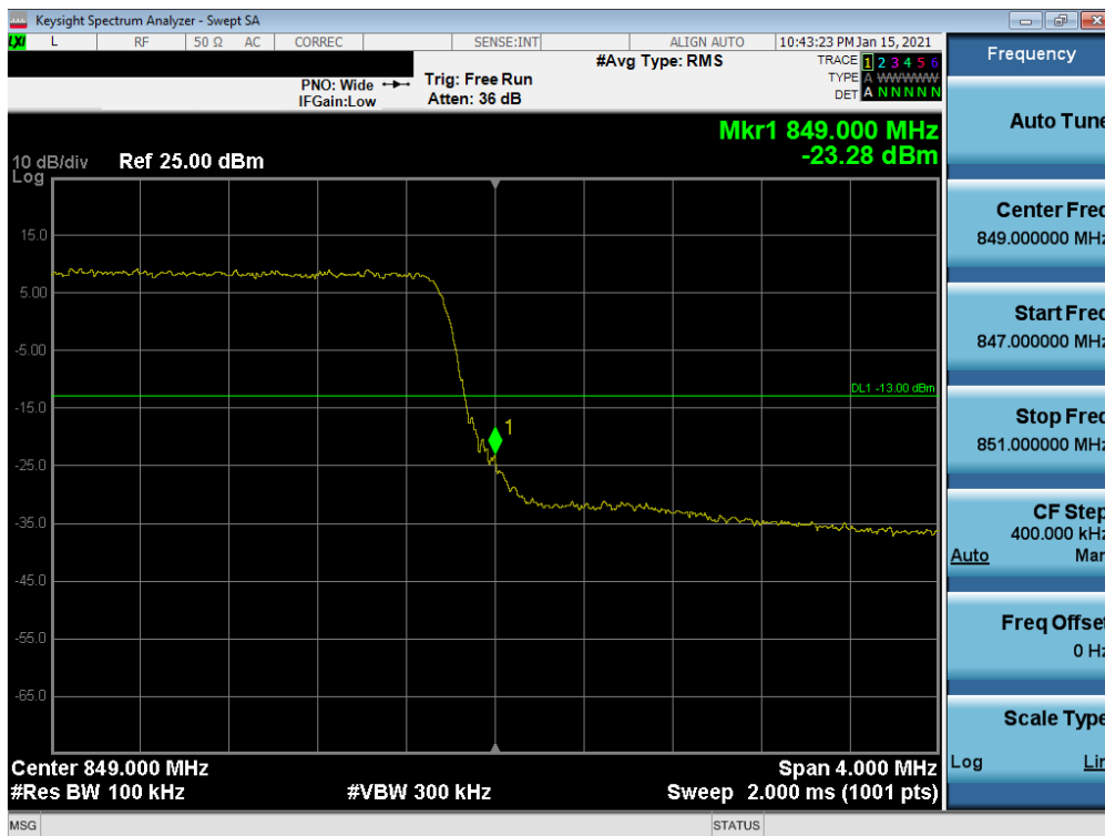
Plot 7-46. Upper Band Edge Plot (LTE Band 5 - 5MHz QPSK – Full RB Configuration)
