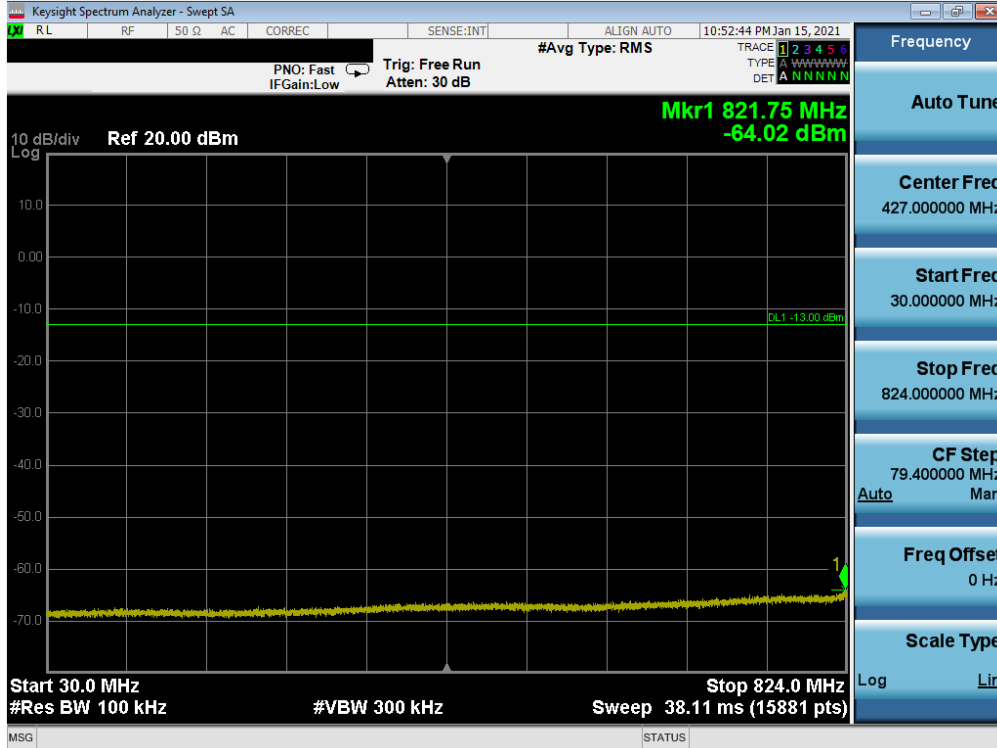
Plot 7-22. Conducted Spurious Plot (LTE Band 5 - 10MHz QPSK - RB Size 1, RB Offset 0 - High Channel)
