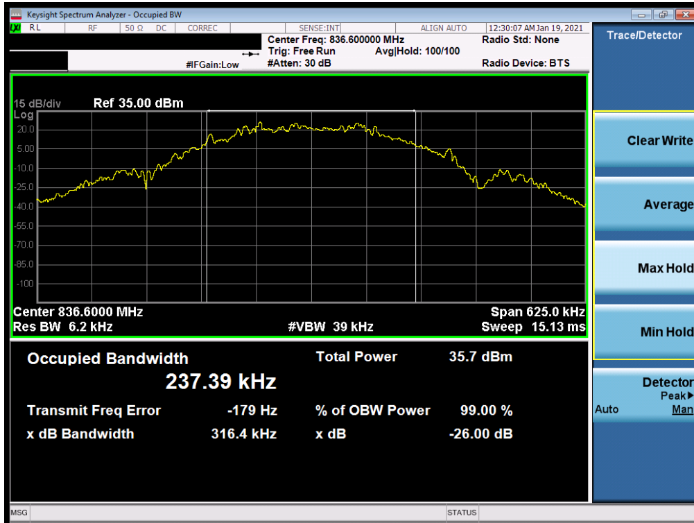
Plot 7-14. Occupied Bandwidth Plot (EDGE, Ch. 190)
