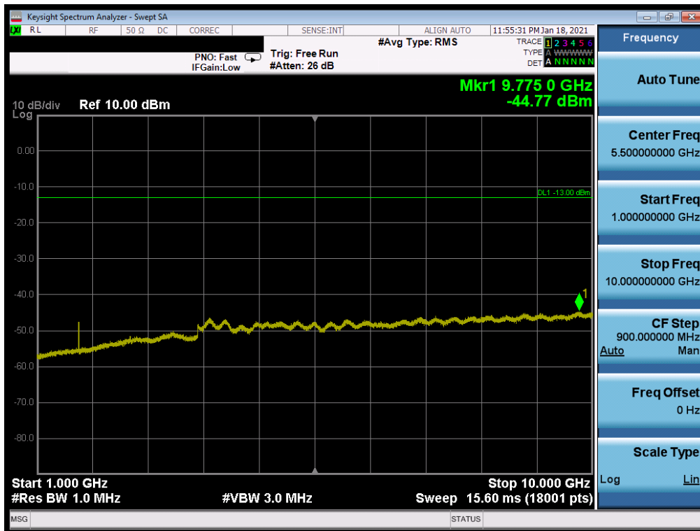
Plot 7-39. Conducted Spurious Plot (WCDMA Ch. 4183)
