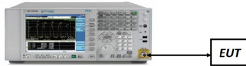
Figure 7-4. Test Instrument & Measurement Setup
