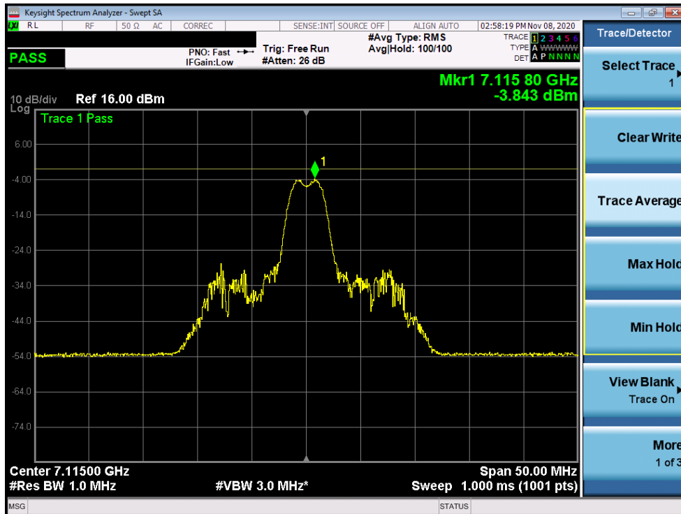
Plot 7-193. Power Spectral Density Plot MIMO ANT2 (20MHz BW 802.11ax (26 Tones) (UNII Band 8) – Ch. 233)
