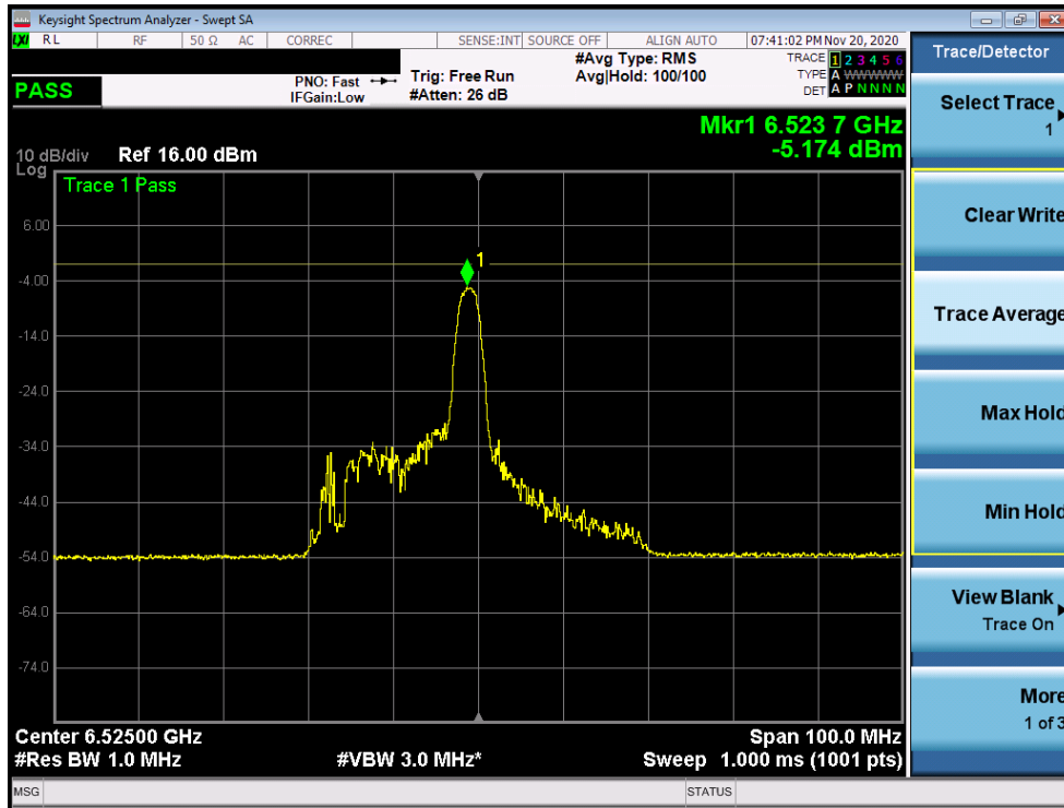
Plot 7-180. Power Spectral Density Plot MIMO ANT2 (40MHz BW 802.11ax (26 Tones) (UNII Band 6) – Ch. 115)
