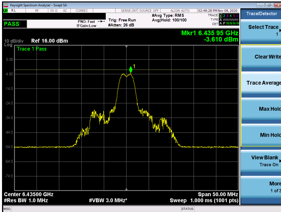
Plot 7-175. Power Spectral Density Plot MIMO ANT2 (20MHz BW 802.11ax (26 Tones) (UNII Band 6) – Ch. 97)
