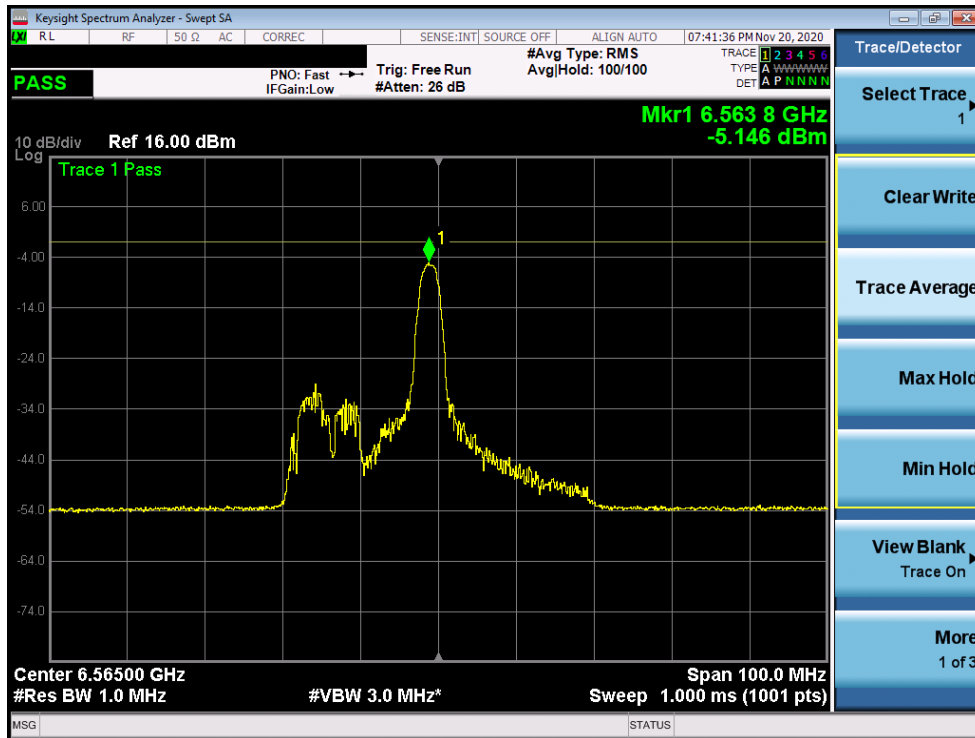
Plot 7-185. Power Spectral Density Plot MIMO ANT2 (40MHz BW 802.11ax (26 Tones) (UNII Band 7) – Ch. 123)
