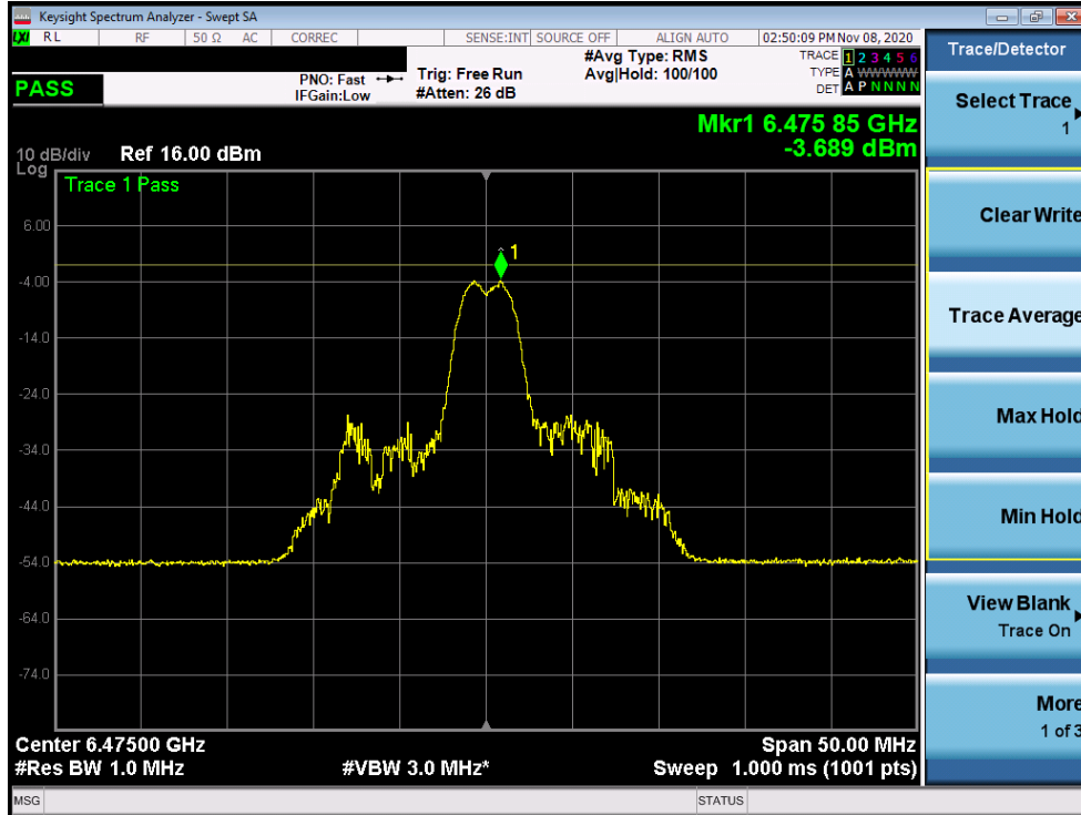
Plot 7-176. Power Spectral Density Plot MIMO ANT2 (20MHz BW 802.11ax (26 Tones) (UNII Band 6) – Ch. 105)
