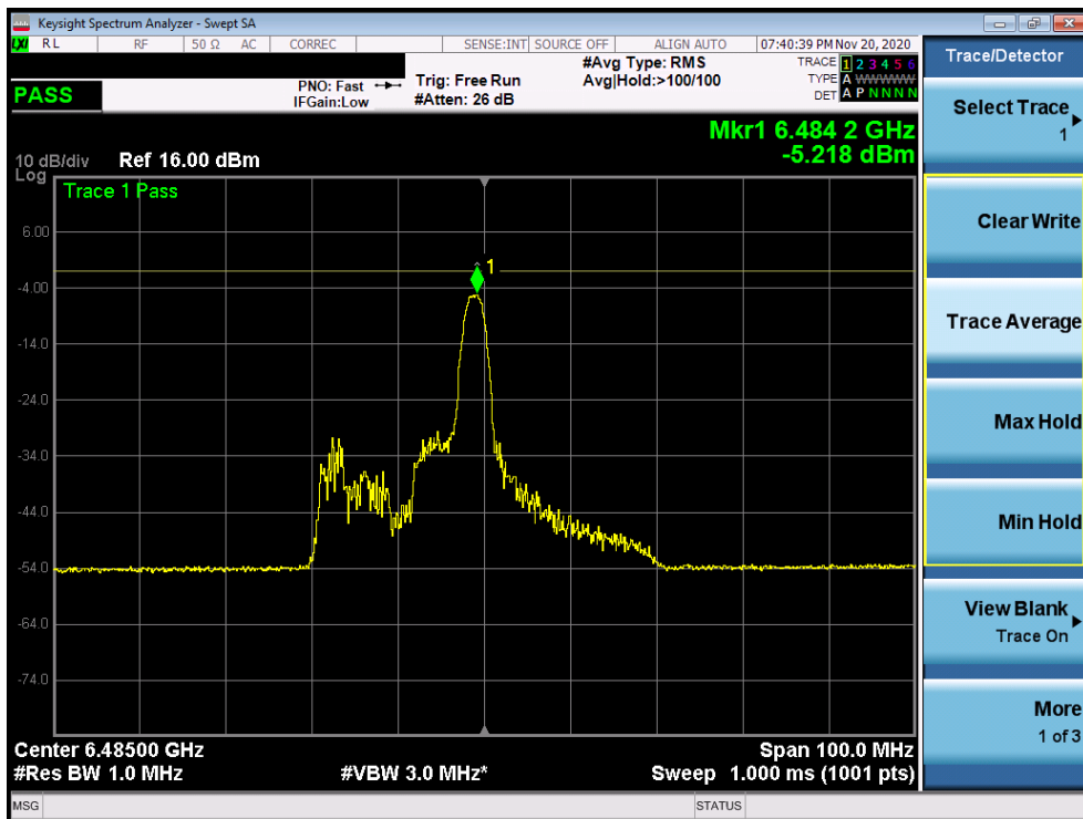
Plot 7-179. Power Spectral Density Plot MIMO ANT2 (40MHz BW 802.11ax (26 Tones) (UNII Band 6) – Ch. 107)
