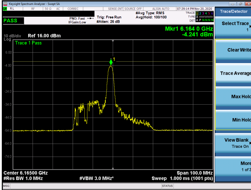
Plot 7-170. Power Spectral Density Plot MIMO ANT2 (40MHz BW 802.11ax (26 Tones) (UNII Band 5) – Ch. 43)
