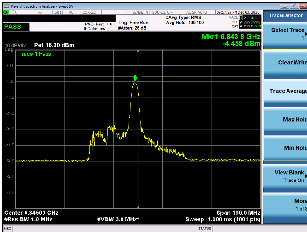
Plot 7-154. Power Spectral Density Plot MIMO ANT1 (40MHz BW 802.11ax (26 Tones) (UNII Band 7) – Ch. 179)
