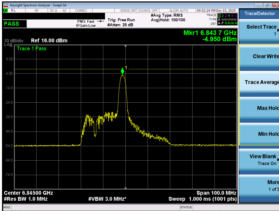
Plot 7-187. Power Spectral Density Plot MIMO ANT2 (40MHz BW 802.11ax (26 Tones) (UNII Band 7) – Ch. 179)
