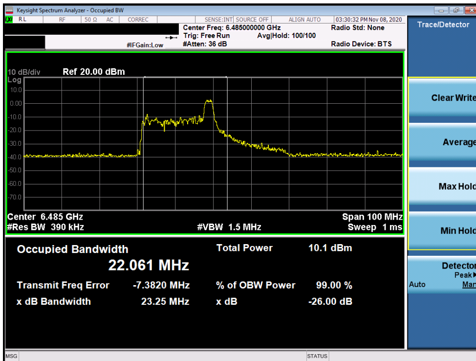
Plot 7-80. 26dB Bandwidth Plot MIMO ANT2 (40MHz BW 802.11ax (26 Tones) (UNII Band 6) – Ch. 107)
