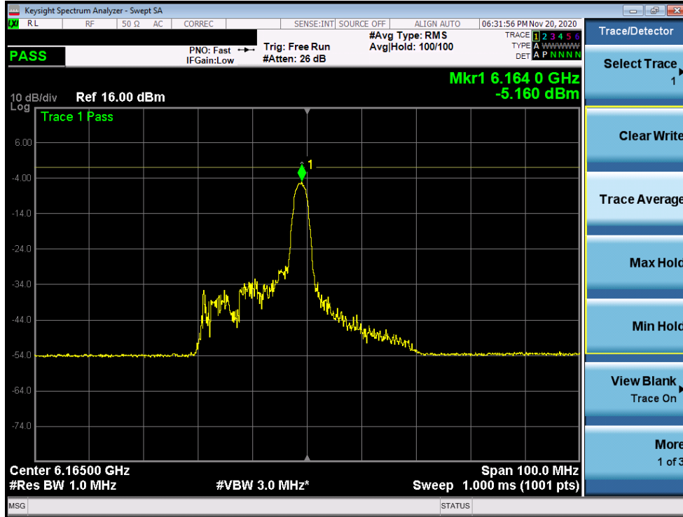
Plot 7-137. Power Spectral Density Plot MIMO ANT1 (40MHz BW 802.11ax (26 Tones) (UNII Band 5) – Ch. 43)
