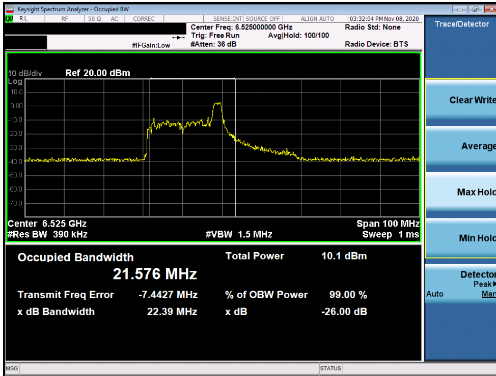
Plot 7-81. 26dB Bandwidth Plot MIMO ANT2 (40MHz BW 802.11ax (26 Tones) (UNII Band 6) – Ch. 115)
