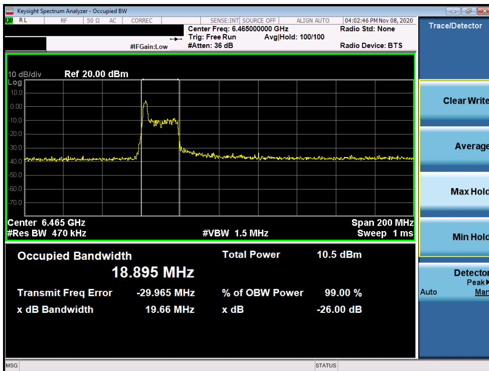
Plot 7-82. 26dB Bandwidth Plot MIMO ANT2 (80MHz BW 802.11ax (26 Tones) (UNII Band 6) – Ch. 103)
