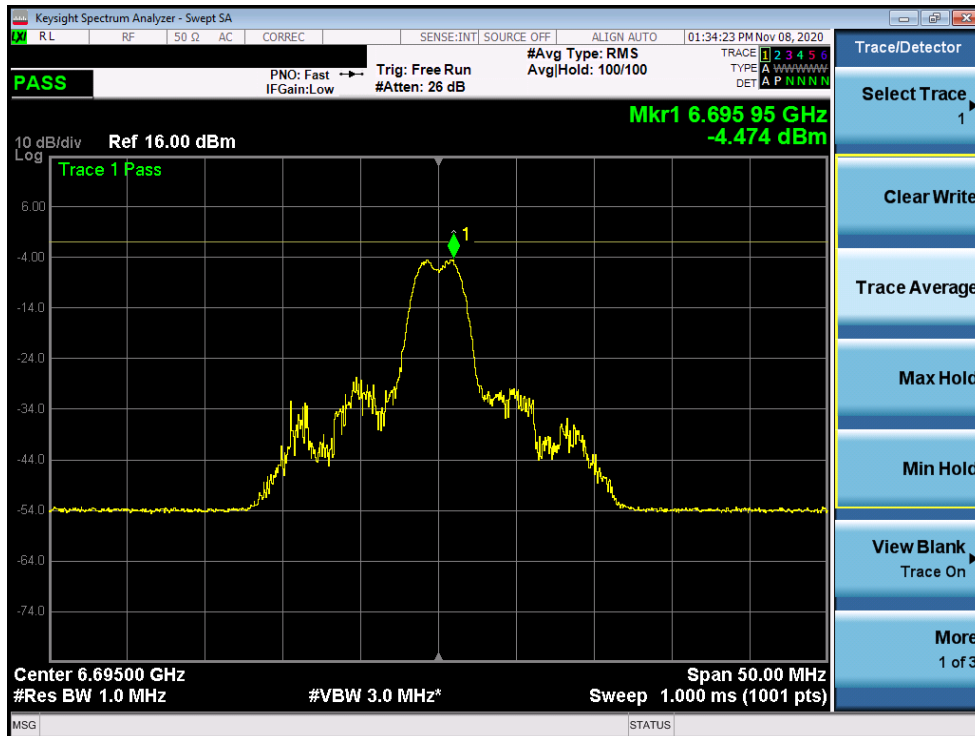
Plot 7-150. Power Spectral Density Plot MIMO ANT1 (20MHz BW 802.11ax (26 Tones) (UNII Band 7) – Ch. 149)
