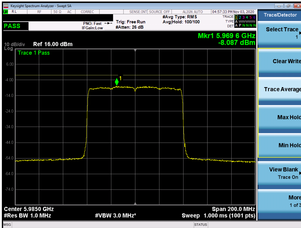
Plot 7-111. Power Spectral Density Plot MIMO ANT1 (80MHz BW 802.11ax (UNII Band 5) – Ch. 7)
