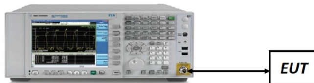
Figure 7-1. Test Instrument & Measurement Setup
