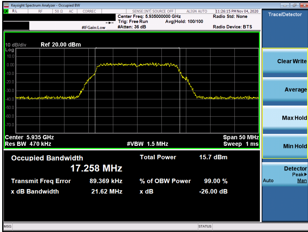
Plot 7-53. 26dB Bandwidth Plot MIMO ANT2 (20MHz BW 802.11a UNII Band 5) – Ch. 2)
