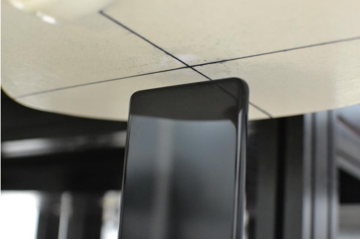
SAR Test Setup Photo 15 – Bottom Edge at 10mm
