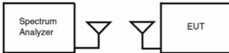
Figure 7-2. Test Instrument and Measurement Setup
