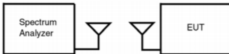
Figure 7-1. Test Instrument and Measurement Setup
