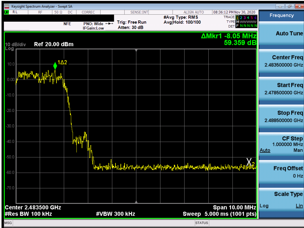
Plot 7-98. Band Edge Plot (Bluetooth with Hopping Enabled, ANT 2-3 Mbps)
