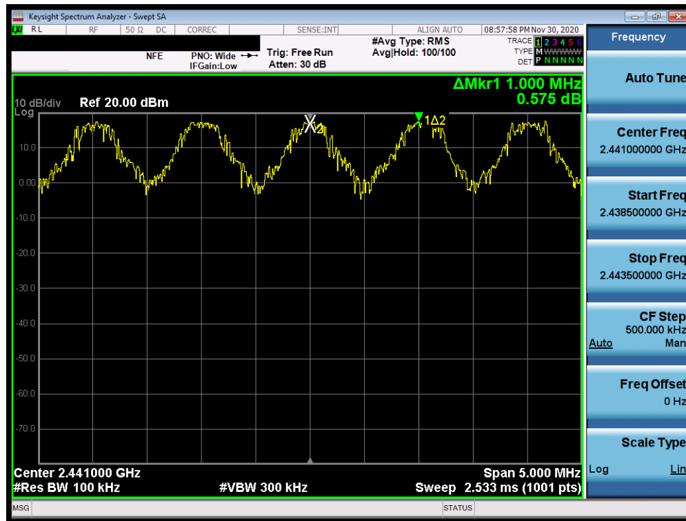
Plot 7-99. Channel Spacing Plot (Bluetooth)-ANT 1
