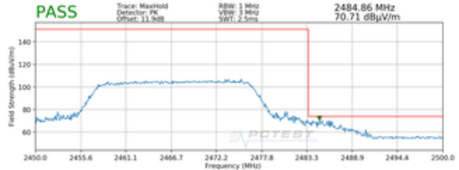
Plot 7-110. Radiated Restricted Upper Band Edge Measurement MIMO (Peak – 242 Tones)
