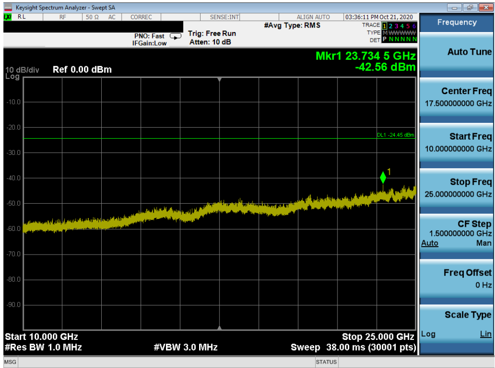
Plot 7-68. Conducted Spurious Plot ANT2 (802.11ax OFDMA – 242 Tones – Ch. 11)
