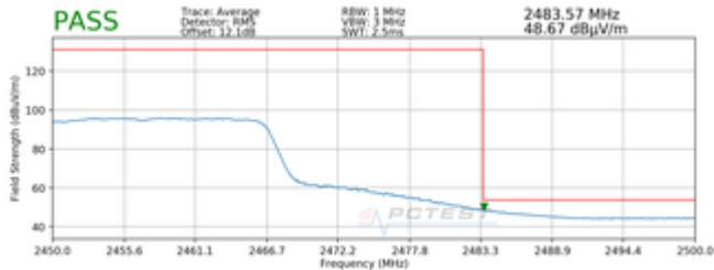
Plot 7-105. Radiated Restricted Upper Band Edge Measurement MIMO (Average – 242 Tones)
