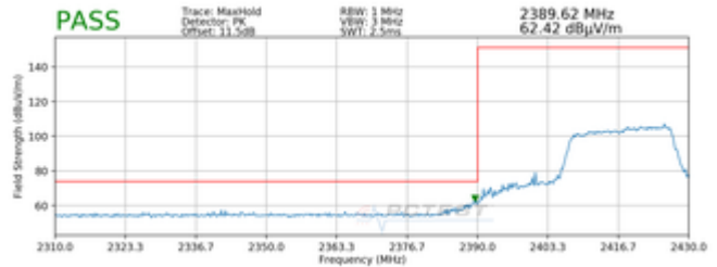
Plot 7-104. Radiated Restricted Lower Band Edge Measurement MIMO (Peak – 242 Tones)
