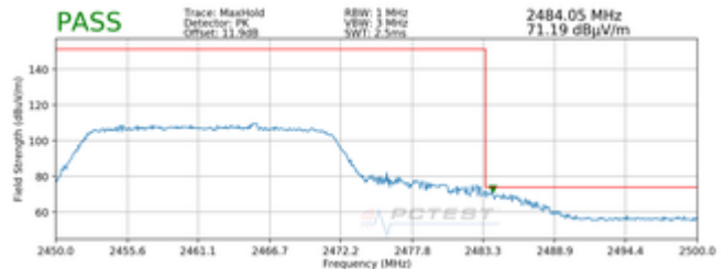
Plot 7-108. Radiated Restricted Upper Band Edge Measurement MIMO (Peak – 242 Tones)
