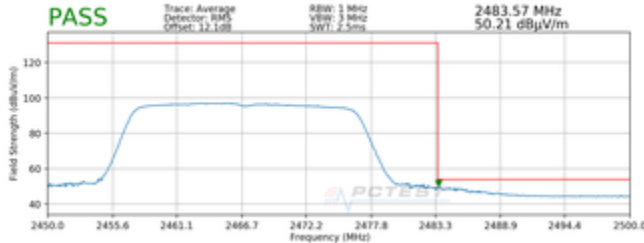
Plot 7-109. Radiated Restricted Upper Band Edge Measurement MIMO (Average – 242 Tones)
