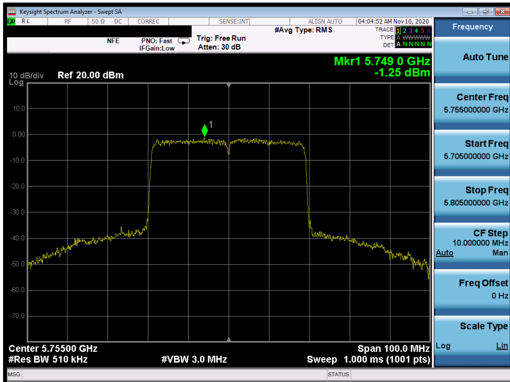
Plot 7-214. Power Spectral Density Plot MIMO ANT2 (40MHz BW 802.11ax – Full Tones (UNII Band 3) – Ch. 151)
