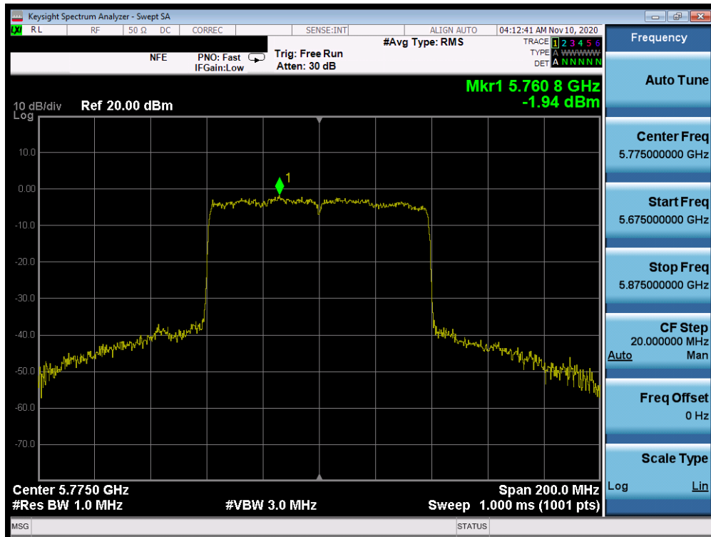
Plot 7-216. Power Spectral Density Plot MIMO ANT2 (80MHz BW 802.11ax – Full Tones (UNII Band 3) – Ch. 155)
