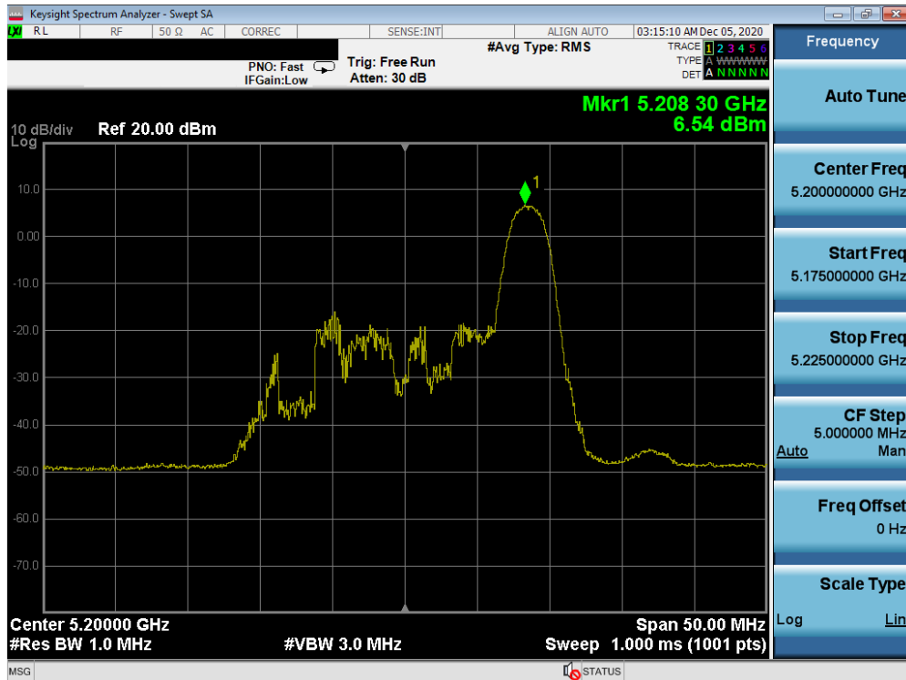
Plot 7-164. Power Spectral Density Plot MIMO ANT2 (20MHz BW 802.11ax – 26 Tones (UNII Band 1) – Ch. 40)
