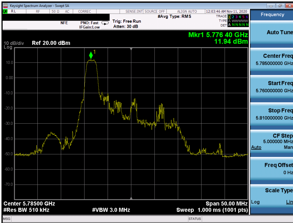
Plot 7-185. Power Spectral Density Plot MIMO ANT2 (20MHz BW 802.11ax – 26 Tones (UNII Band 3) – Ch. 157)
