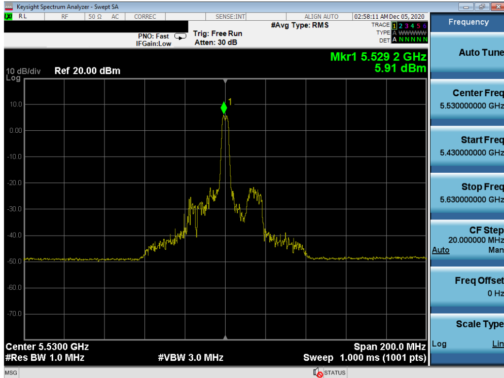
Plot 7-127. Power Spectral Density Plot MIMO ANT1 (80MHz BW 802.11ax – 26 Tones (UNII Band 2C) – Ch. 106)
