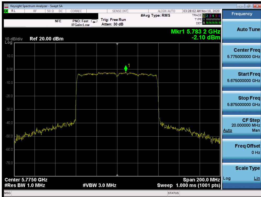
Plot 7-162. Power Spectral Density Plot MIMO ANT1 (80MHz BW 802.11ax – Full Tones (UNII Band 3) – Ch. 155)
