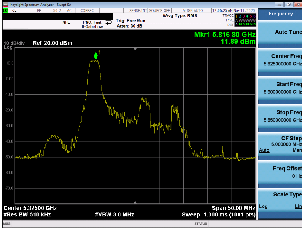
Plot 7-186. Power Spectral Density Plot MIMO ANT2 (20 MHz BW 802.11ax – 26 Tones (UNII Band 3) – Ch. 165)
