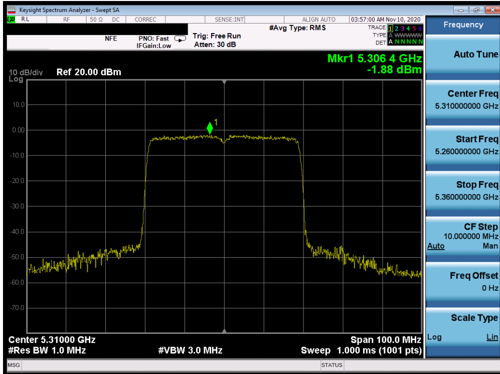
Plot 7-200. Power Spectral Density Plot MIMO ANT2 (40MHz BW 802.11ax – Full Tones (UNII Band 2A) – Ch. 62)
