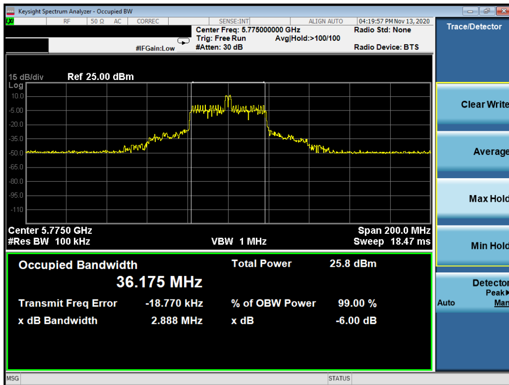
Plot 7-102. 6dB Bandwidth Plot MIMO ANT2 (80MHz BW 802.11ax – 26 Tones (UNII Band 3) – Ch. 155)
