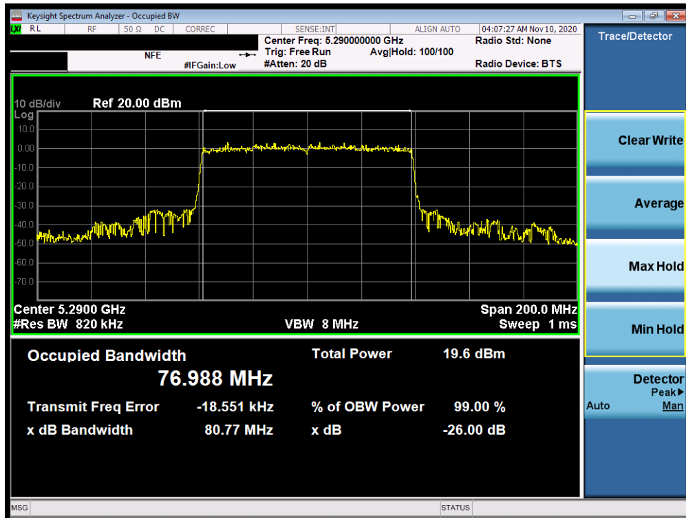
Plot 7-75. 26dB Bandwidth Plot MIMO ANT2 (80MHz BW 802.11ax – 996 Tones (UNII Band 2A) – Ch. 58)
