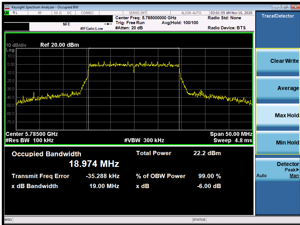
Plot 7-92. 6dB Bandwidth Plot MIMO ANT1 (20MHz BW 802.11ax – 242 Tones (UNII Band 3) – Ch. 157)
