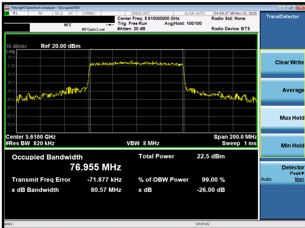
Plot 7-83. 26dB Bandwidth Plot MIMO ANT2 (80MHz BW 802.11ax – 996 Tones (UNII Band 2C) – Ch. 122)
