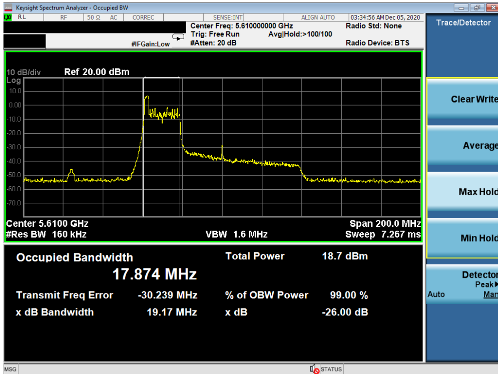
Plot 7-62. 26dB Bandwidth Plot MIMO ANT2 (80MHz BW 802.11ax – 26 Tones (UNII Band 2C) – Ch. 122)
