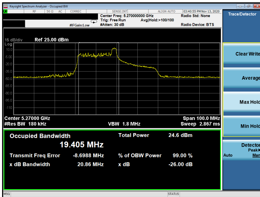
Plot 7-52. 26dB Bandwidth Plot MIMO ANT2 (40MHz BW 802.11ax – 26 Tones (UNII Band 2A) – Ch. 54)
