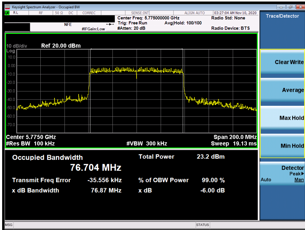
Plot 7-96. 6dB Bandwidth Plot MIMO ANT1 (80MHz BW 802.11ax – 996 Tones (UNII Band 3) – Ch. 155)
