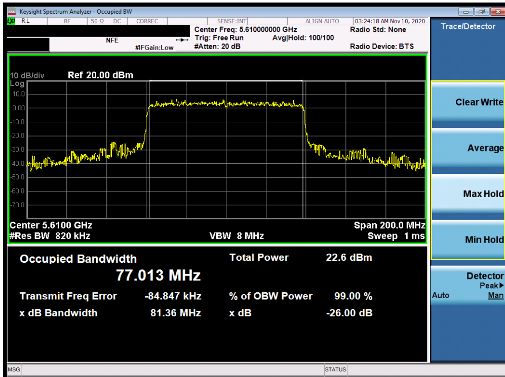
Plot 7-41. 26dB Bandwidth Plot MIMO ANT1 (80MHz BW 802.11ax – 996 Tones (UNII Band 2C) – Ch. 122)
