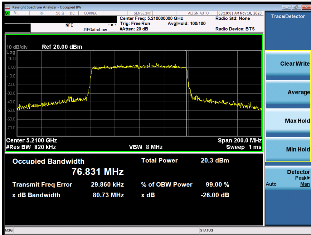
Plot 7-27. 26dB Bandwidth Plot MIMO ANT1 (80MHz BW 802.11ax – 996 Tones (UNII Band 1) – Ch. 42)
