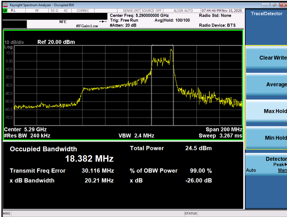
Plot 7-12. 26dB Bandwidth Plot MIMO ANT1 (80MHz BW 802.11ax – 26 Tones (UNII Band 2A) – Ch. 58)
