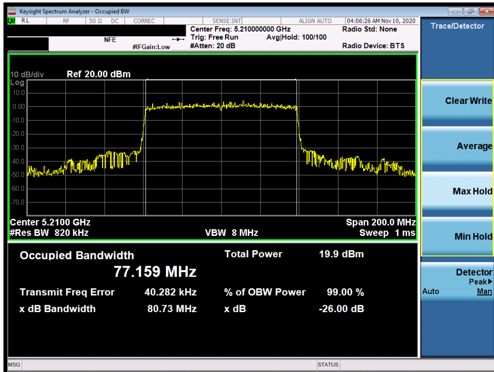
Plot 7-69. 26dB Bandwidth Plot MIMO ANT2 (80MHz BW 802.11ax – 996 Tones (UNII Band 1) – Ch. 42)
