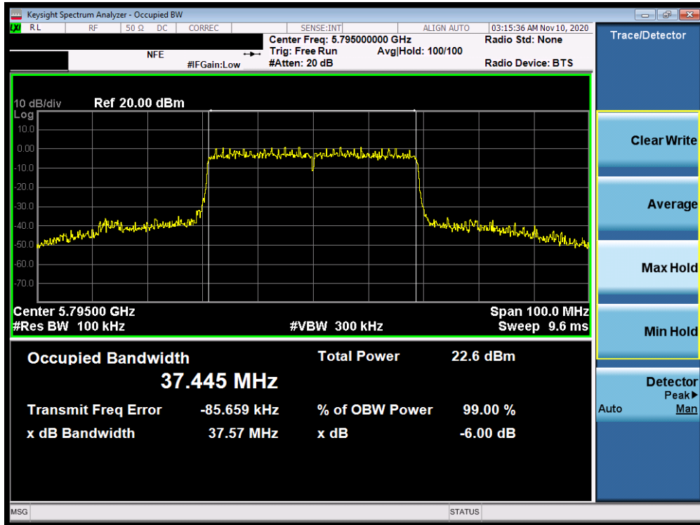
Plot 7-95. 6dB Bandwidth Plot MIMO ANT1 (40MHz BW 802.11ax – 484 Tones (UNII Band 3) – Ch. 159)
