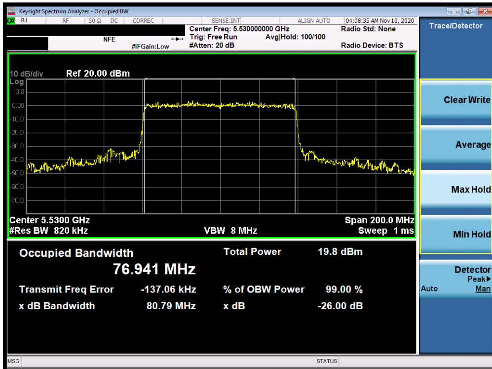
Plot 7-82. 26dB Bandwidth Plot MIMO ANT2 (80MHz BW 802.11ax – 996 Tones (UNII Band 2C) – Ch. 106)
