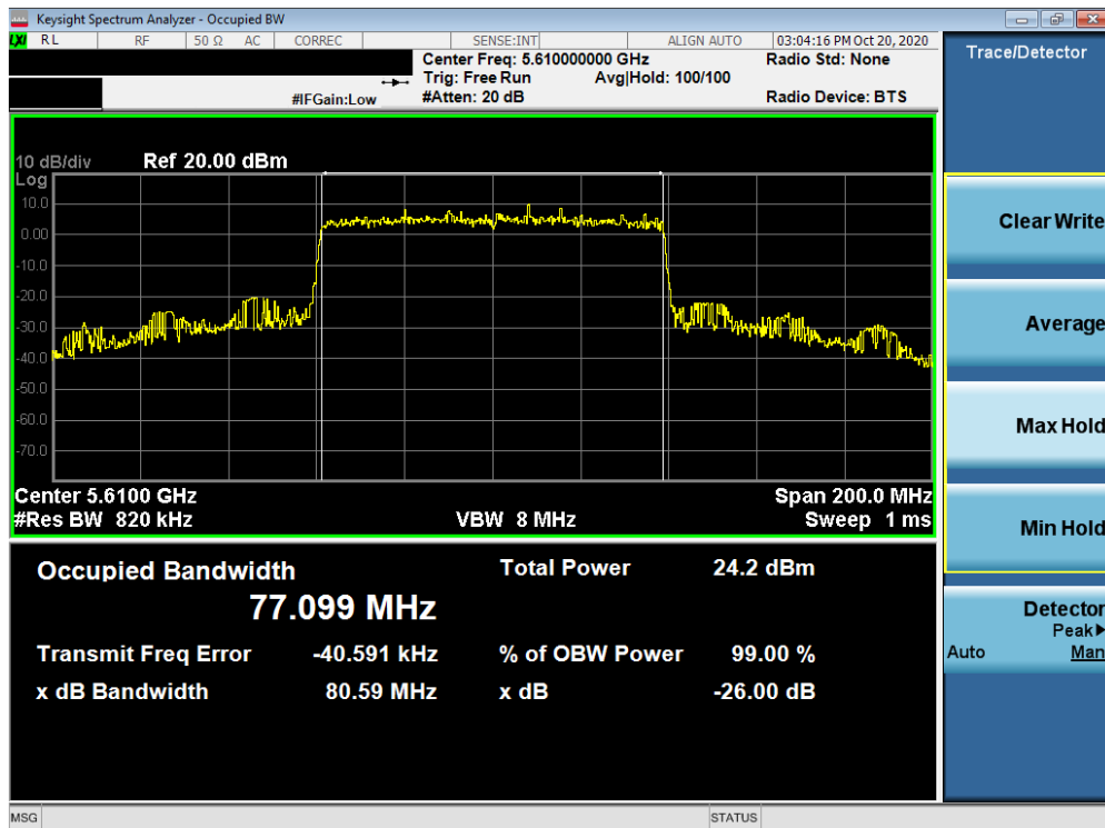
Plot 7-107. 26dB Bandwidth Plot MIMO ANT2 (80MHz BW 802.11ax (UNII Band 2C) – Ch. 122)
