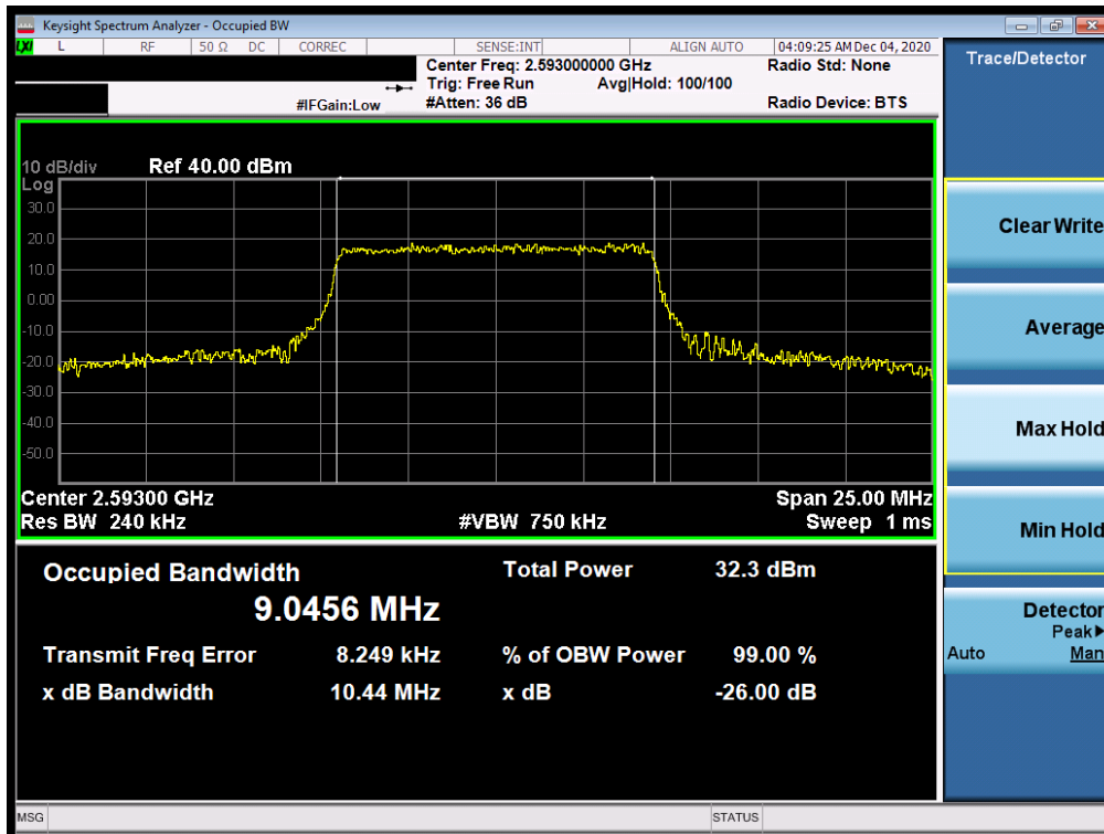
Plot 7-10. Occupied Bandwidth Plot (LTE Band 41(PC2) - 10MHz 16-QAM - Full RB Configuration)
