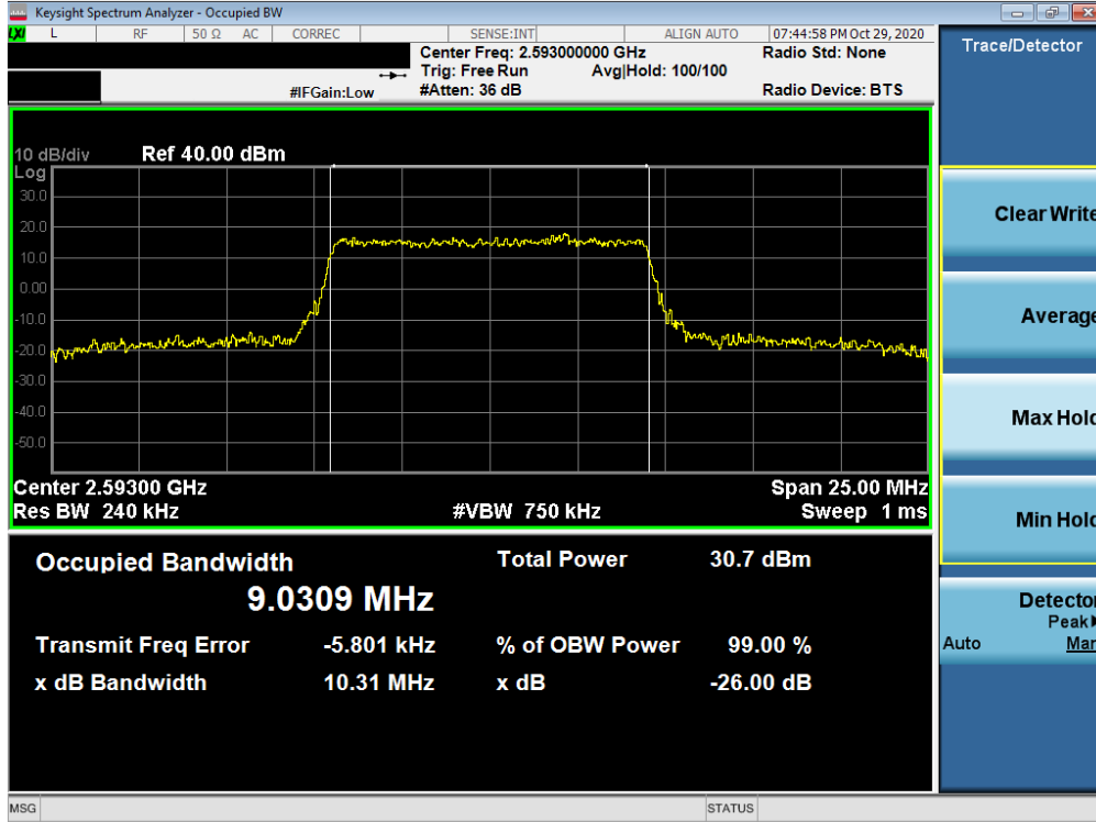
Plot 7-11. Occupied Bandwidth Plot (LTE Band 41(PC2) - 10MHz 64-QAM - Full RB Configuration)
