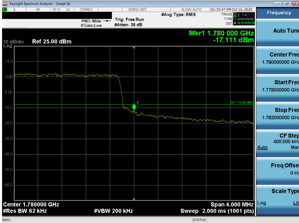
Plot 7-110. Upper Band Edge Plot (LTE Band 66 - 5MHz QPSK – Full RB Configuration)
