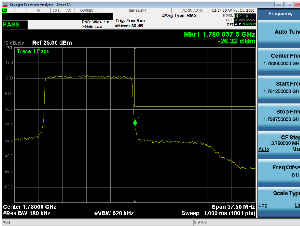
Plot 7-130. Upper Band Edge Plot (NR Band n66 – 15.0MHz DFT-s - Full RB)
