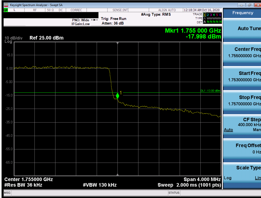
Plot 7-114. Upper Band Edge Plot (LTE Band 4 - 3MHz QPSK – Full RB Configuration)
