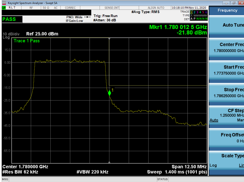
Plot 7-138. Upper Band Edge Plot (NR Band n66 – 5.0MHz DFT-s - Full RB)
