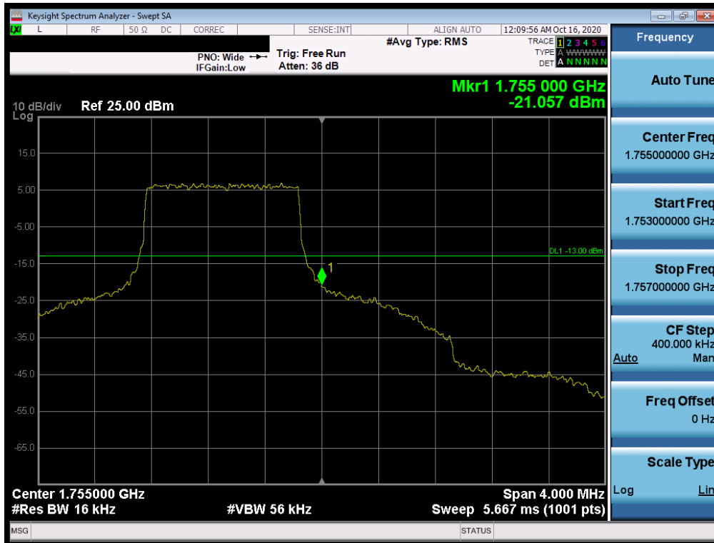
Plot 7-120. Upper Band Edge Plot (LTE Band 4 – 1.4MHz QPSK – Full RB Configuration)
