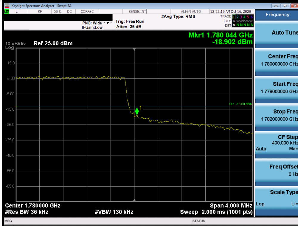
Plot 7-116. Upper Band Edge Plot (LTE Band 66 - 3MHz QPSK – Full RB Configuration)
