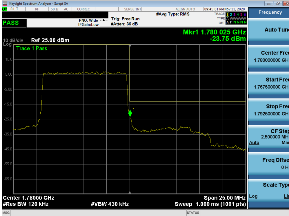
Plot 7-134. Upper Band Edge Plot (NR Band n66 – 10.0MHz DFT-s - Full RB)
