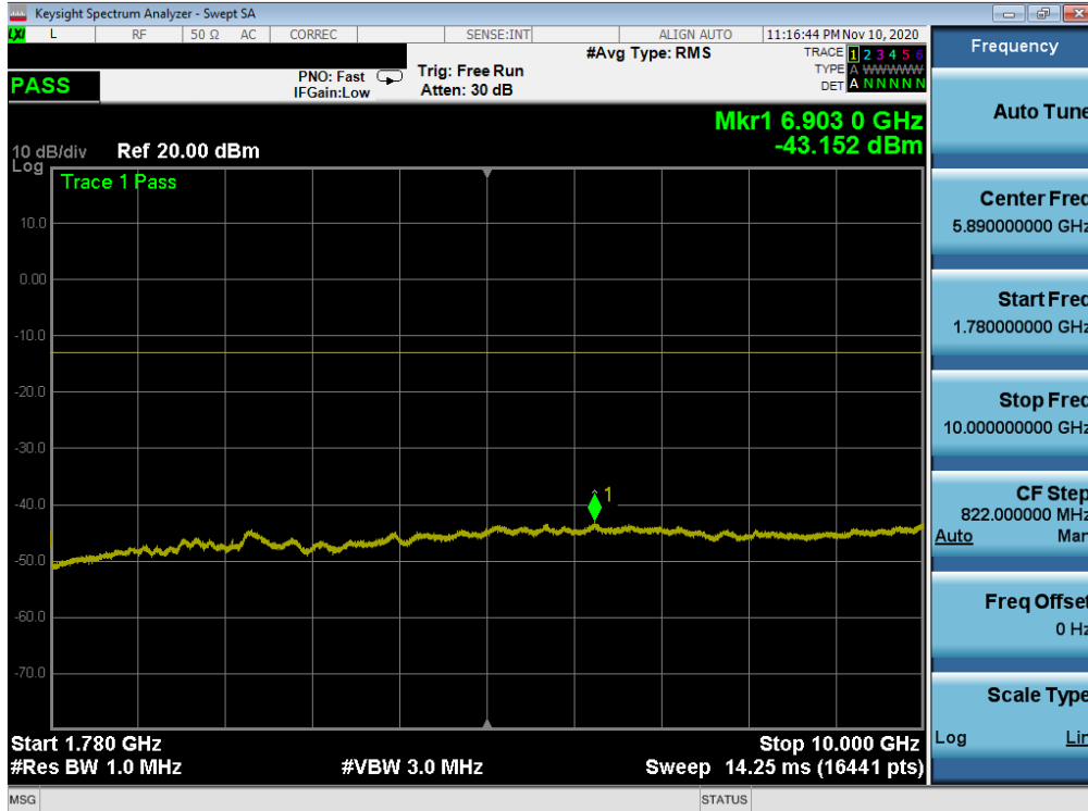
Plot 7-165. Conducted Spurious Plot (NR Band n66 - 20.0MHz - RB Size 1, RB Offset 0 - Mid Channel)
