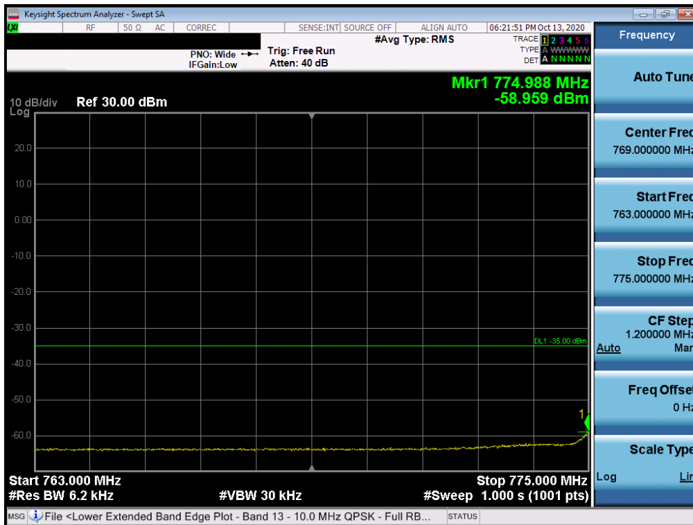
Plot 7-77. Lower Emission Mask Plot (LTE Band 13 - 10MHz QPSK – Full RB Configuration)
