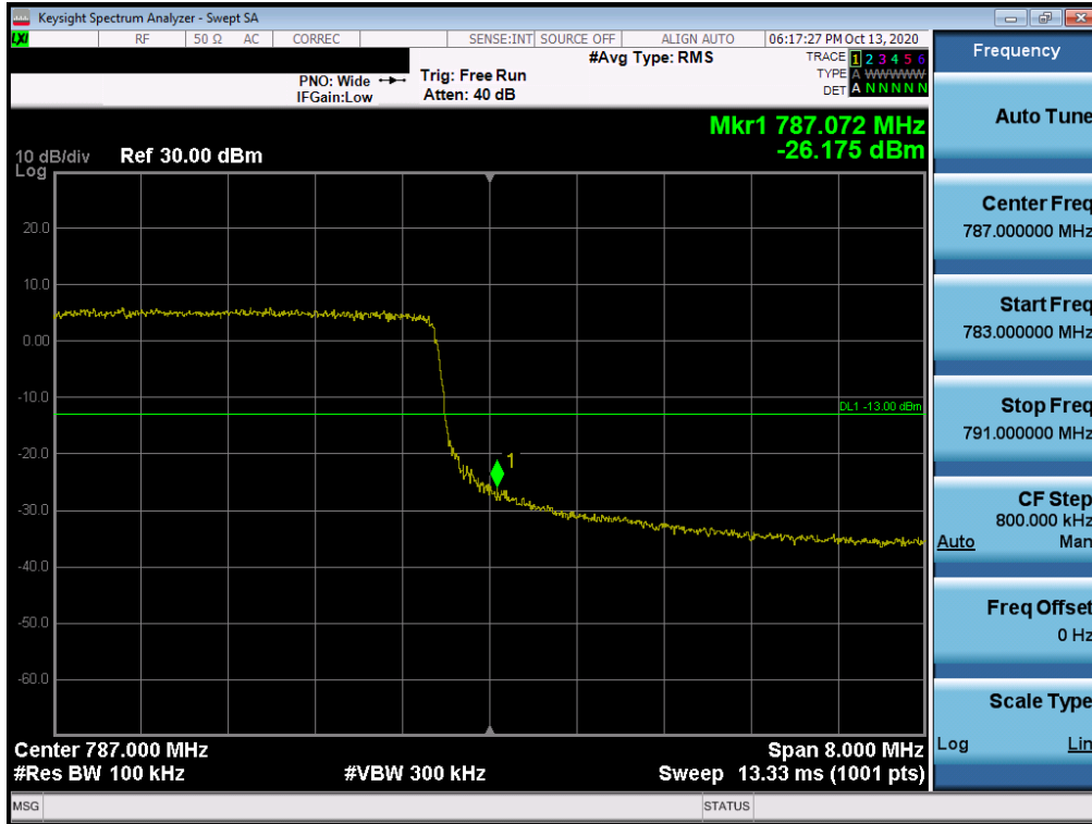
Plot 7-78. Upper Band Edge Plot (LTE Band 13 - 10MHz QPSK – Full RB Configuration)
