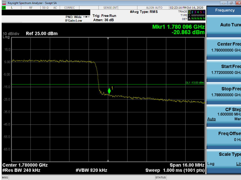
Plot 7-92. Upper Band Edge Plot (LTE Band 66 - 20MHz QPSK – Full RB Configuration)
