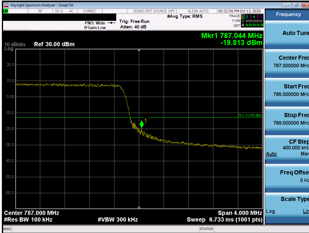
Plot 7-82. Upper Band Edge Plot (LTE Band 13 - 5MHz QPSK – Full RB Configuration)
