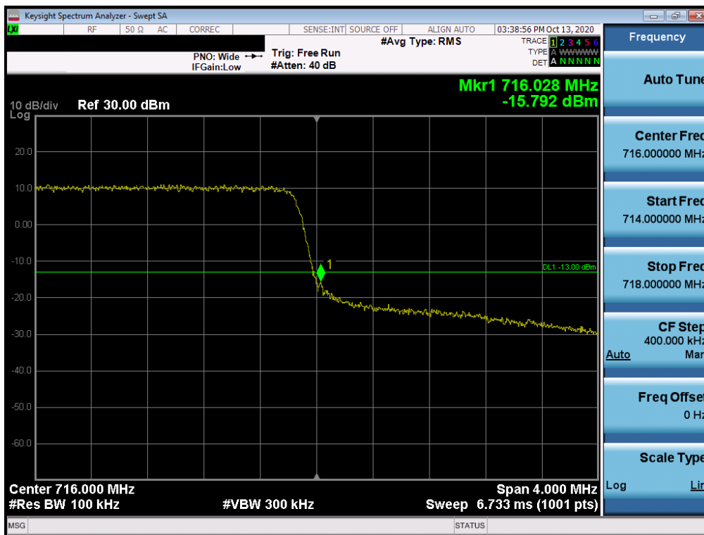
Plot 7-73. Upper Band Edge Plot (LTE Band 12 - 3MHz QPSK – Full RB Configuration)
