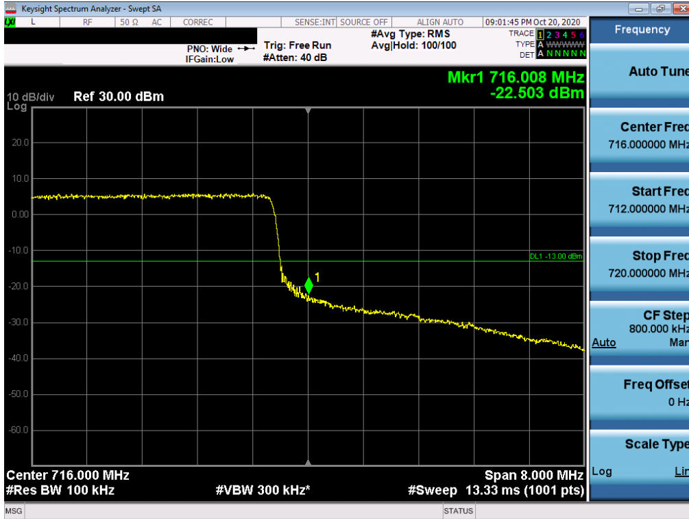
Plot 7-68. Upper Band Edge Plot (LTE Band 12/17 - 10MHz QPSK – Full RB Configuration)
