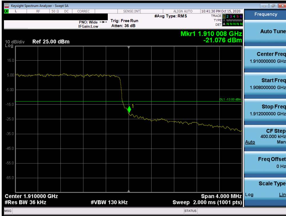
Plot 7-81. Upper Band Edge Plot (LTE Band 2 - 3MHz QPSK – Full RB Configuration)
