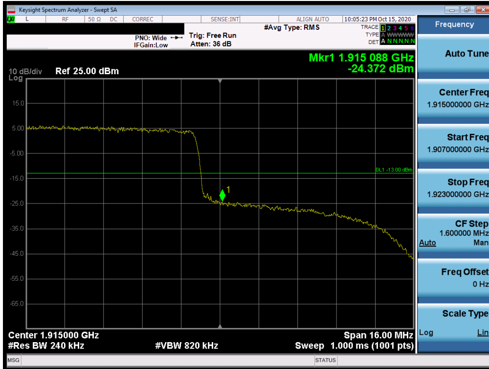
Plot 7-59. Upper Band Edge Plot (LTE Band 25 - 20MHz QPSK – Full RB Configuration)
