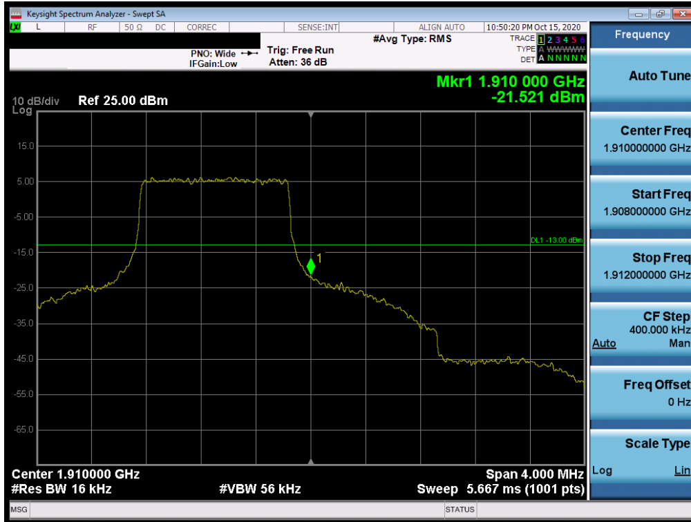
Plot 7-87. Upper Band Edge Plot (LTE Band 2 – 1.4MHz QPSK – Full RB Configuration)
