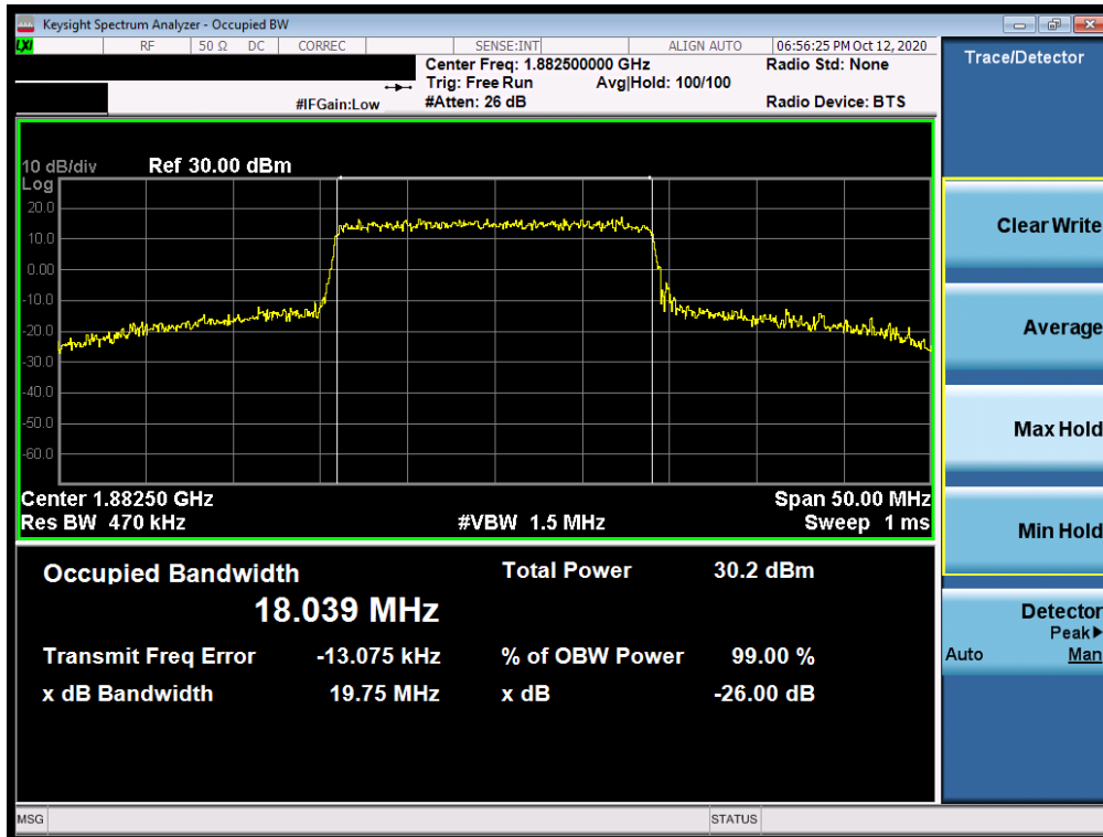
Plot 7-2. Occupied Bandwidth Plot (LTE Band 25/2 - 20MHz 16-QAM - Full RB Configuration)
