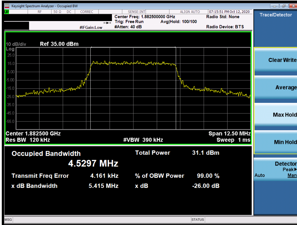
Plot 7-13. Occupied Bandwidth Plot (LTE Band 25/2 - 5MHz QPSK - Full RB Configuration)
