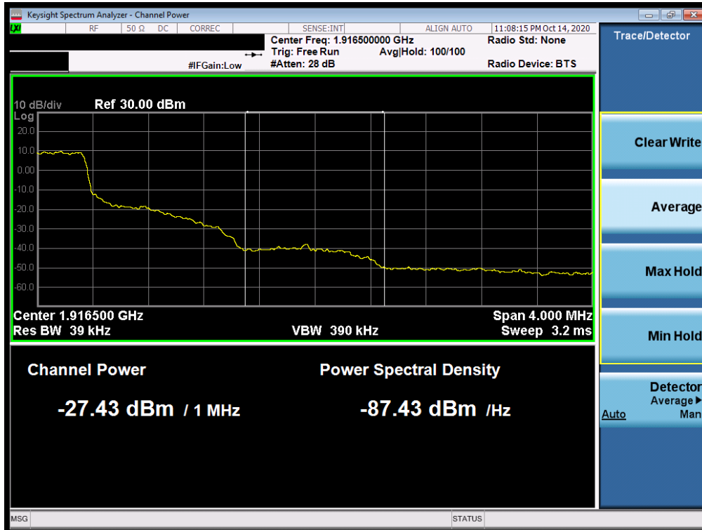
Plot 7-90. Extended Upper Band Edge Plot (LTE Band 25 – 1.4MHz QPSK – Full RB Configuration)
