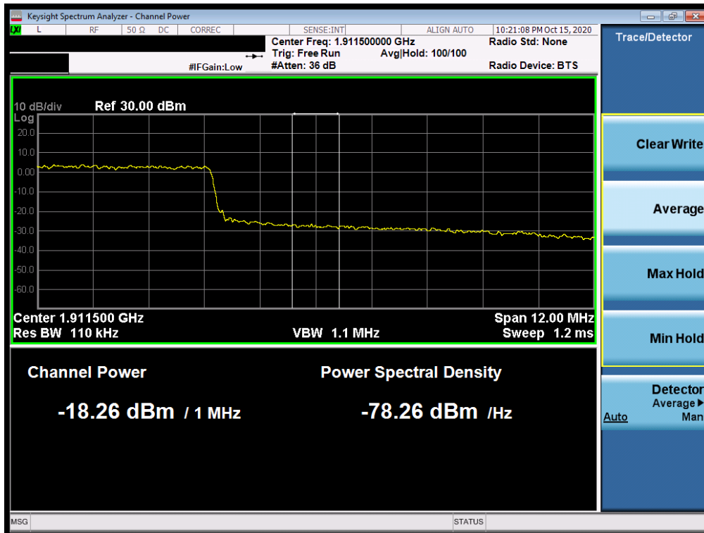
Plot 7-64. Extended Upper Band Edge Plot (LTE Band 2 - 15MHz QPSK – Full RB Configuration)
