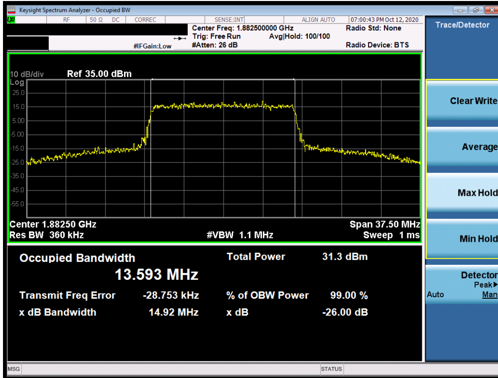
Plot 7-5. Occupied Bandwidth Plot (LTE Band 25/2 - 15MHz QPSK - Full RB Configuration)
