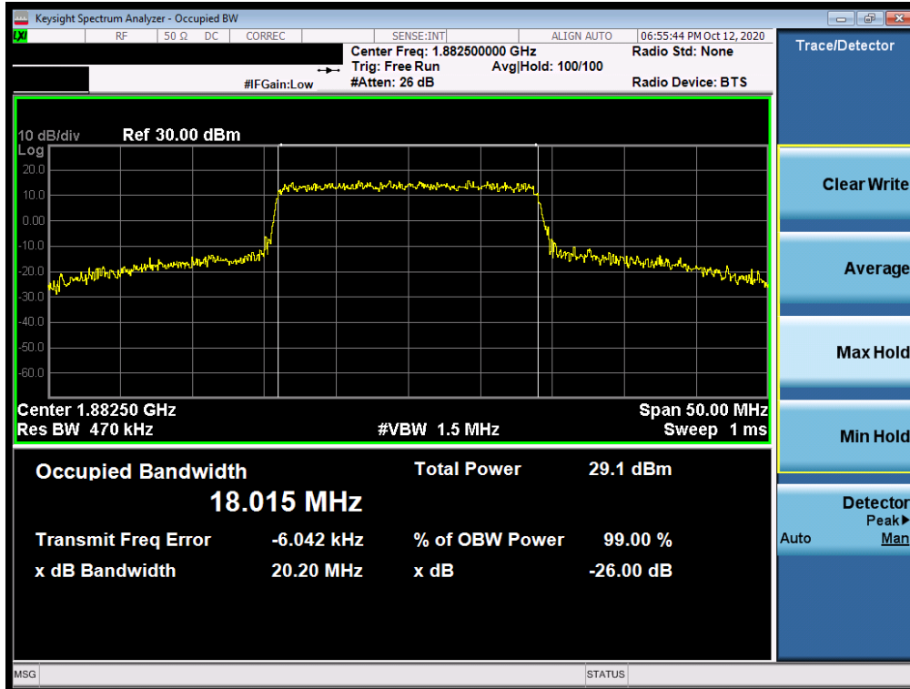
Plot 7-3. Occupied Bandwidth Plot (LTE Band 25/2 - 20MHz 64-QAM - Full RB Configuration)
