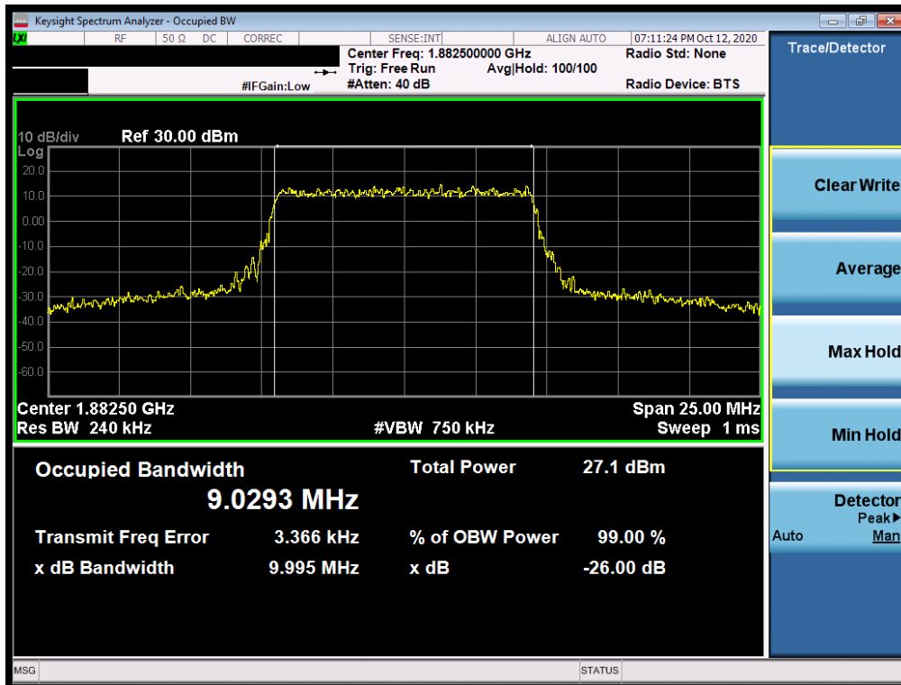
Plot 7-12. Occupied Bandwidth Plot (LTE Band 25/2 - 10MHz 256-QAM - Full RB Configuration)
