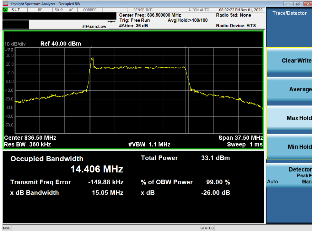
Plot 7-25. Occupied Bandwidth Plot (NR Band n5 - 15MHz QPSK - Full RB Configuration)
