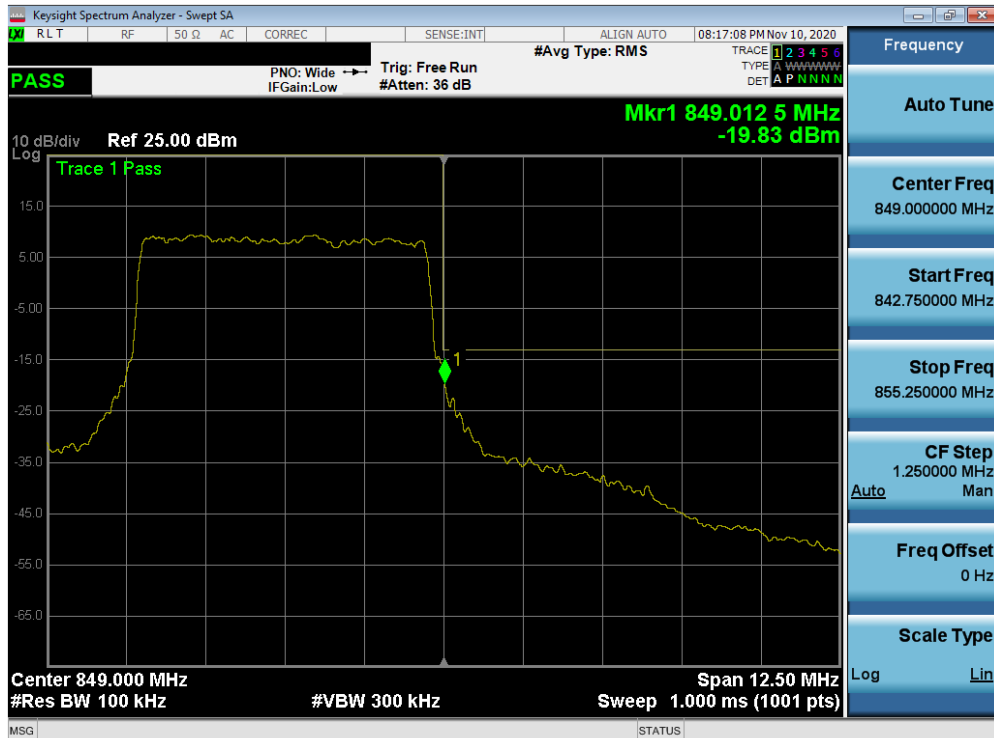
Plot 7-75. Upper Band Edge Plot (NR Band n5 – 5.0MHz – DFT-s QPSK - Full RB)
