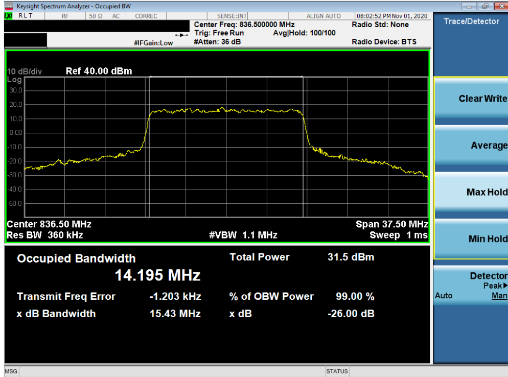
Plot 7-27. Occupied Bandwidth Plot (NR Band n5 - 15MHz 64-QAM - Full RB Configuration)
