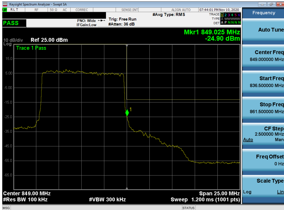
Plot 7-73. Upper Band Edge Plot (NR Band n5 – 10.0MHz – DFT-s QPSK - Full RB)
