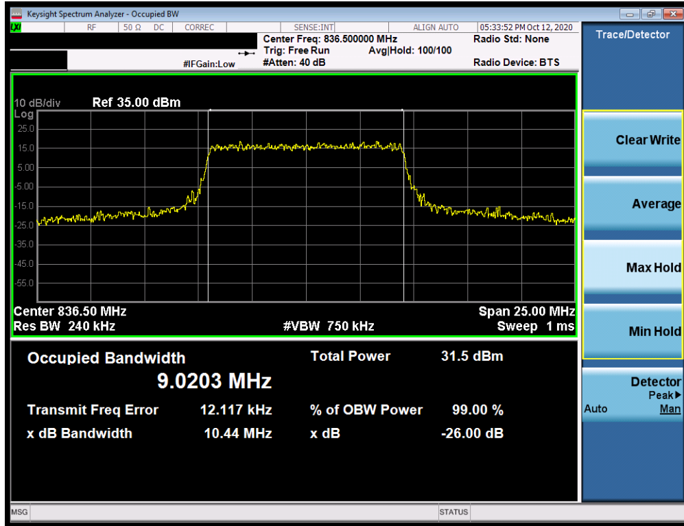
Plot 7-5. Occupied Bandwidth Plot (LTE Band 26/5 - 10MHz QPSK - Full RB Configuration)
