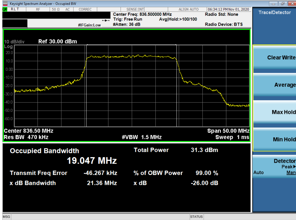
Plot 7-23. Occupied Bandwidth Plot (NR Band n5 - 20MHz 64-QAM - Full RB Configuration)
