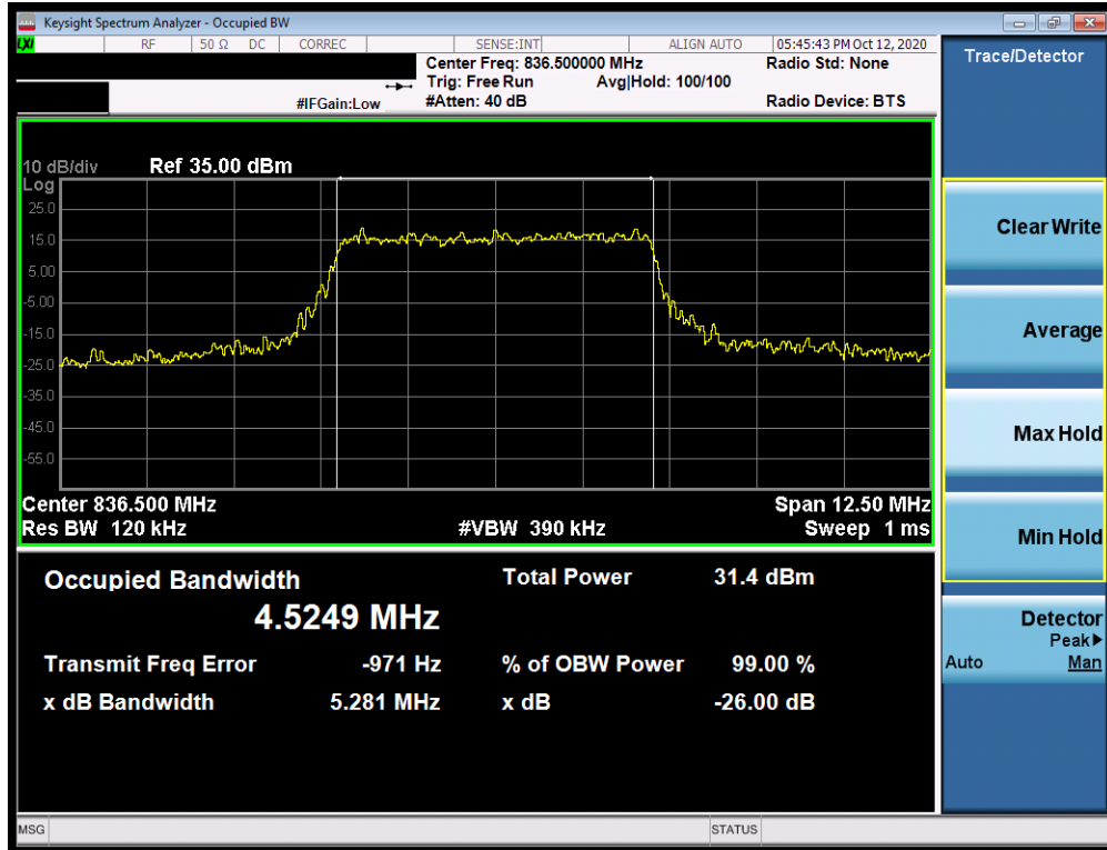
Plot 7-9. Occupied Bandwidth Plot (LTE Band 26/5 - 5MHz QPSK - Full RB Configuration)
