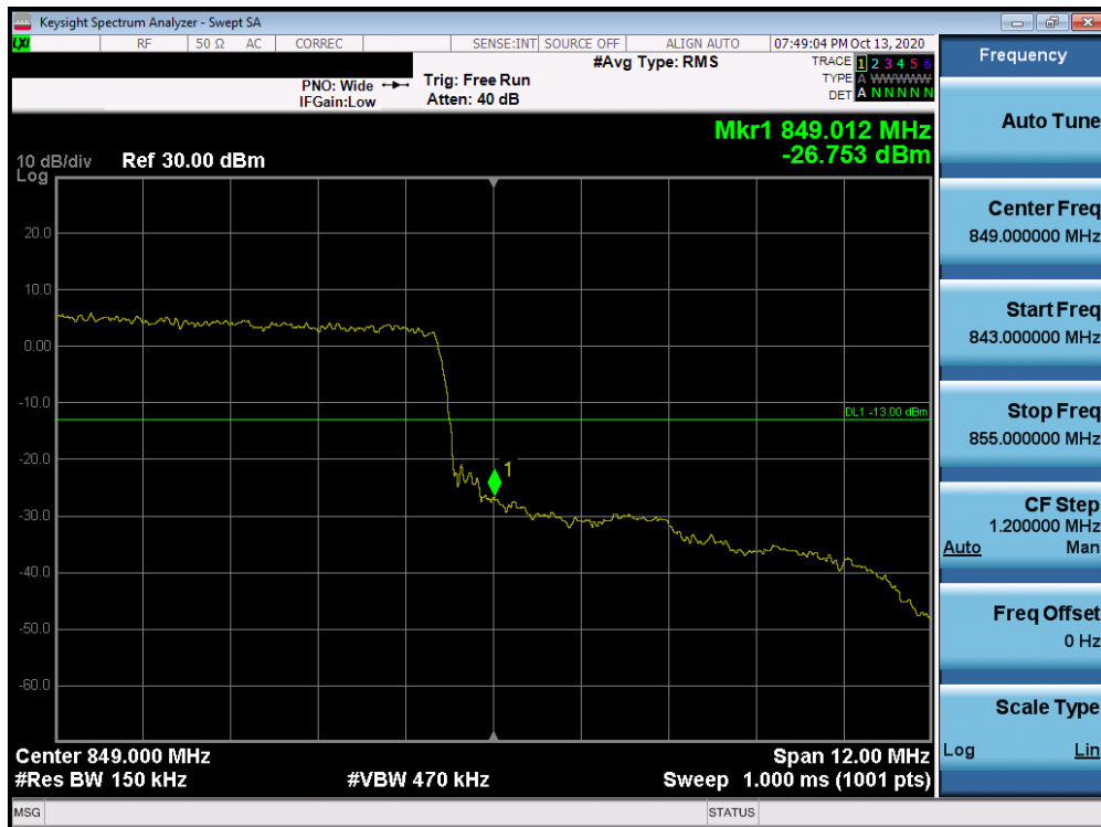
Plot 7-59. Upper Band Edge Plot (LTE Band 26 - 15MHz QPSK – Full RB Configuration)
