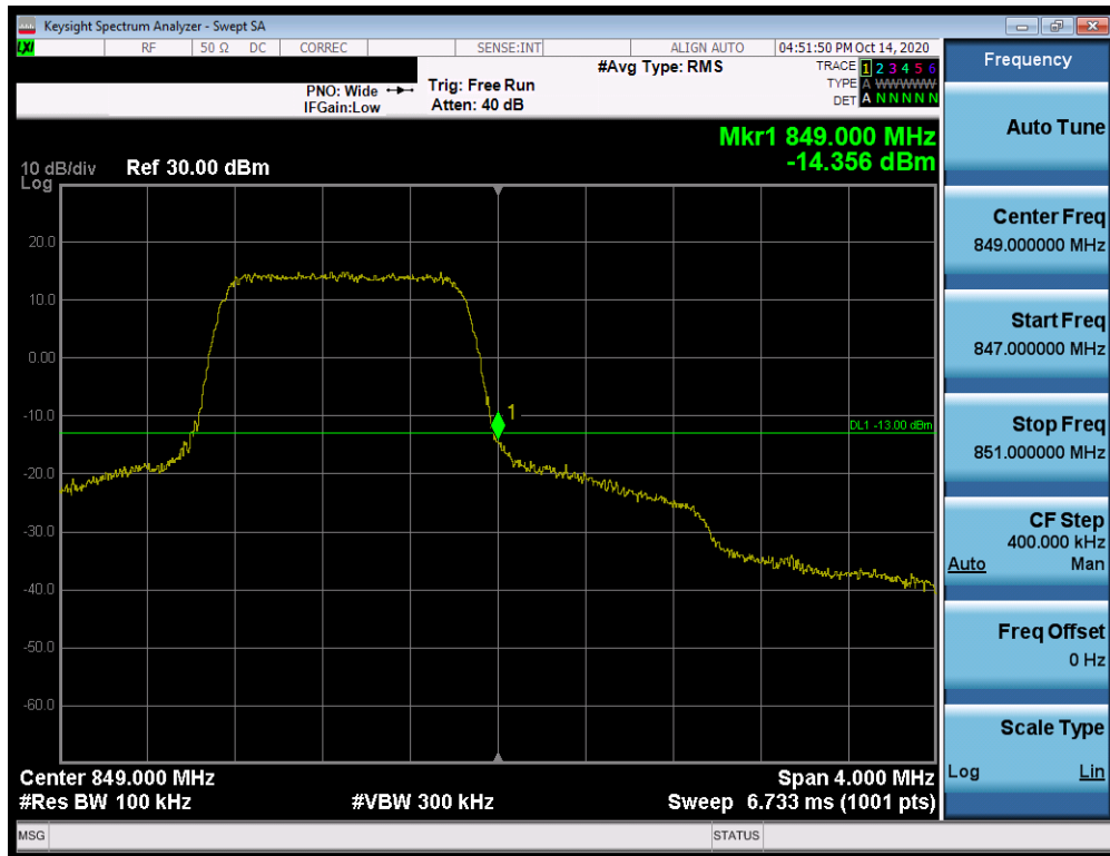
Plot 7-67. Upper Band Edge Plot (LTE Band 26/5 – 1.4MHz QPSK – Full RB Configuration)
