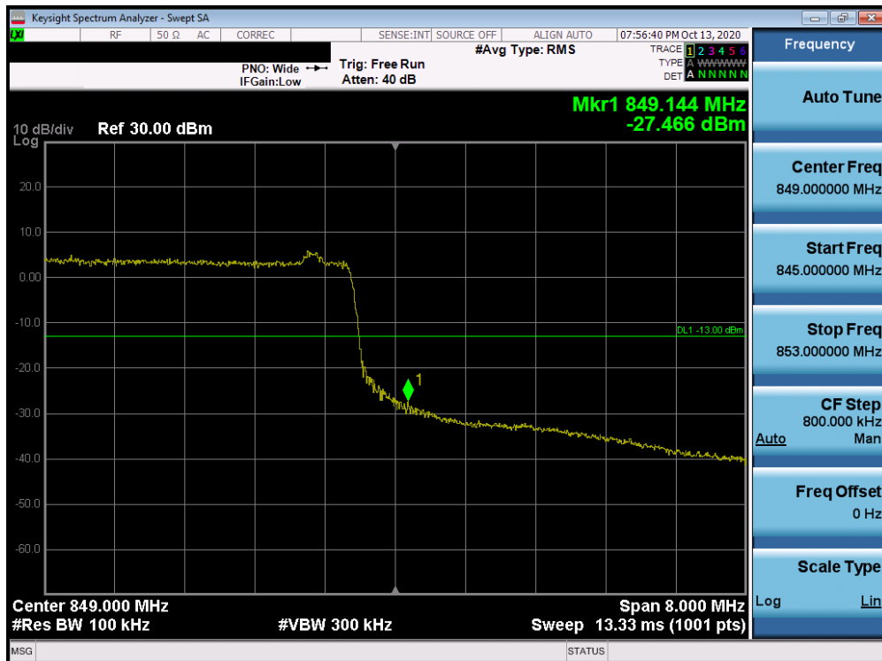
Plot 7-61. Upper Band Edge Plot (LTE Band 26/5 - 10MHz QPSK – Full RB Configuration)
