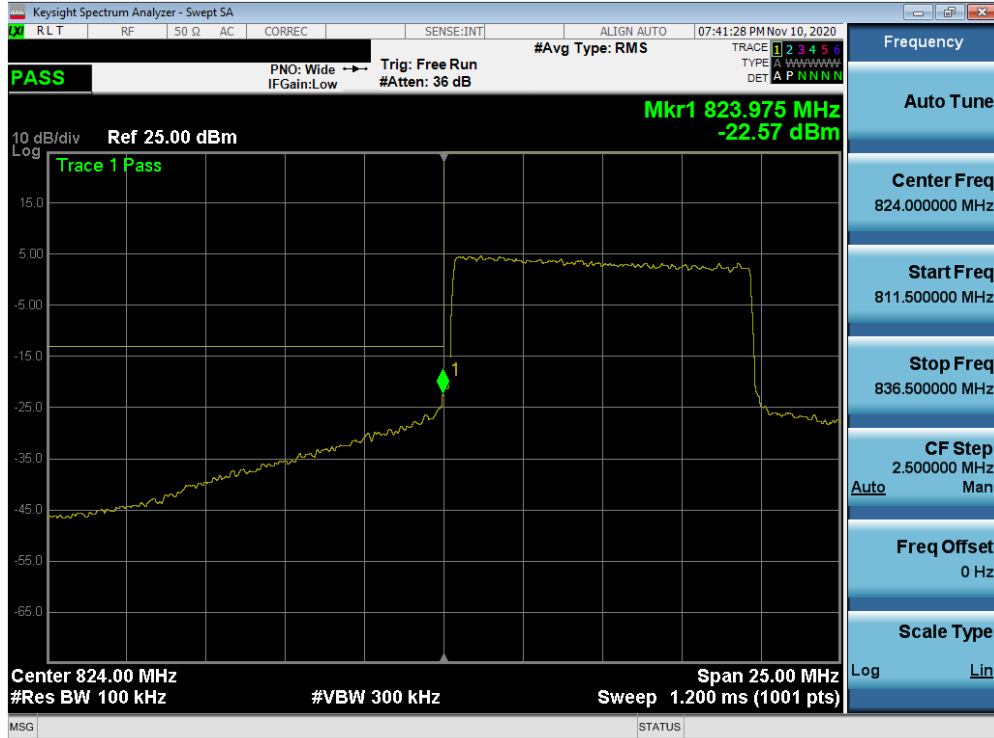
Plot 7-72. Lower Band Edge Plot (NR Band n5 – 10.0MHz - CP QPSK - Full RB)
