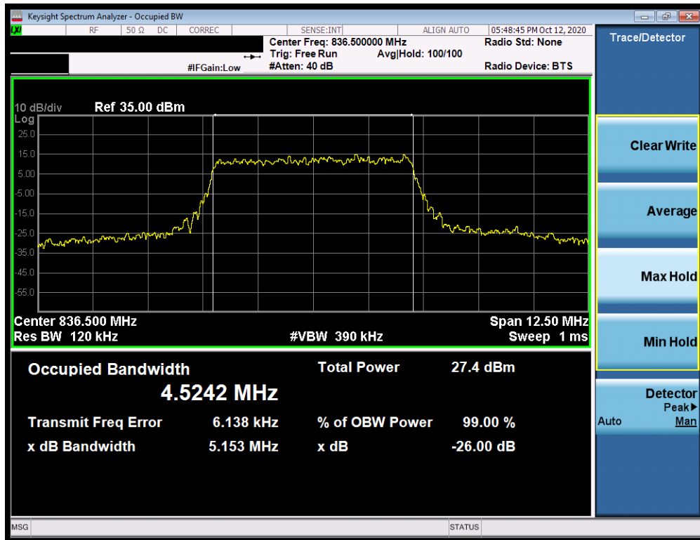
Plot 7-12. Occupied Bandwidth Plot (LTE Band 26/5 - 5MHz 256-QAM - Full RB Configuration)
