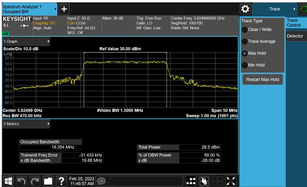
Plot 7-6. Occupied Bandwidth Plot (NR Band n48 - 20MHz 16-QAM - Full RB Configuration)
